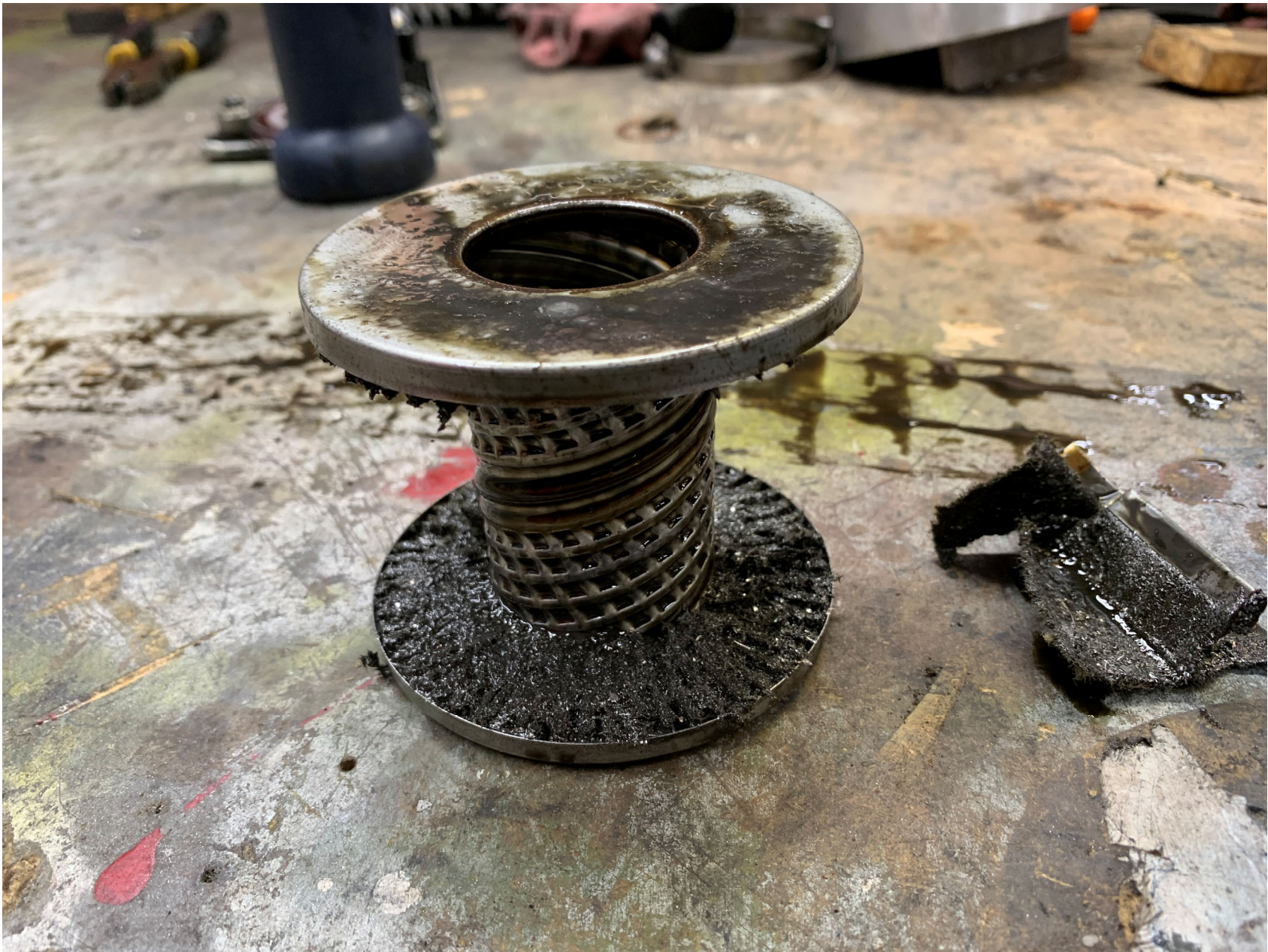
Photo 4 – Engine Oil Filter, Opened for Examination
