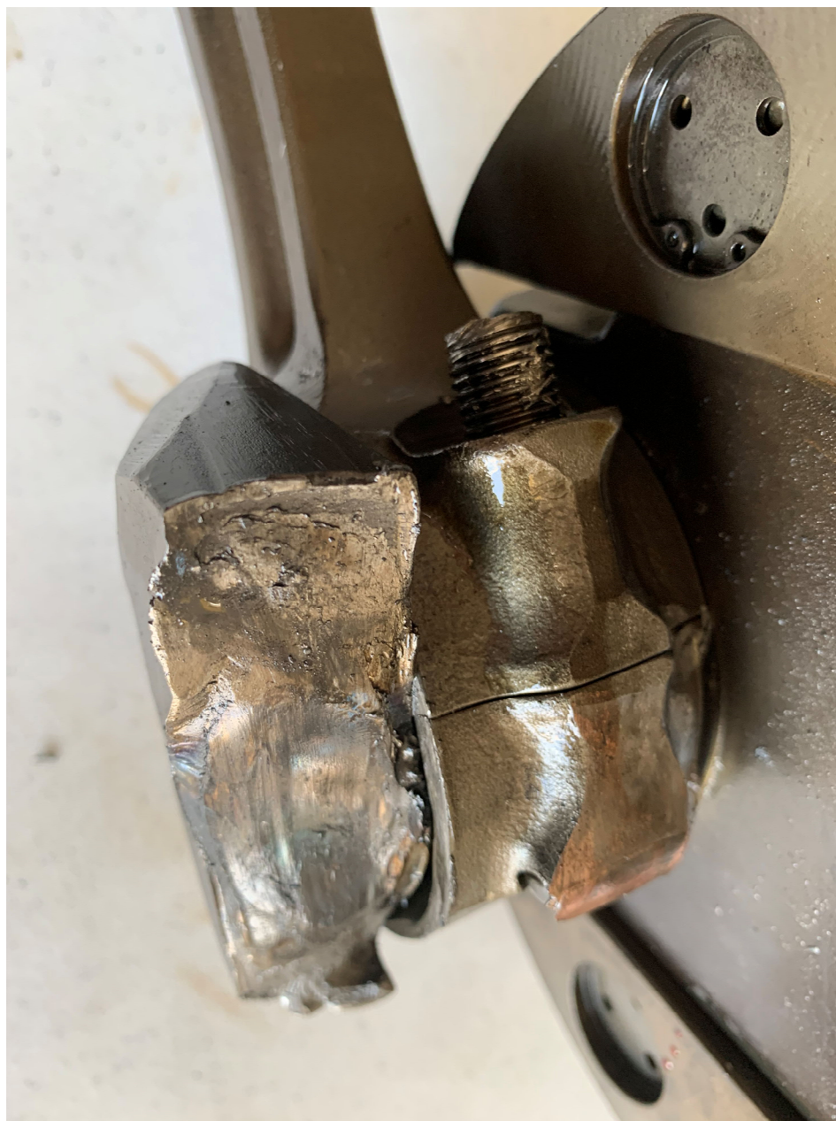
Photo 23 - #2 Connecting Rod (Foreground) with Fractured Crankshaft
