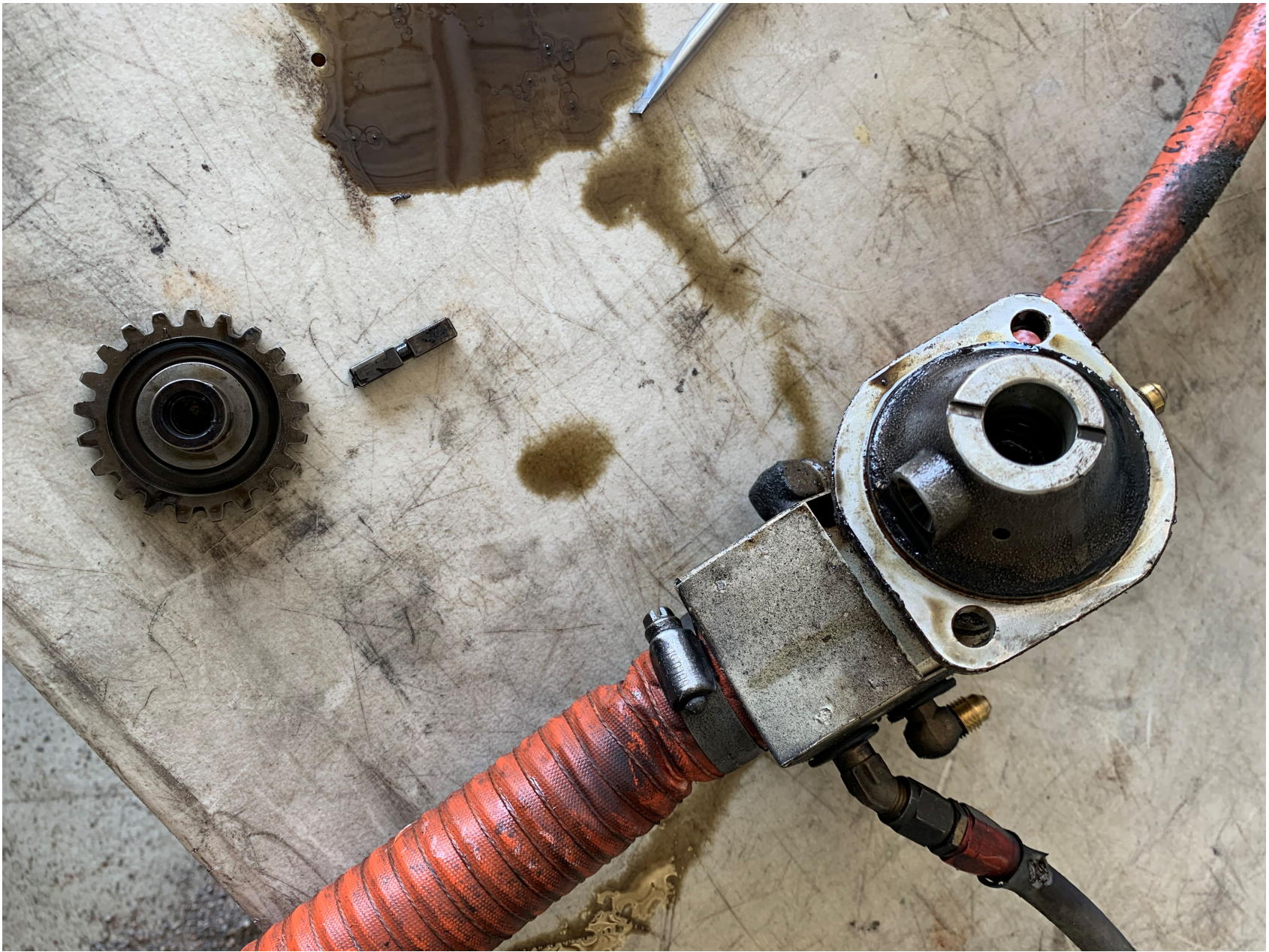
Photo 9 – Engine-driven Fuel Pump
