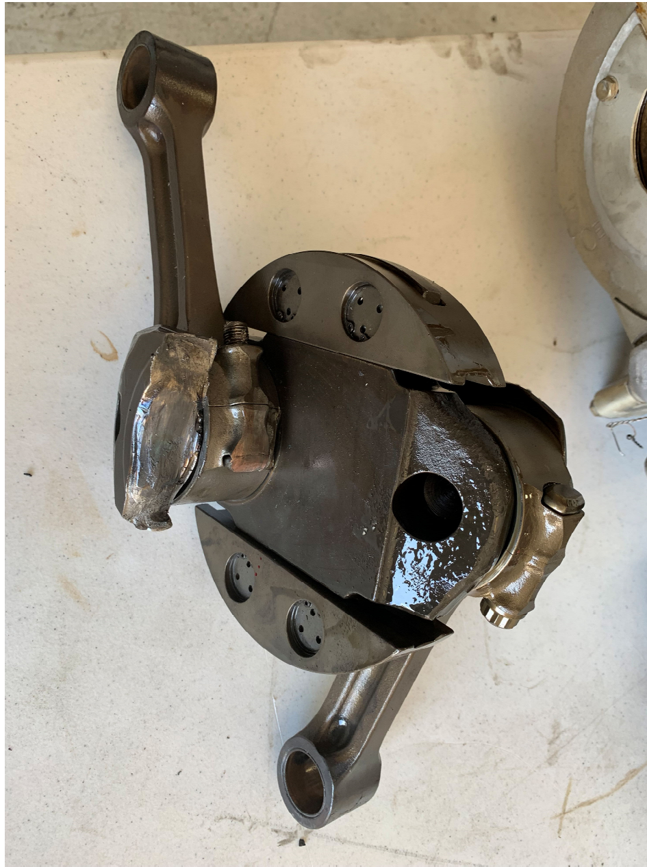
Photo 21 – #2 Connecting Rod (Foreground) with Fractured Crankshaft
