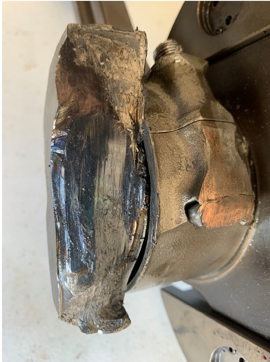
Photo 22 - #2 Connecting Rod (Foreground) with Fractured Crankshaft
