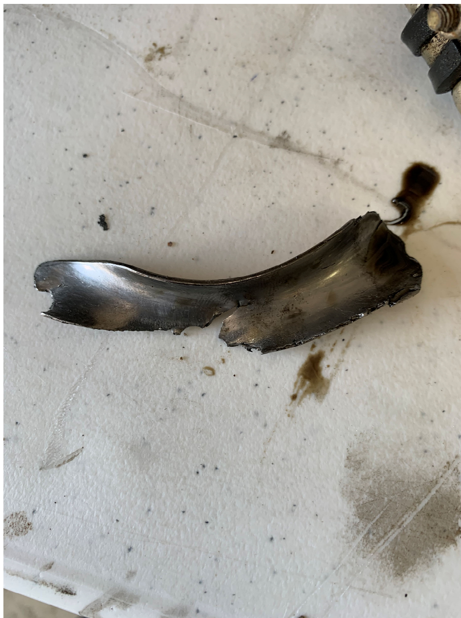
Photo 17 – Bearing Material Found Inside Engine Case
