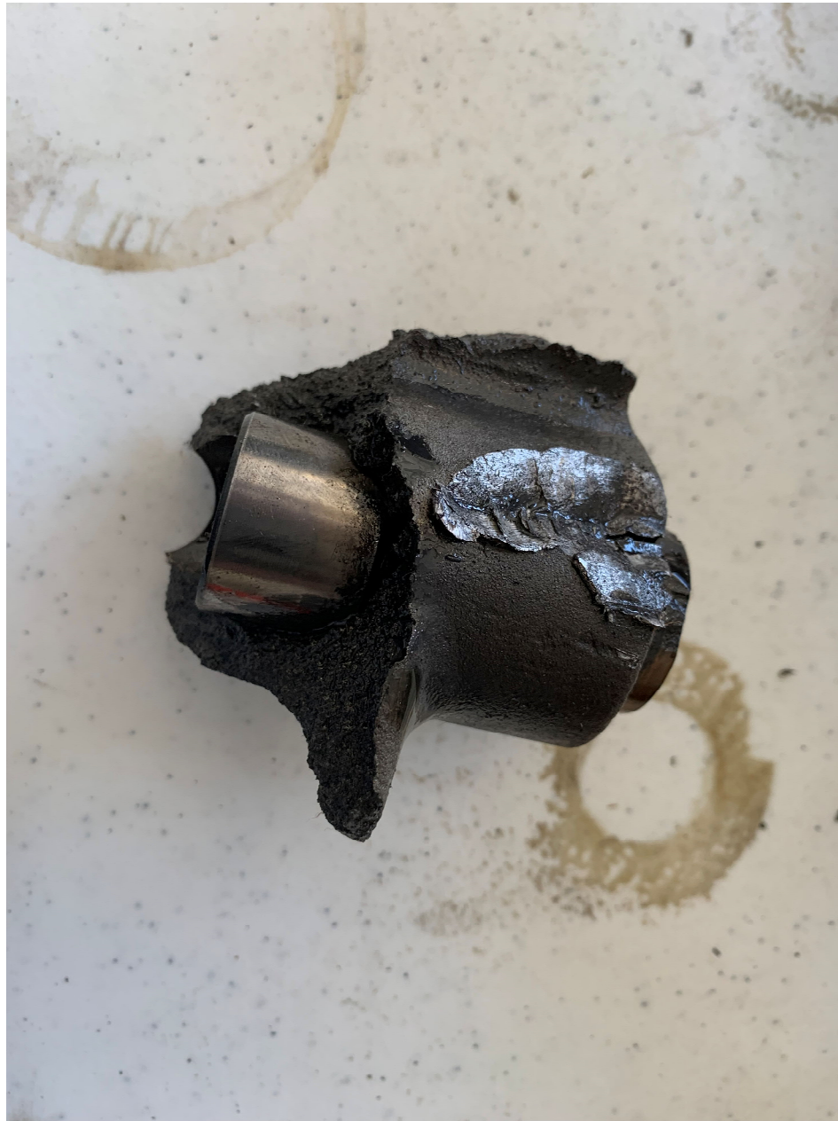
Photo 24- Separated Casting with #2 Cyl Intake Valve Tappet
