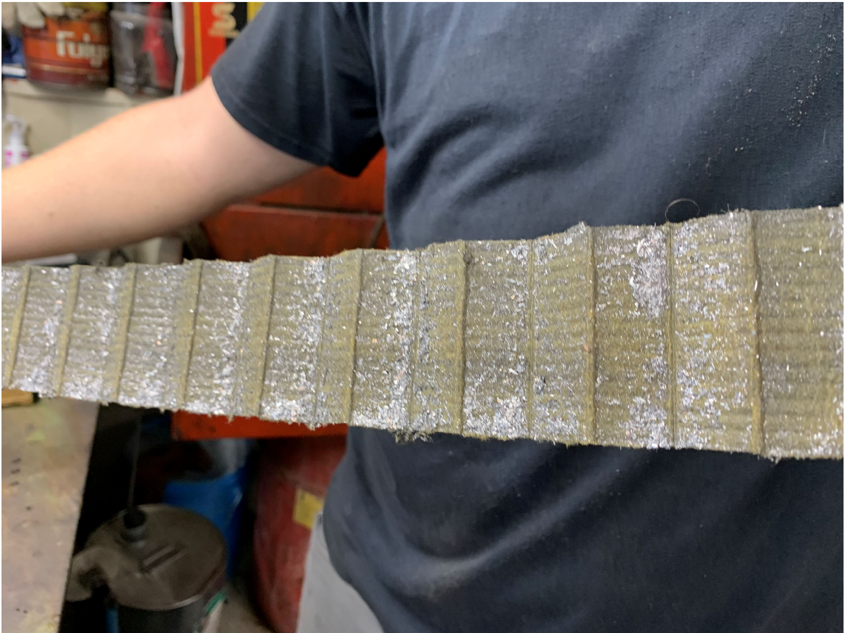
Photo 5 – Silver-colored Metallic Particulates in Oil Filter Element
