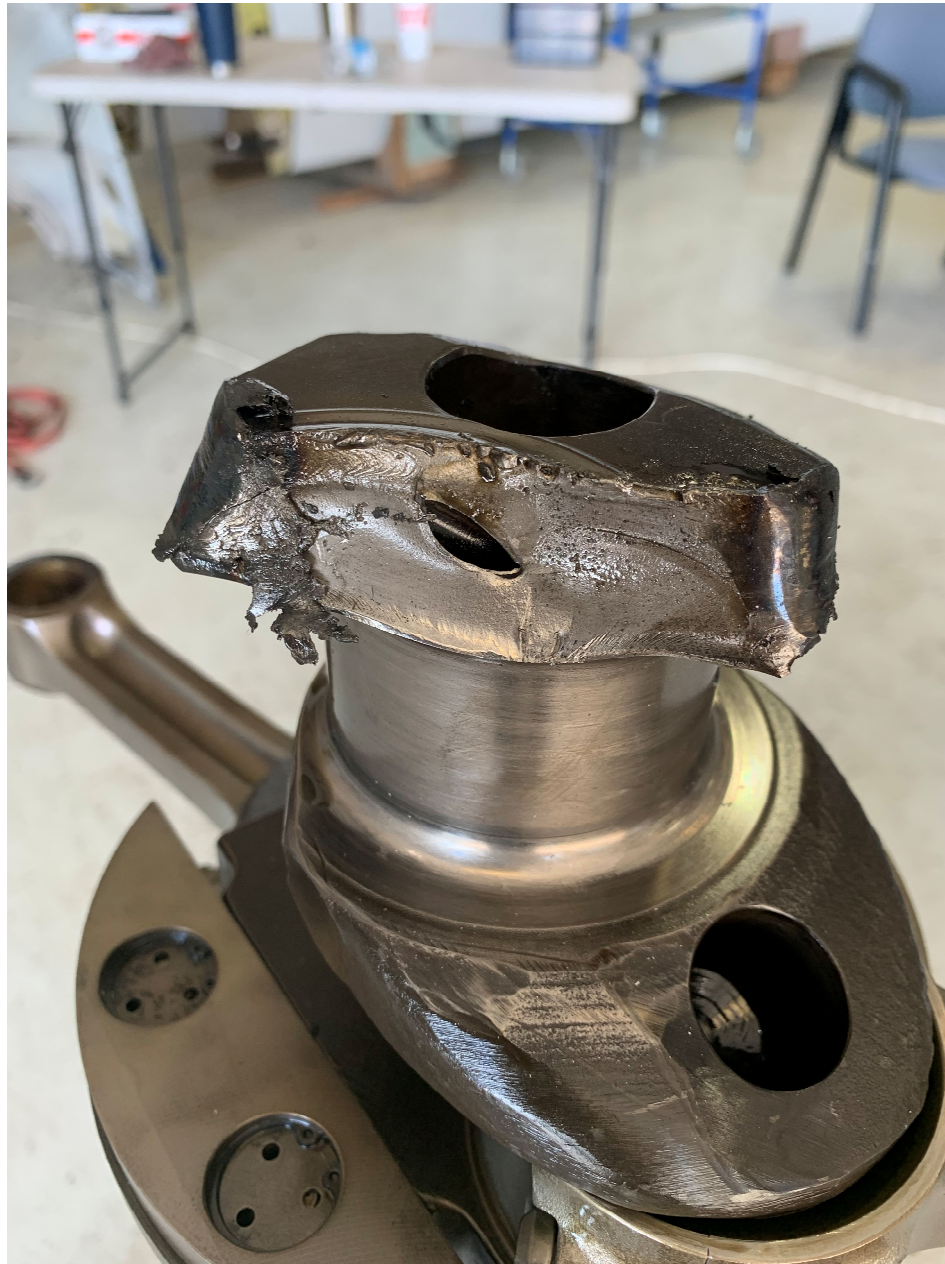
Photo 27 – Crankshaft with Fracture Surface
