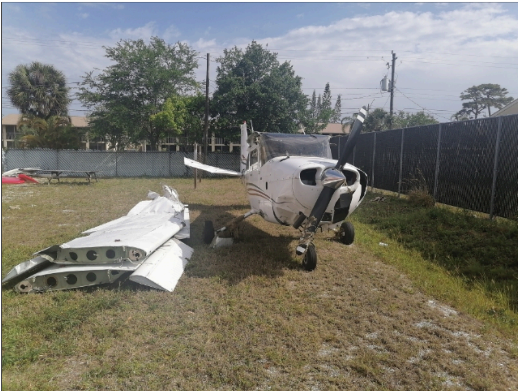
Photo 2 – View of the substantially damaged fuselage and empennage (Photo Courtesy of FAA)
