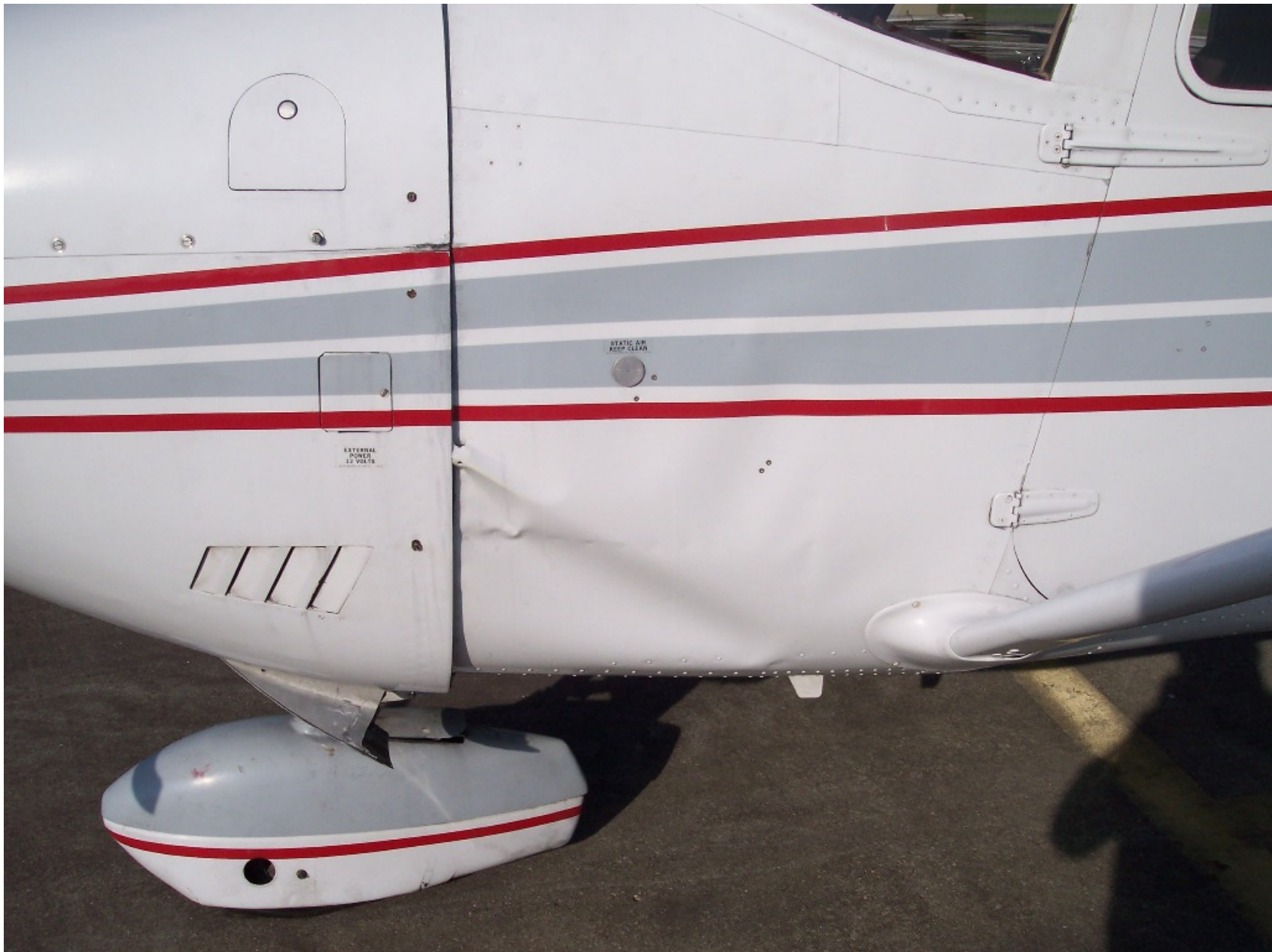
Photo 1 – FAA Digital Photograph. Left Side View of the Front Fuselage Depicting a Compression Wrinkle in the Lower Fuselage Aft of the Firewall.
