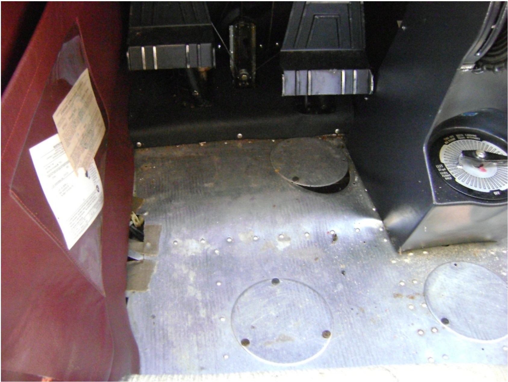
Photo 3 - FAA Digital Photograph. View Depicting Buckling of the Pilot's Floor.
