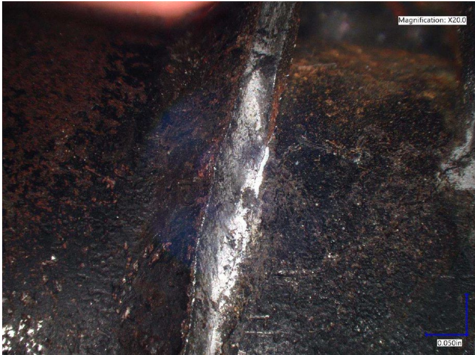
Photo 19 – Left Hand Side of Fracture Surface Magnified to 20x Showing Fresh Substrate – Courtesy of Piper Aircraft
