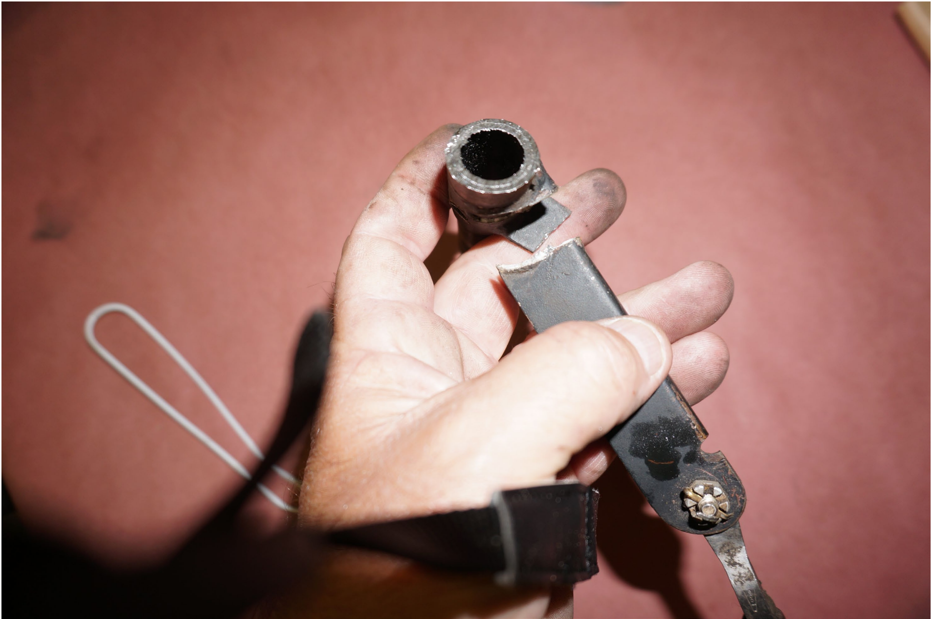
Photo 12 –Rudder Control Assembly Tube and Rudder Control Arm
