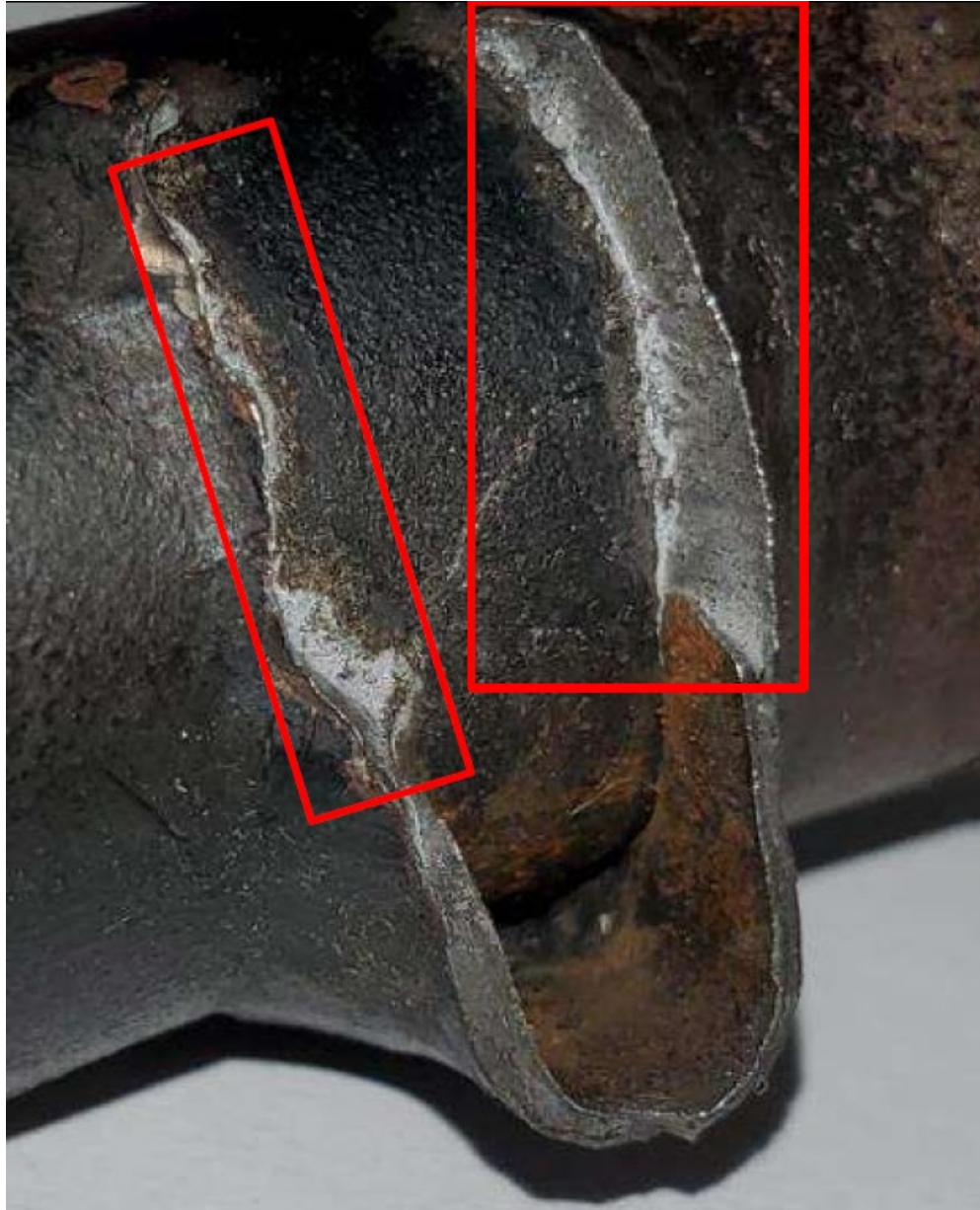
Photo 14 – Fracture Surface Near Weld – Courtesy of Piper Aircraft
