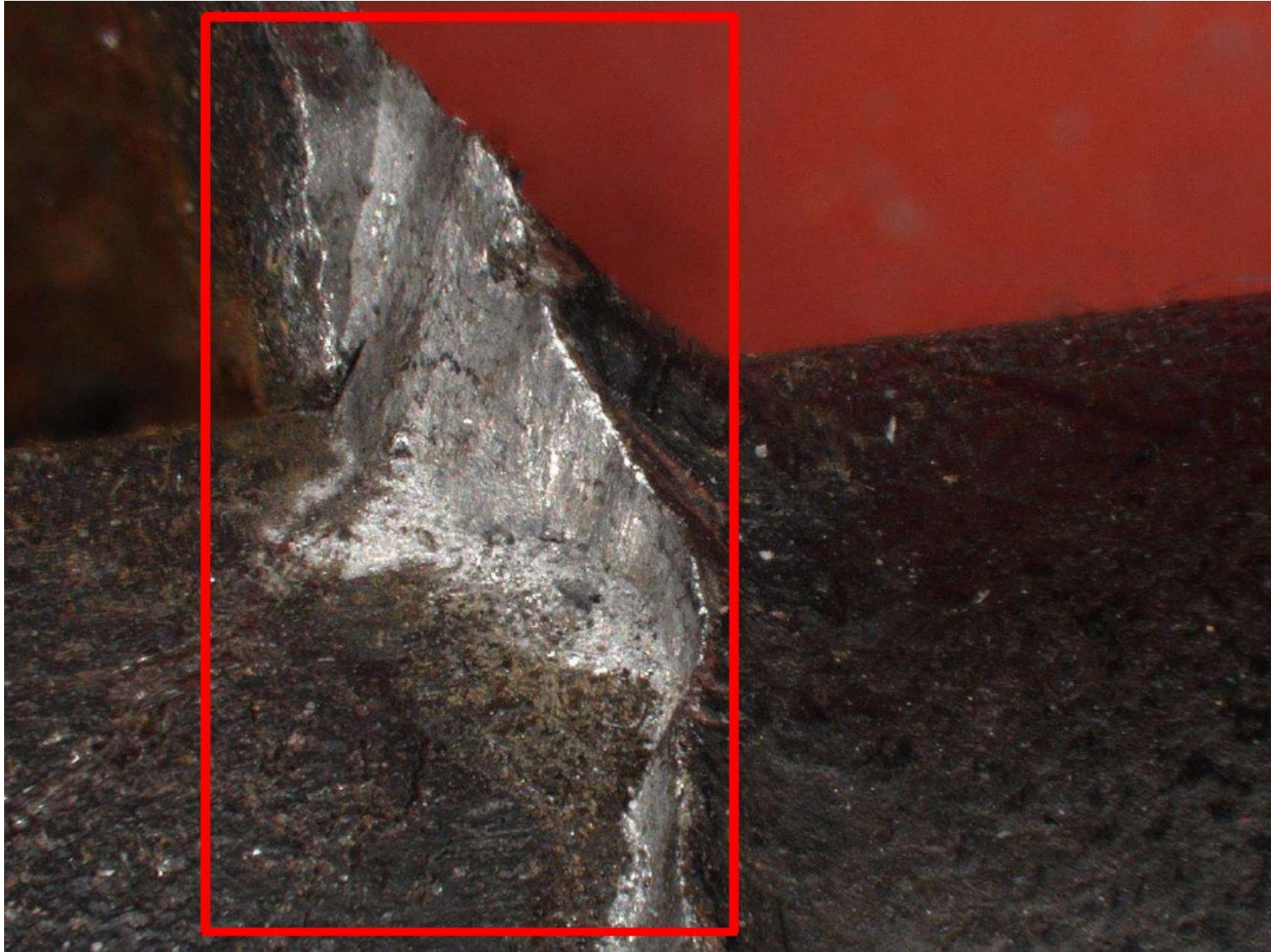
Photo 17 – Right Hand Fracture Surface with Porosity – Courtesy of Piper Aircraft
