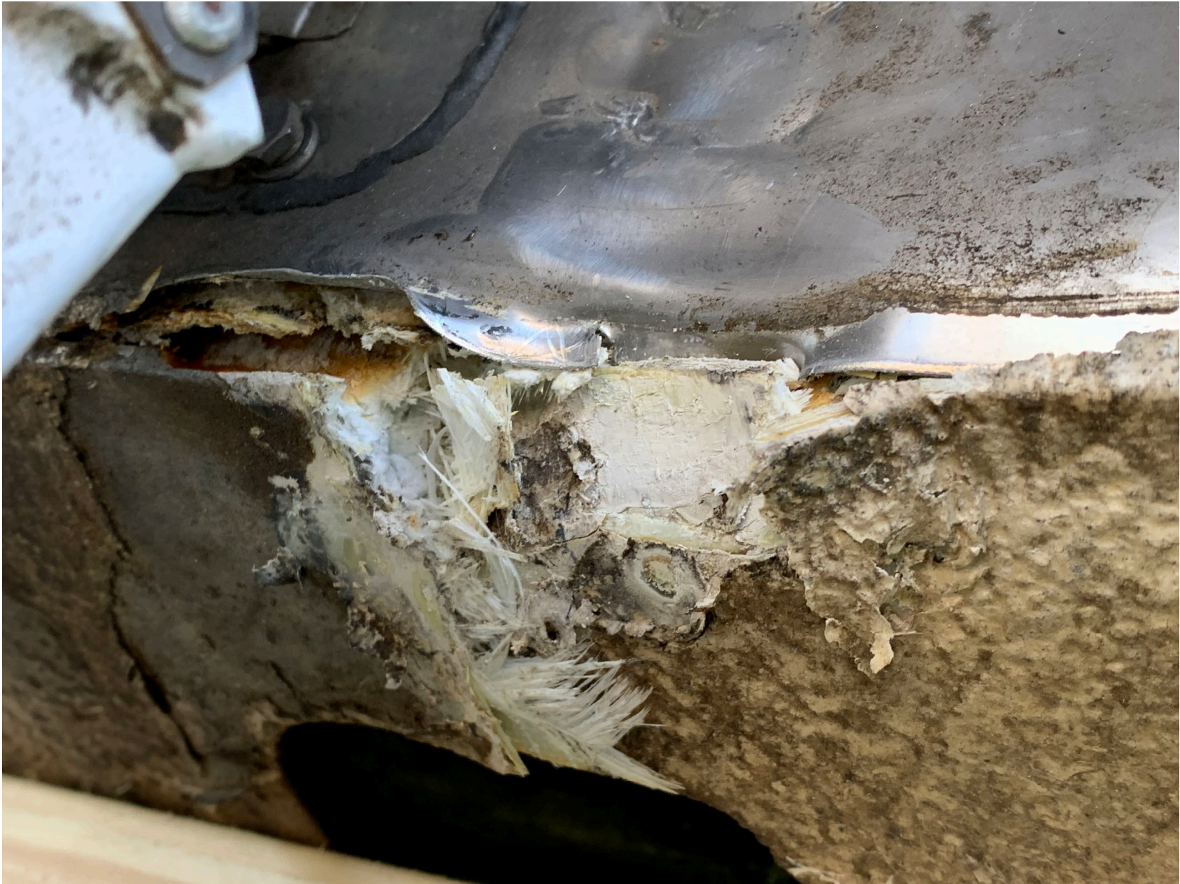
Photo 1 – View of damaged fuselage structure and firewall (FAA Photo)
