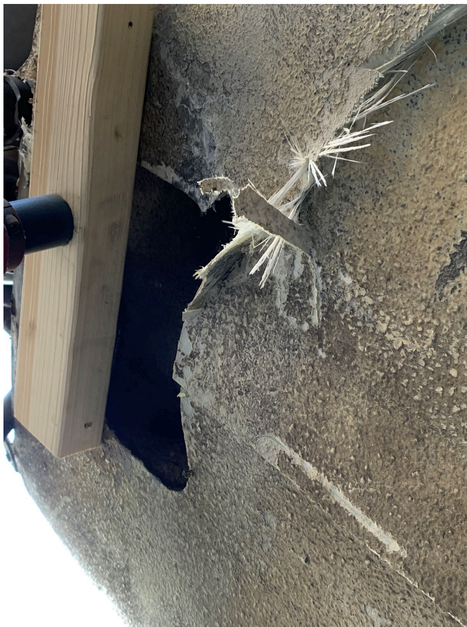
Photo 2 – View of underside of fuselage showing structural damage, (FAA Photo)
