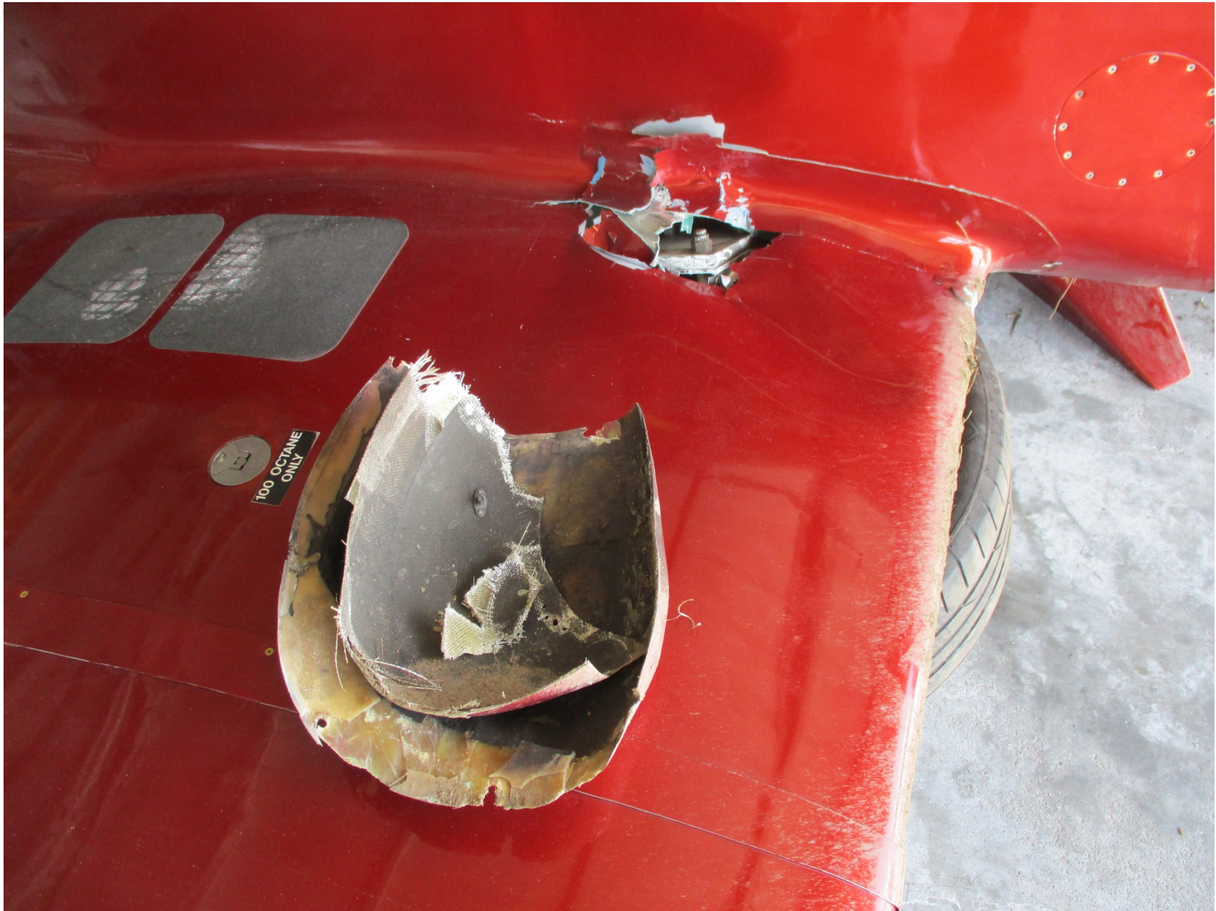
Photo 2 – right wing with gear protruding through (FAA)
