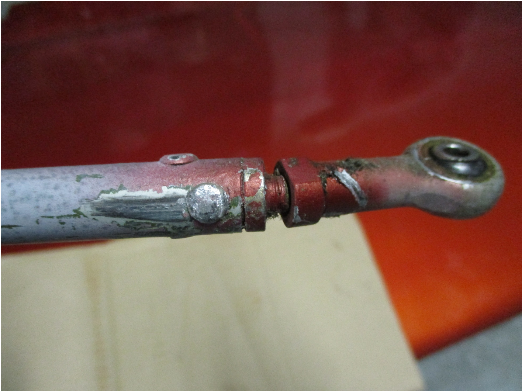
Photo 3 – Left Push/pull rod with rivet that was binding (FAA)
