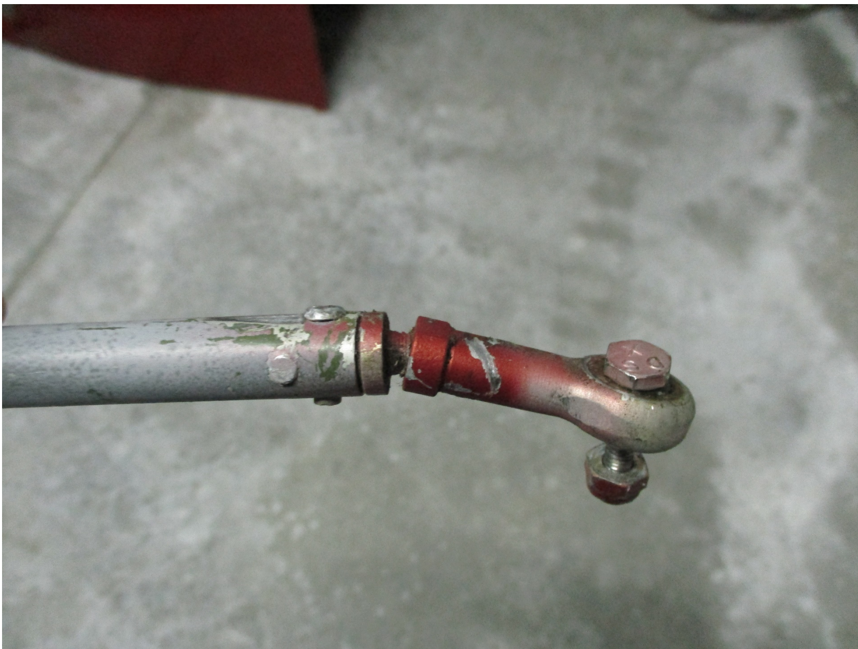
Photo 4 – left push /pull rod bent (FAA)
