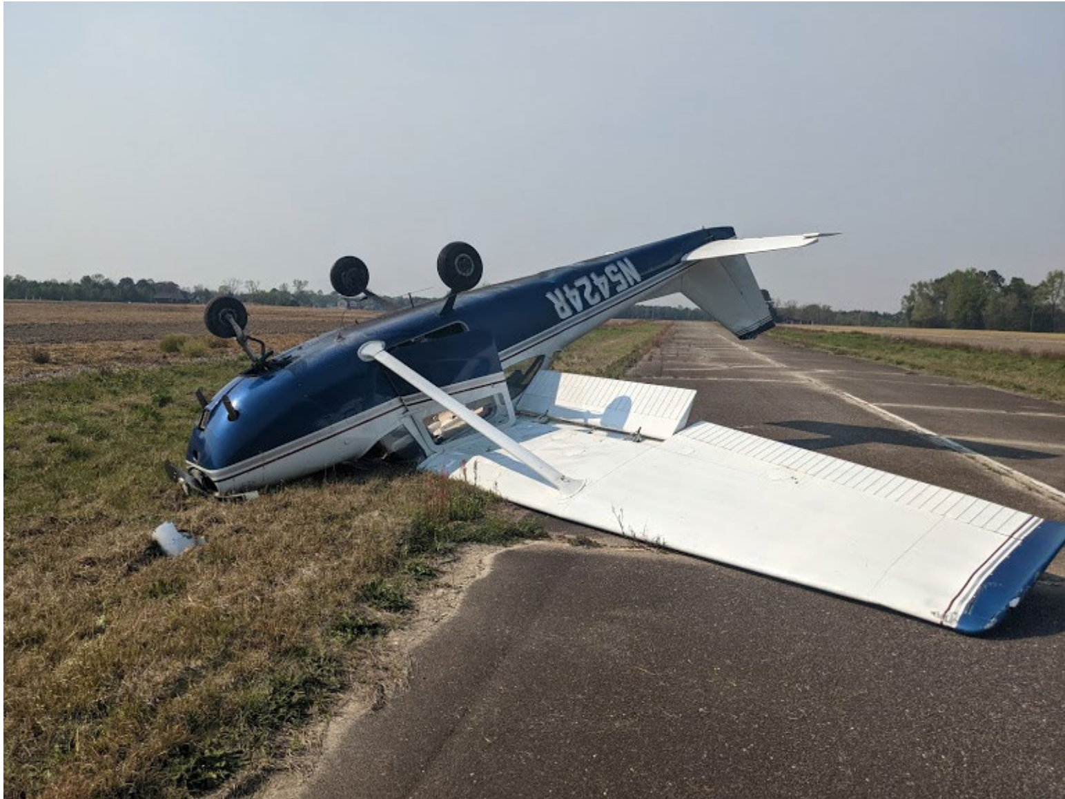
Photo 1 – View of right side of airplane as it rests inverted off runway. Note damage to right wing. (Courtesy of FAA)
