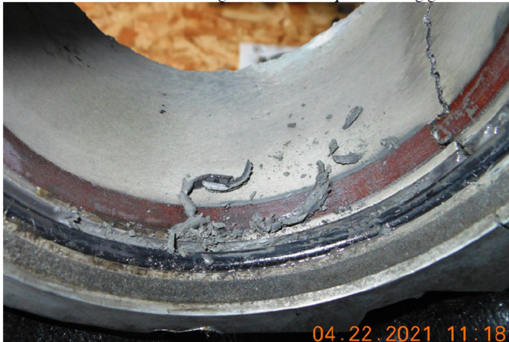
Photo # 11- Hardened sludge removed from piston O-ring groove
