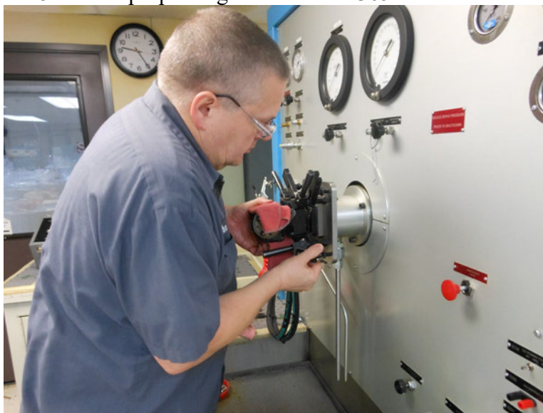
Photo # 18-1 –Left propeller governor S/N 4365F mounted to test stand
