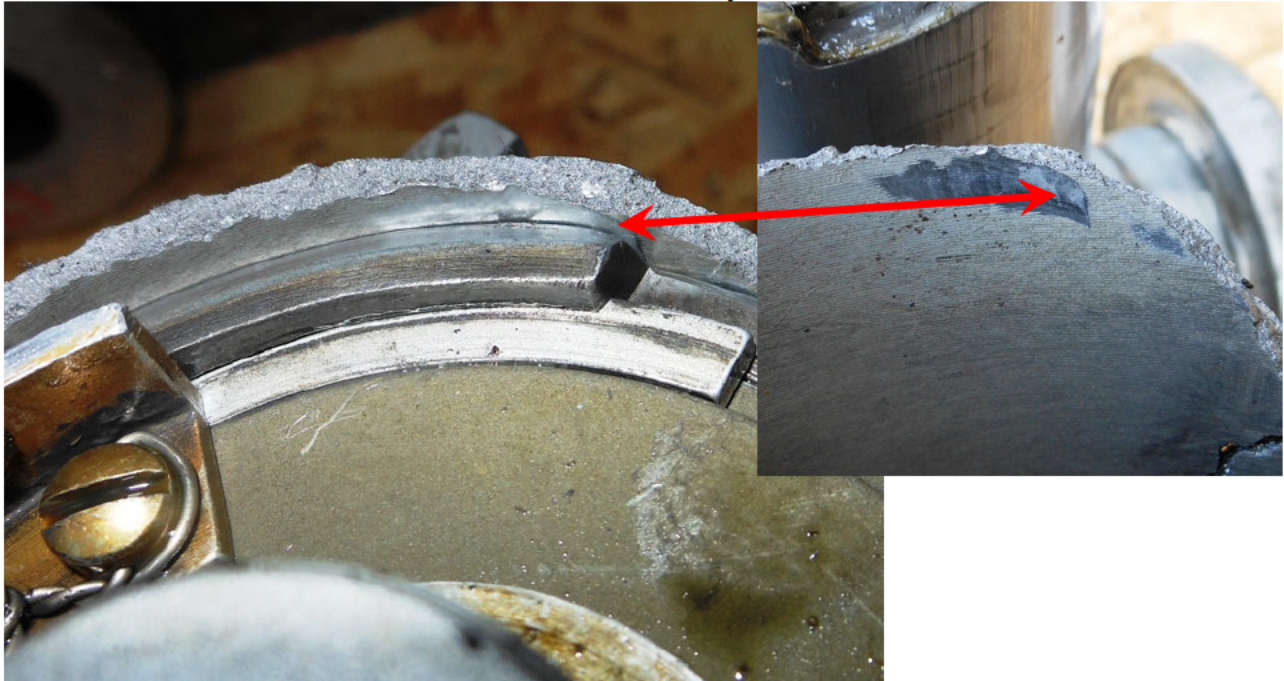
Photo #9 – Piston contact mark with cylinder forward corner
