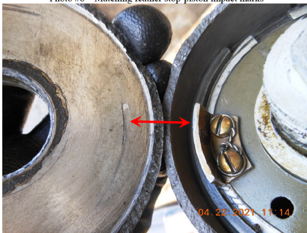
Photo #8 – Matching feather stop-piston impact marks
