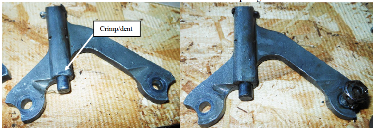
Photo # 12- Start lock brackets and plungers
