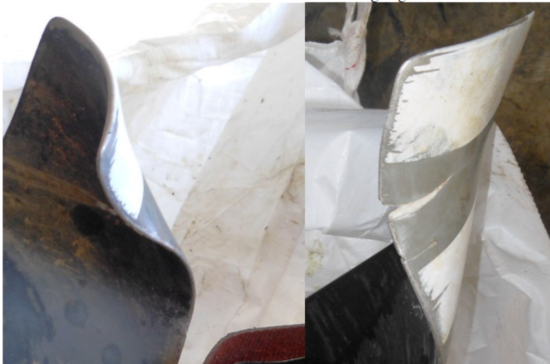
Photo # 21 – Wave bends in leading edge
