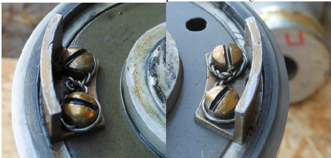
Photo #7 – Feather stops with contact damage
