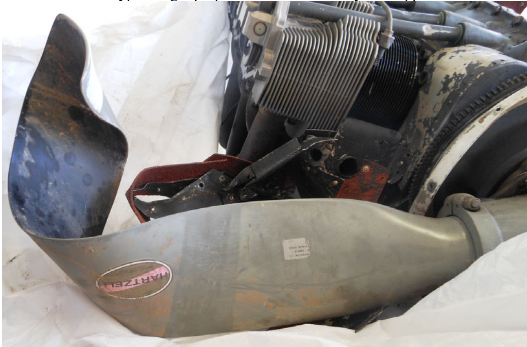
Photo #20 – Typical right propeller blade remarkably bent opposite rotation
