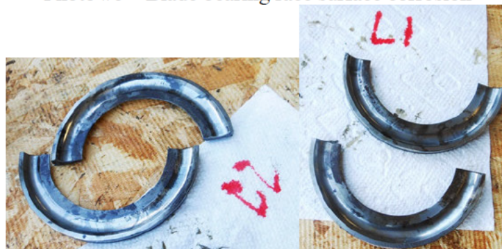
Photo #6 – Blade bearing race surface corrosion
