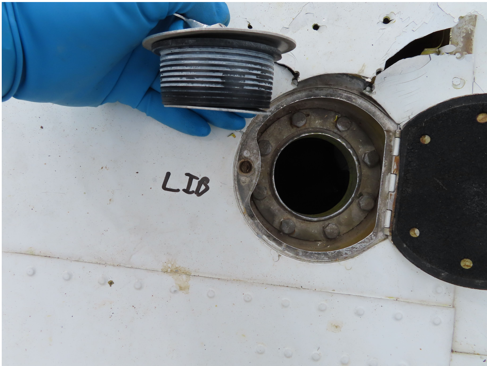
Photo 9 – View of Duct Tape and Adhesive Residue on Left Inboard Fuel Tank Cap (Piper)
