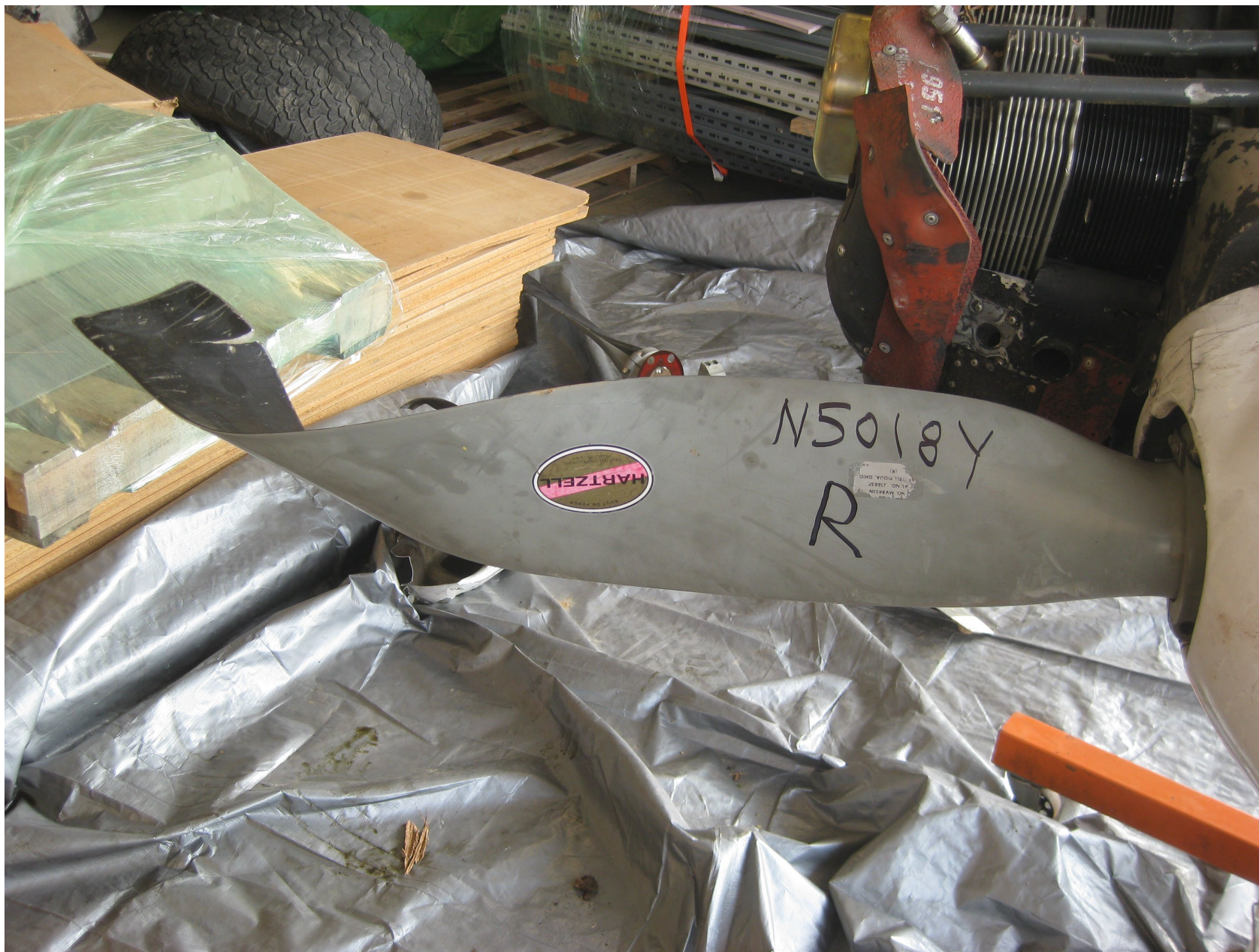
Photo 5 – View of Right Propeller Blade, Tip Curl, and Tear (Lycoming)
