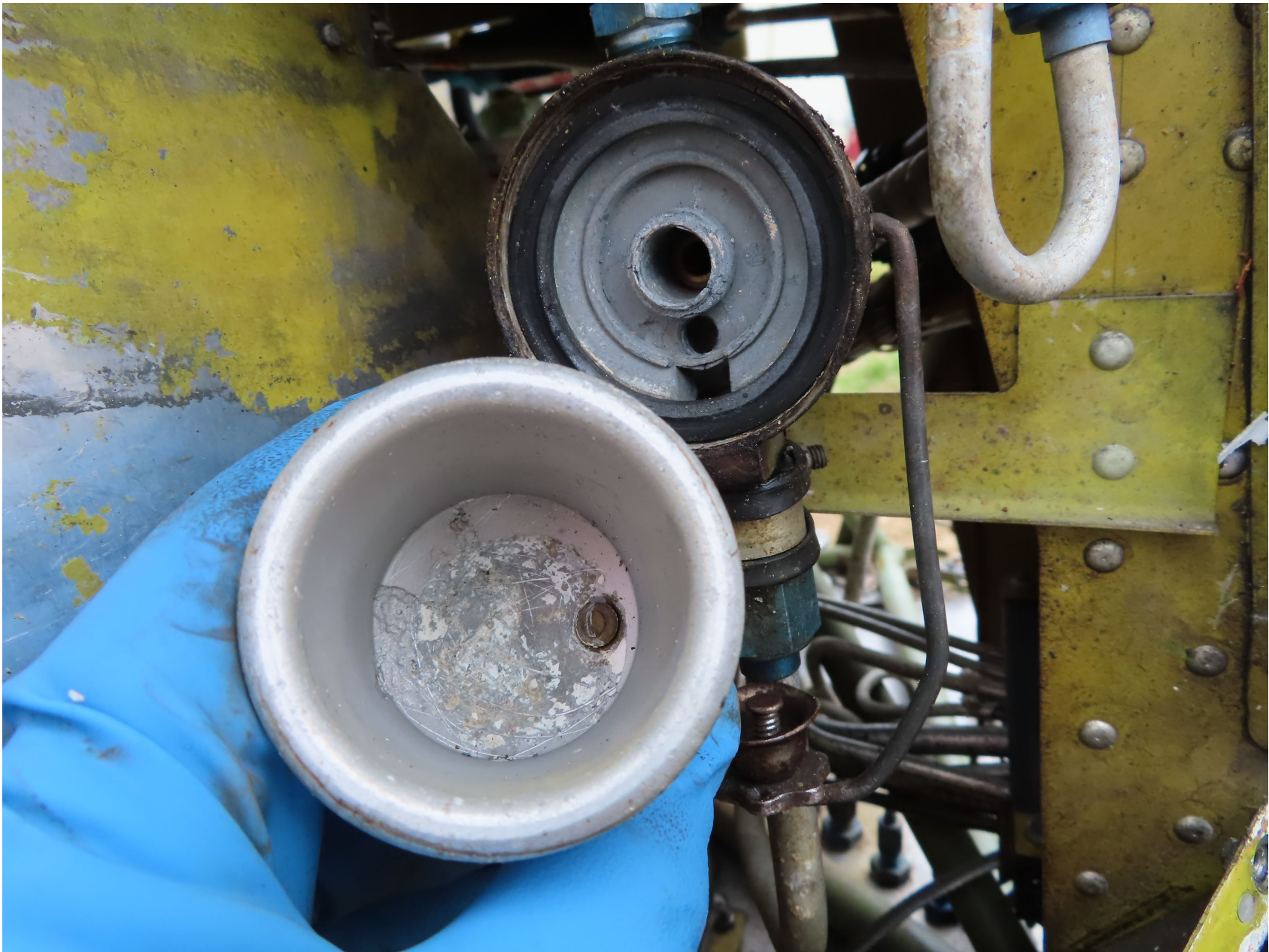
Photo 6 – Left Wing Gascolator as Found (Piper)
