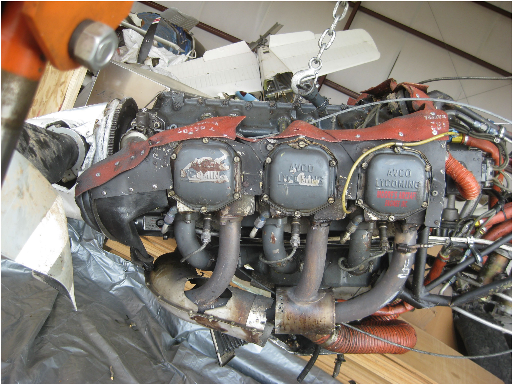
Photo 4 – View of Right Engine and Curled Propeller Tip (Lycoming)
