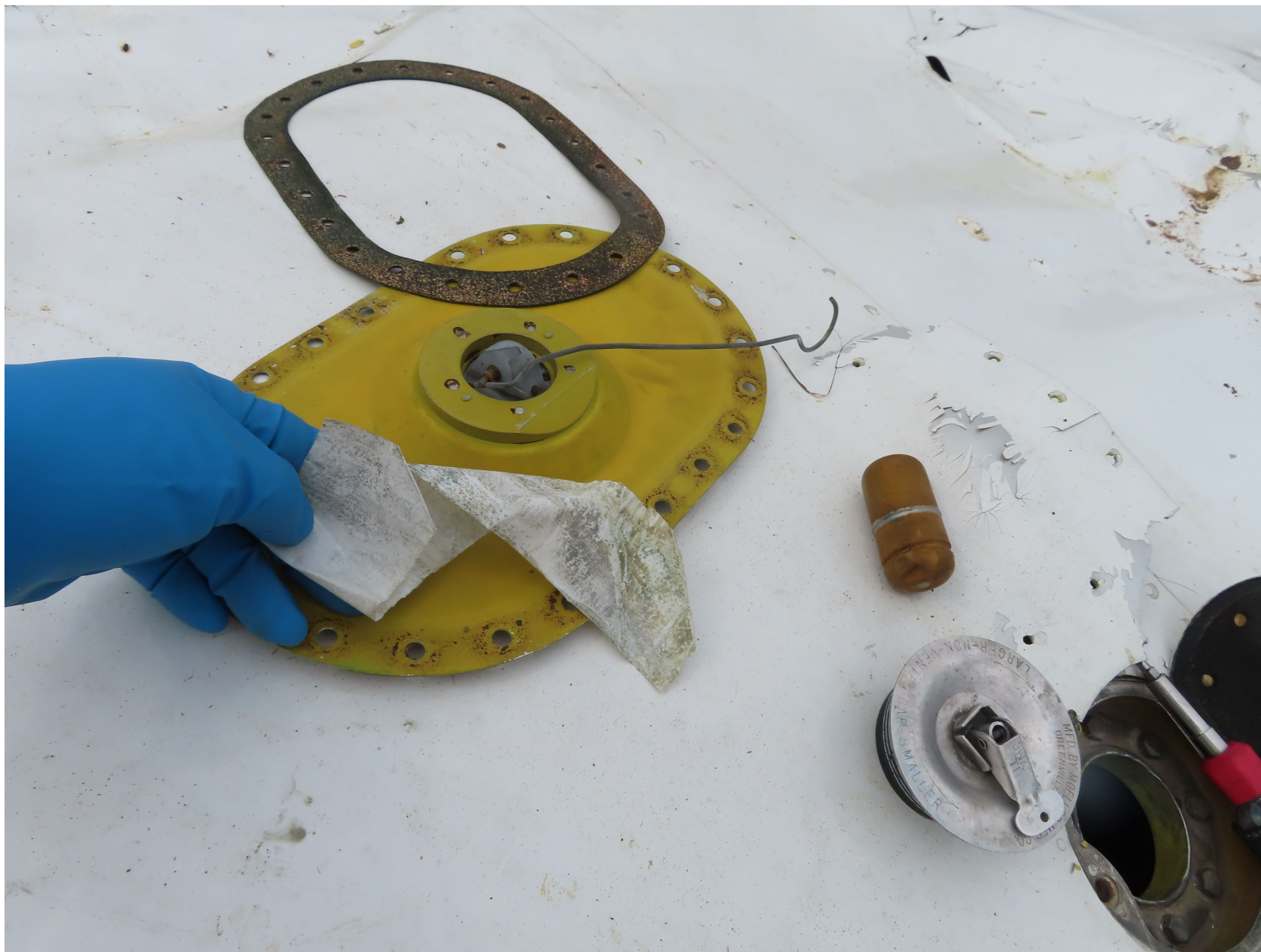
Photo 8 – View of Duct Tape Strip Found Loose Inside Left Wing Inboard Fuel Cell (Piper)
