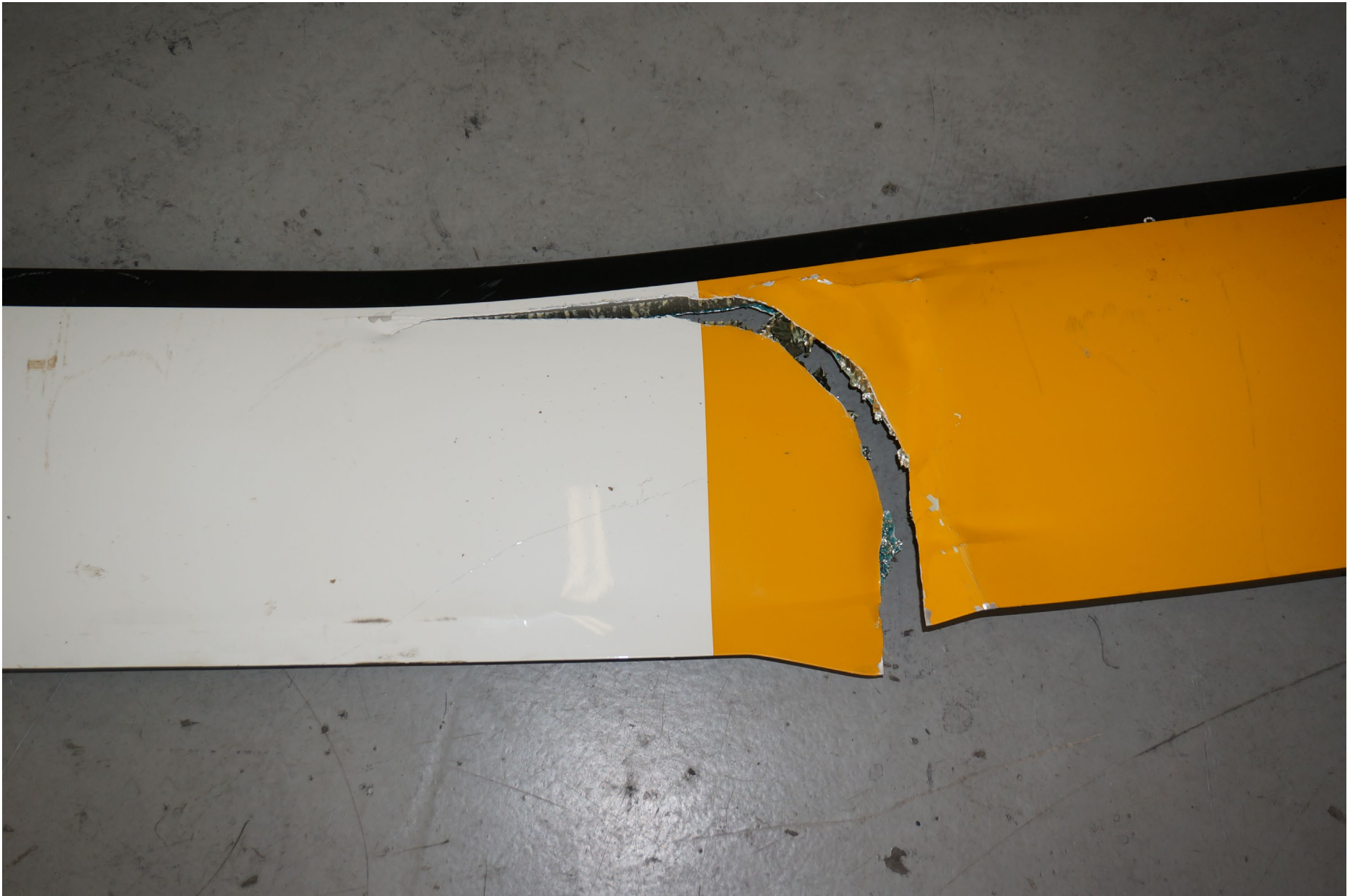
Photo 12 – Close Up of Break in Main Rotor Blade No. 2
