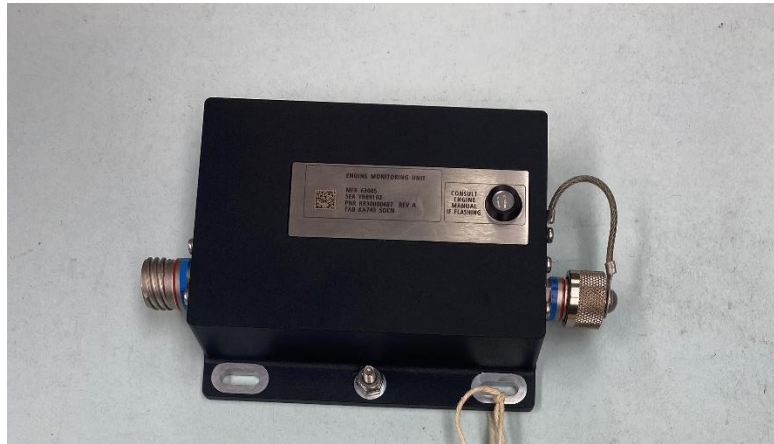
Figure 1. The Rolls-Royce EMU-300 from the accident aircraft.
