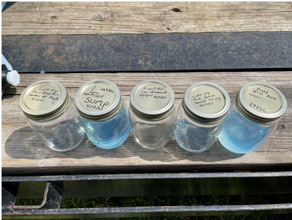
Figure 2: Top View of Sample Jars in Same Orientation as Figure 1 Depicting Labeling of Jars. 3 rd Jar from the Left is the Fluid Drained From the Flexible Hose From the Firewall Fitting to the Inlet of the Engine-Driven Fuel Pump.
