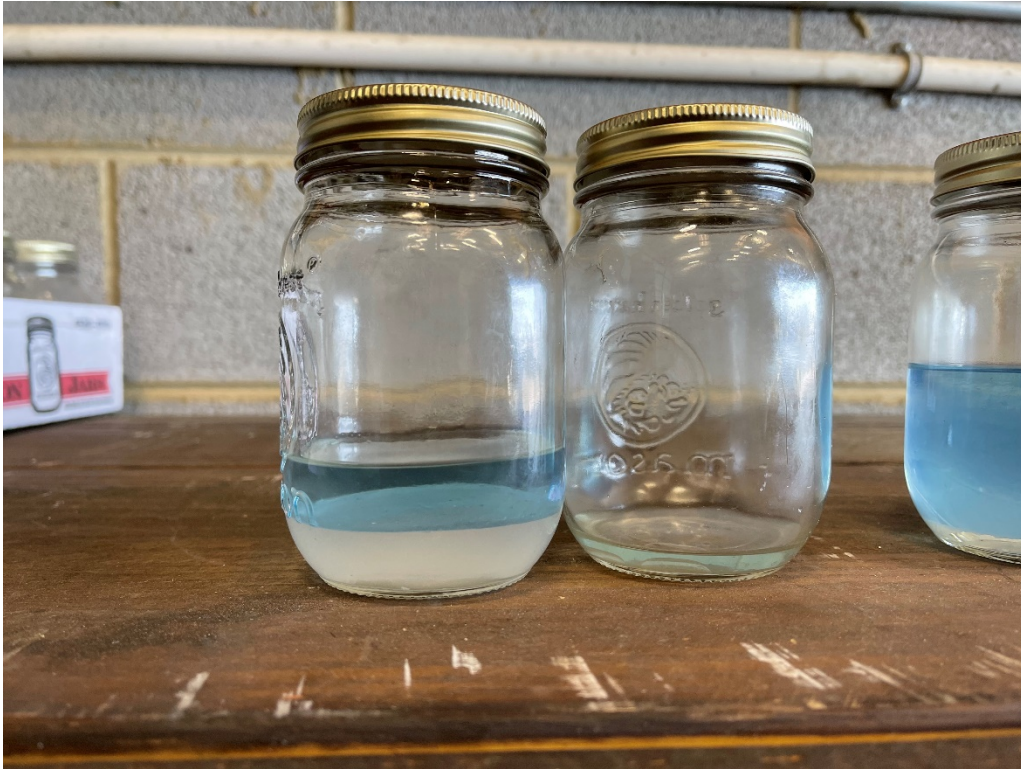
Figure 3: Jar on Left Depicts the Fluids Drained From the Carburetor Bowl. Note The Total Drained Amount was About 5 Ounces and was About Equal Parts Fuel and Water.
