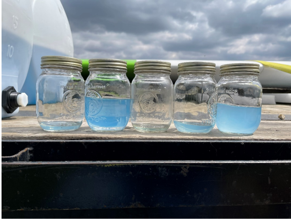
Figure 1: Photograph Taken by Dave Stanton. View of the Fuel Samples Taken During Recovery of the Airplane. 3 rd Jar from the Left is the Fluid Drained From the Flexible Hose From the Firewall Fitting to the Inlet of the Engine-Driven Fuel Pump.
