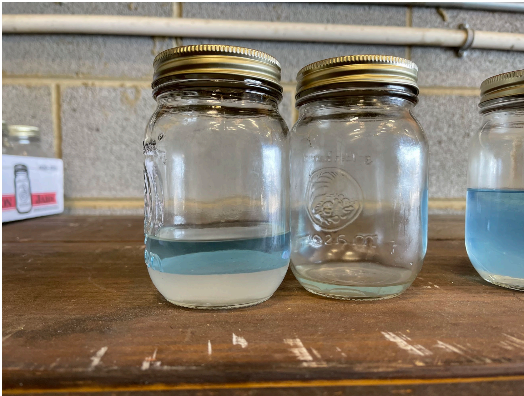
Photo 5 - Digital Photograph From Recovery Company. Left Glass Jar Contains 2.5 ounces of Blue Colored Fuel and 2.5 ounces of Water Drained from Carburetor During Postaccident Inspection.
