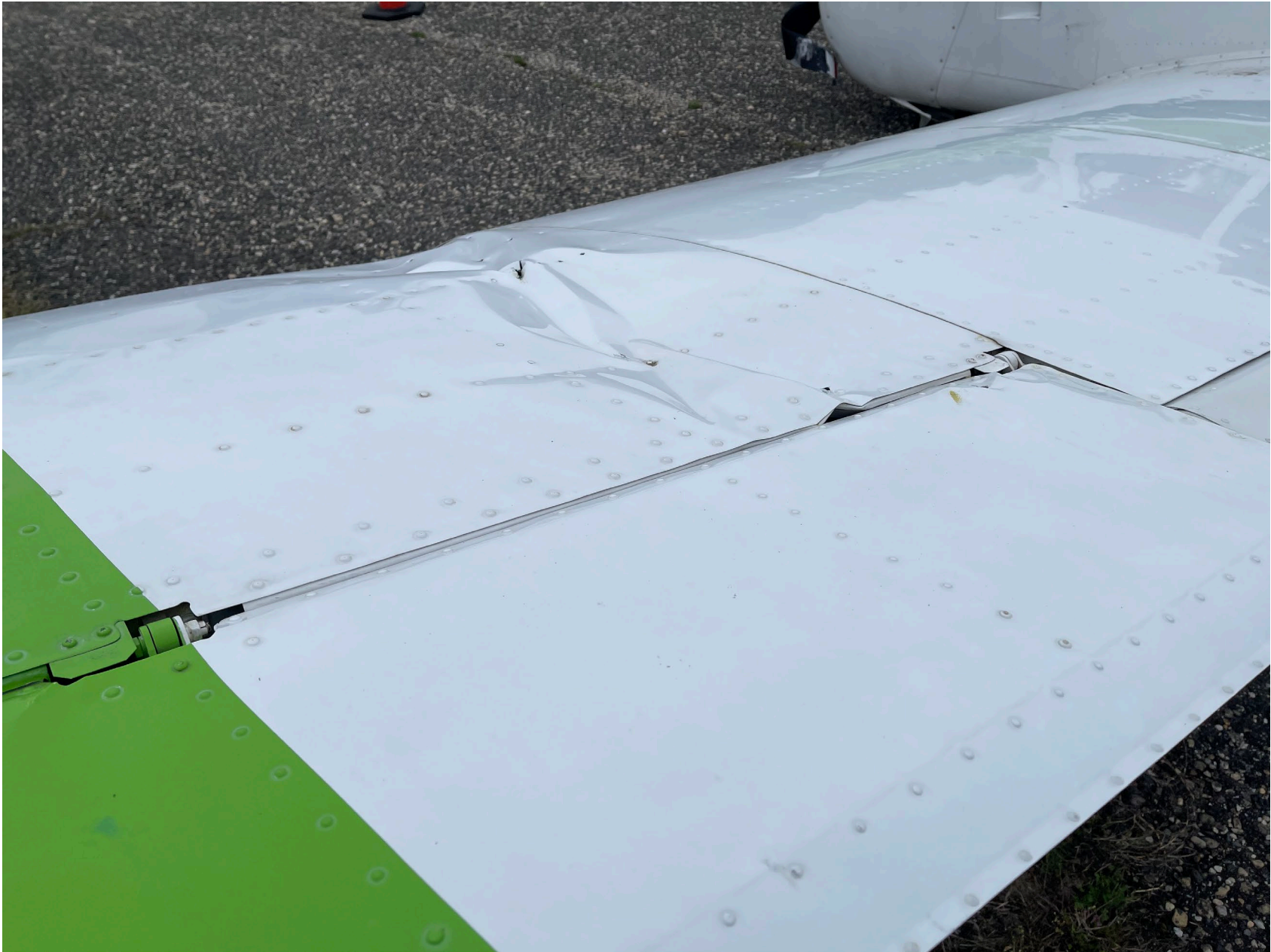
Photo 4 - Digital Photograph From Recovery Company. Rear View Looking Forward of a Portion of the Left Wing Depicting Structural Damage.
