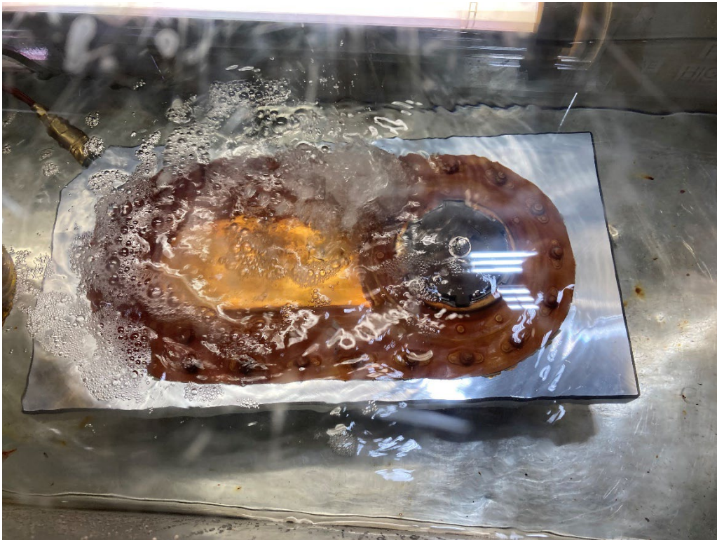
Figure 10: Right Panel Leak Test 25 psi
