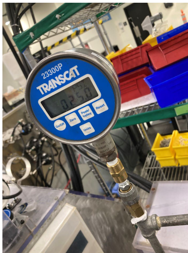
Figure 8: Left Cap-Adapter Leak Test 25 psi Gage
