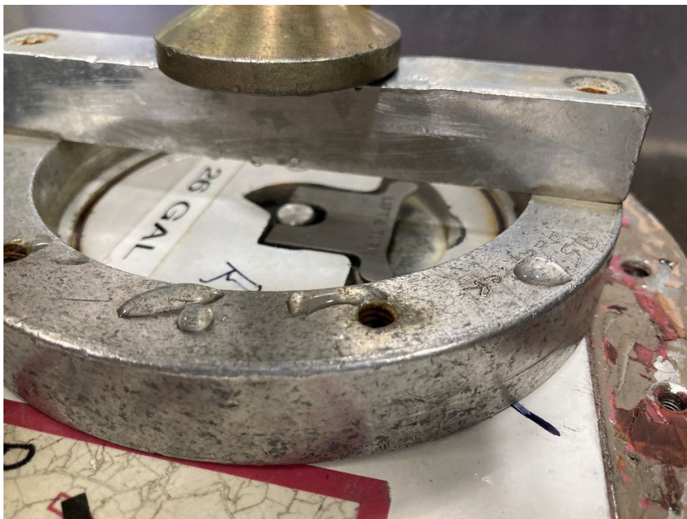
Figure 12: Right Cap-Adapter Leak Test 25 psi
