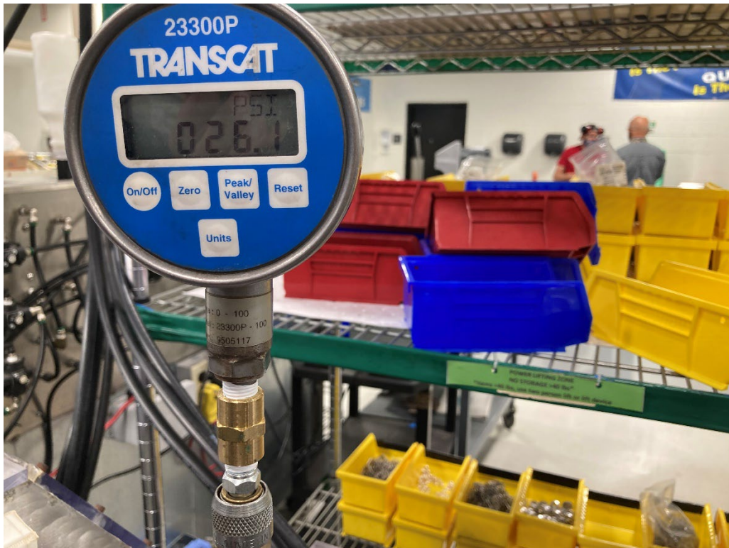
Figure 13: Right Cap-Adapter Leak Test 25 psi Gage
