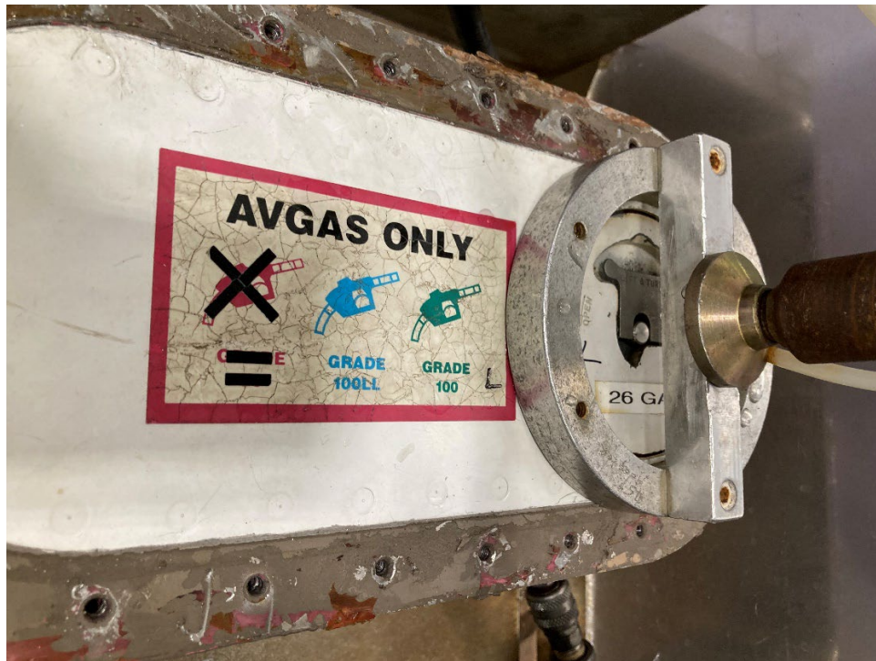
Figure 7: Left Cap-Adapter Leak Test 25 psi
