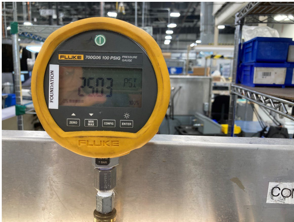
Figure 11: Right Panel Leak Test 25 psi Gage
