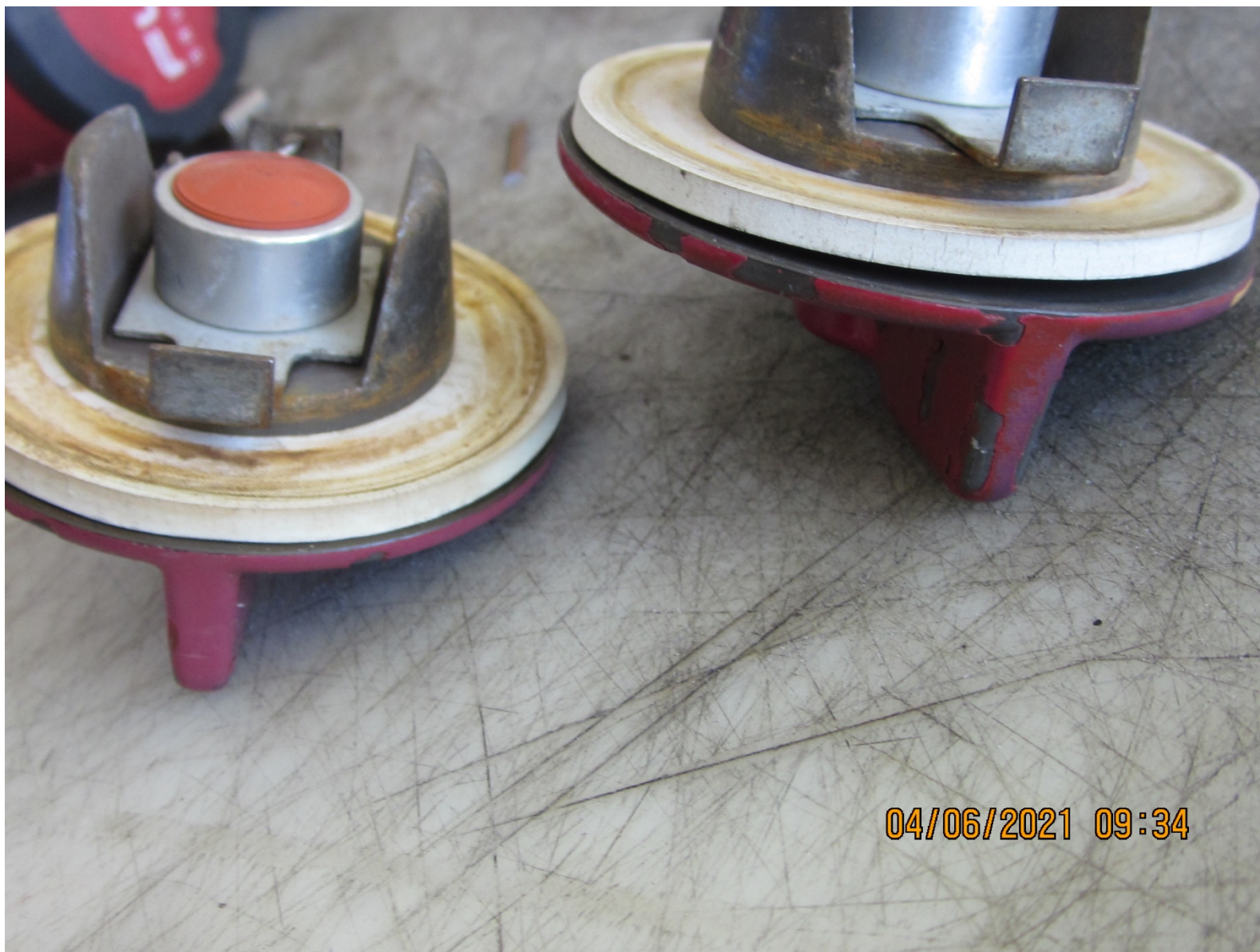
Photo 3 – View of fuel caps and seals. (Courtesy of FAA)
