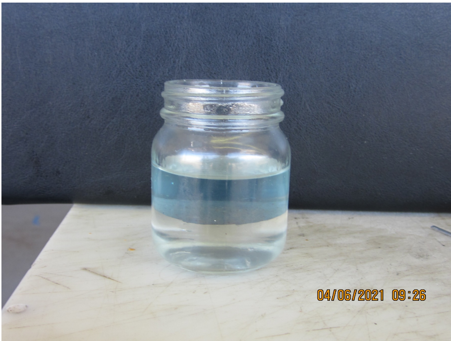
Photo 2 – View of contents drained from carburetor bowl. Note the water. (Courtesy of FAA)
