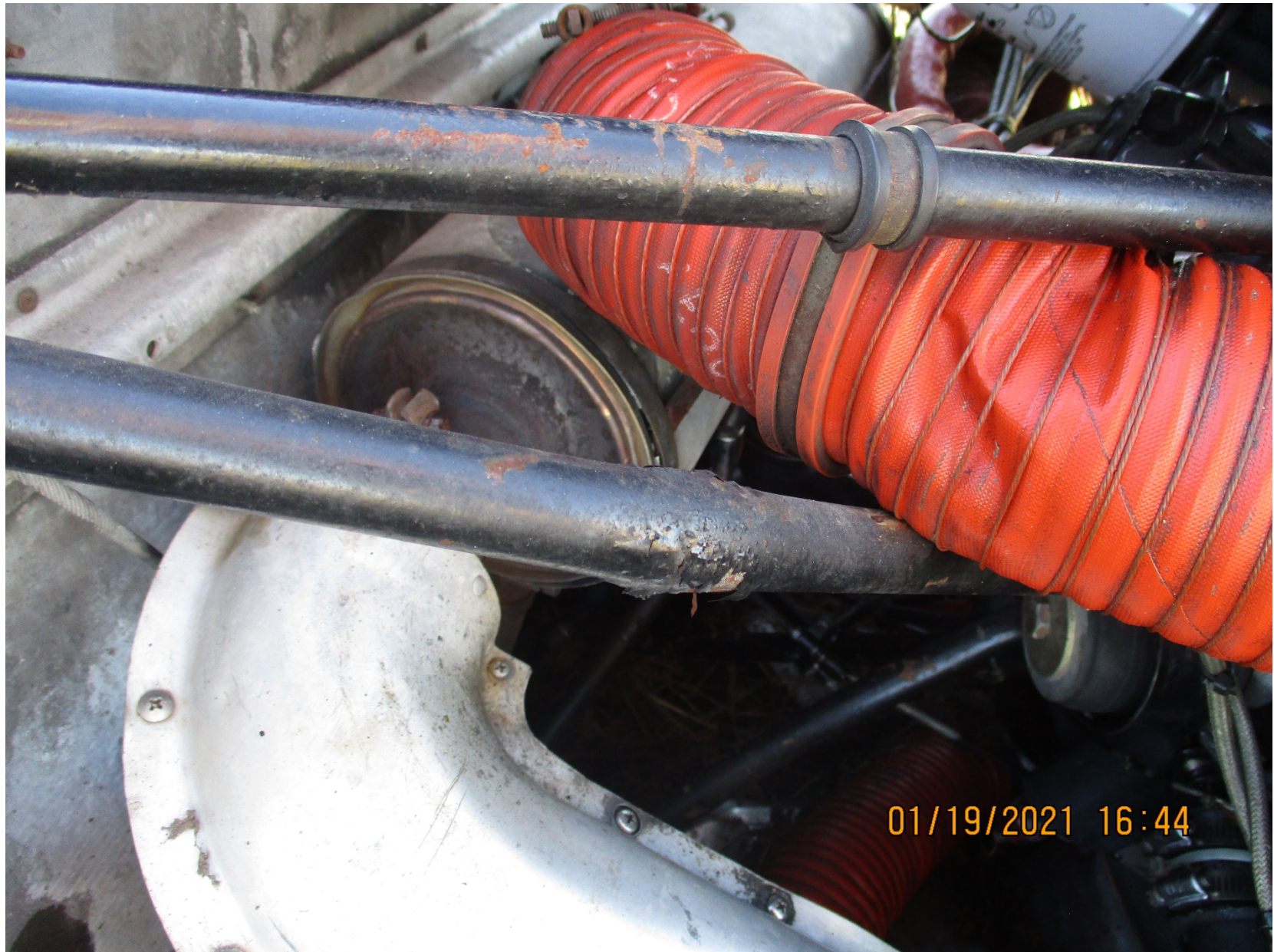
Photo 3 – Bent motor mount (FAA)
