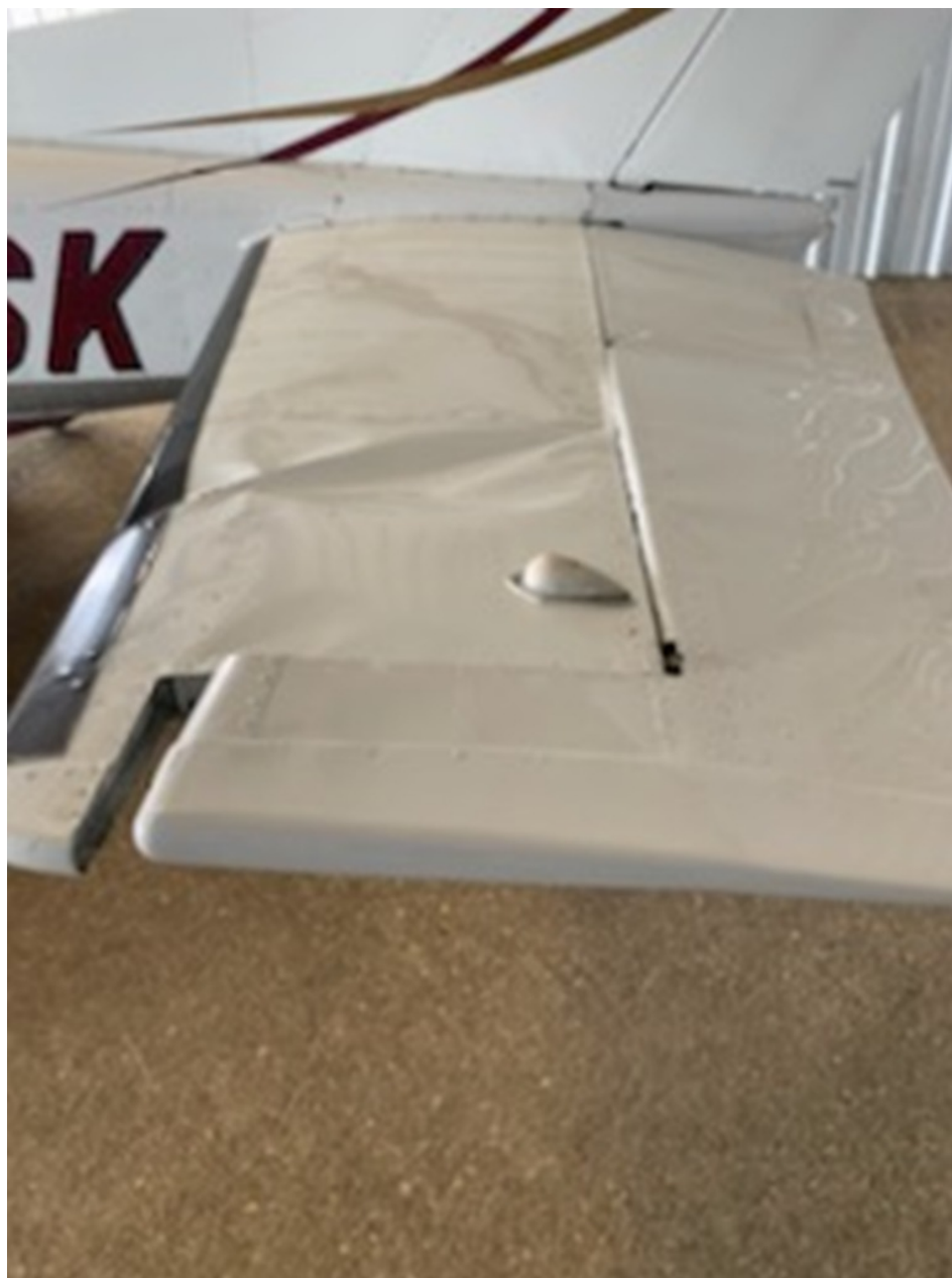
Photo 2 – Damage to Left Horizontal Stabilizer (photo provided by FAA)
