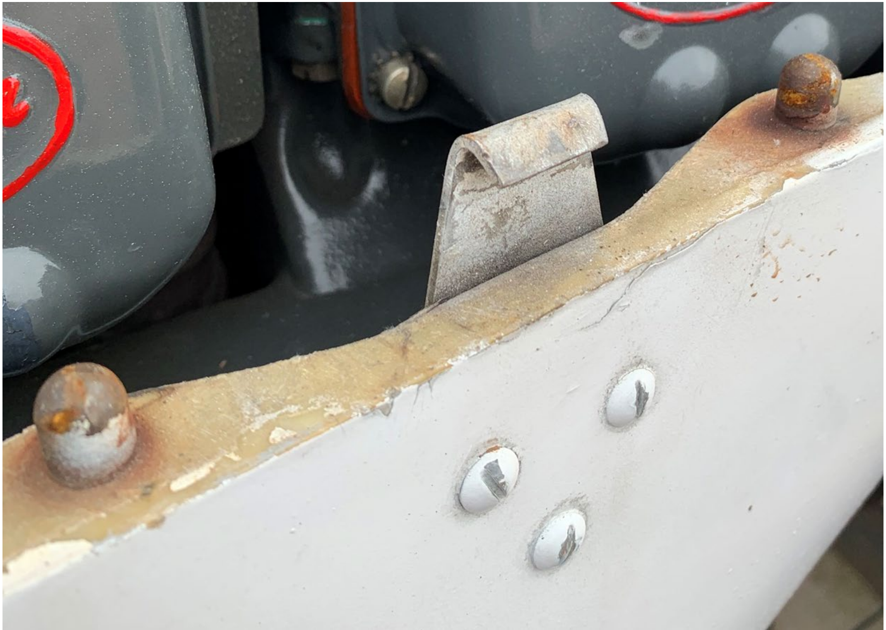
Photo 10 – Right Forward Lower Catch
