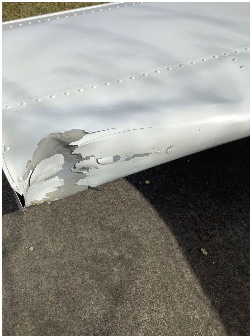
Photo 4 – Right Side of Horizontal Stabilizer – Courtesy of FAA
