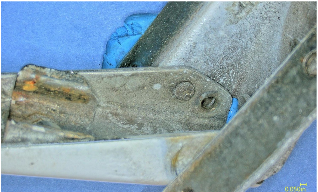
Figure 12 – Angled view of the left side pinhole and rivet of the broken latch.
