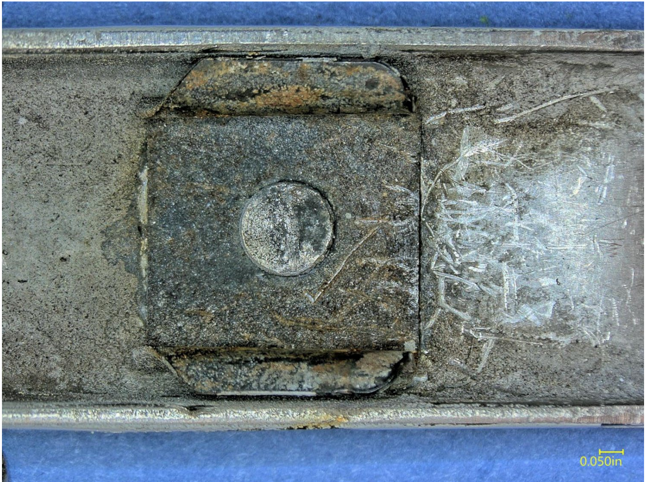
Figure 6 – View of the riveted clasp of the fractured latch.
