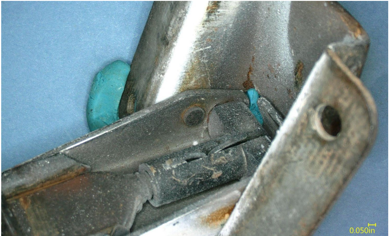
Figure 11 – Angled view of the left side pin and rivet attachments of the intact latch.
