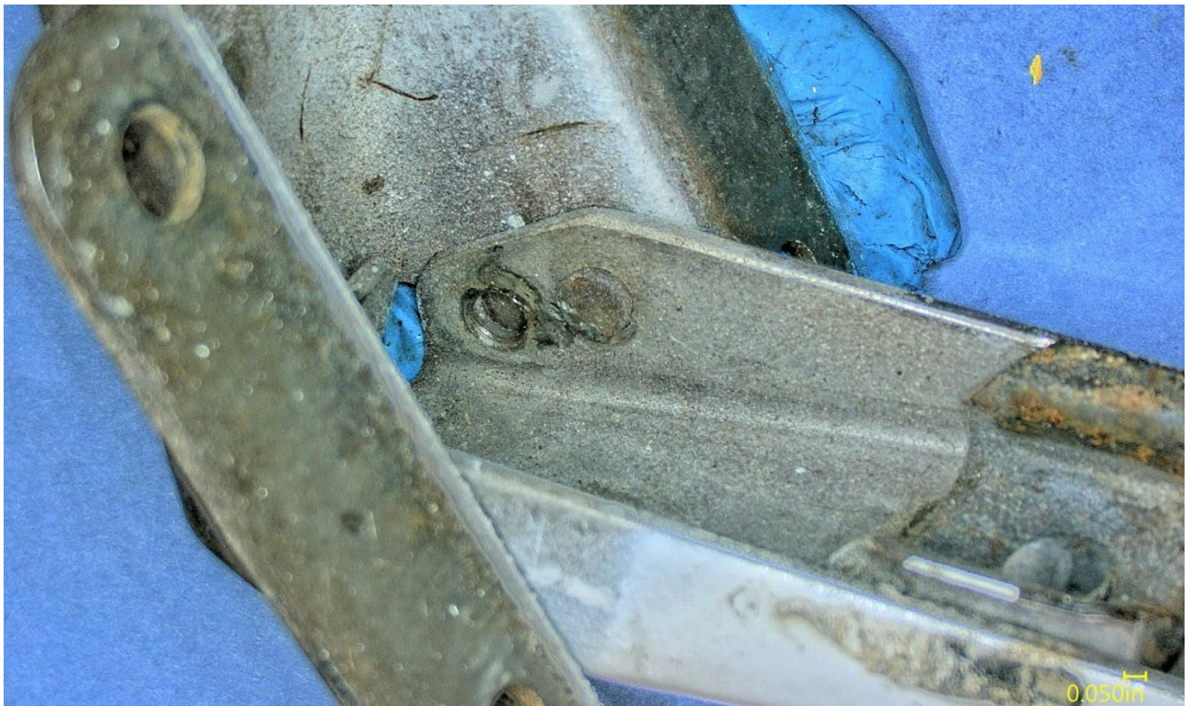
Figure 8 – Angled view of the right side pinhole and rivet of the broken latch.
