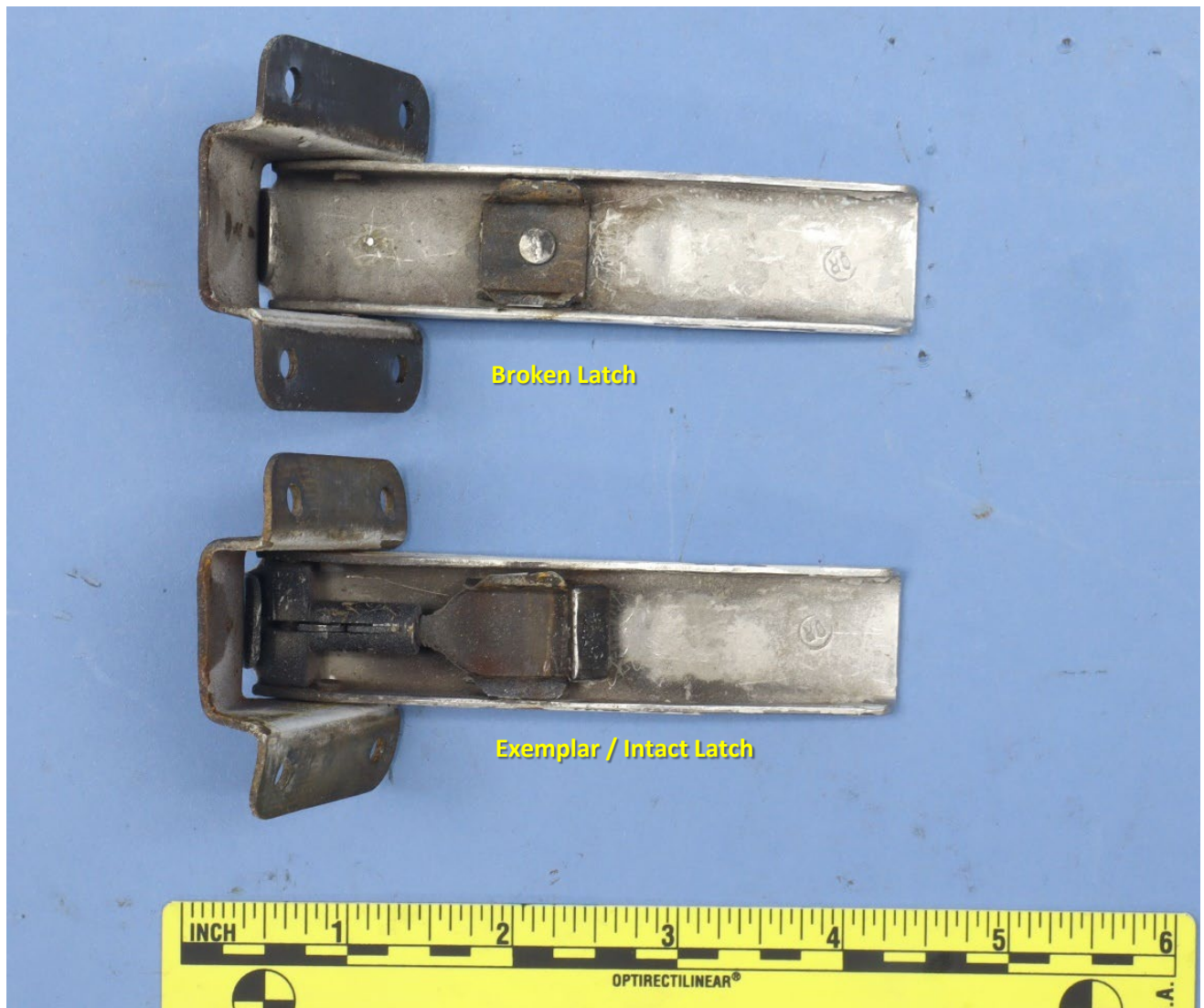
Figure 3 – View of the cowling latches, as received. The latches are in the open position, showing the missing hook and shaft subassembly in the upper latch.
