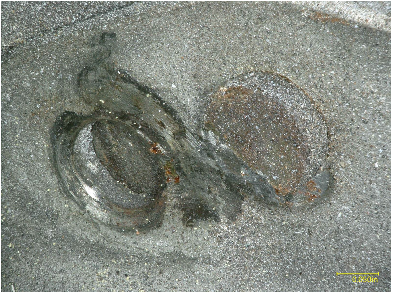
Figure 9 – Closer view of the right side rivet and pin hole from the latch interior in Figure 8.
