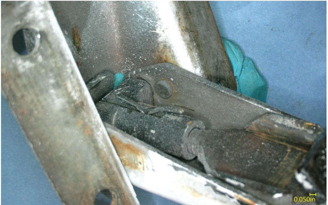
Figure 7 – Angled view of the right side pin and rivet attachments of the intact latch.
