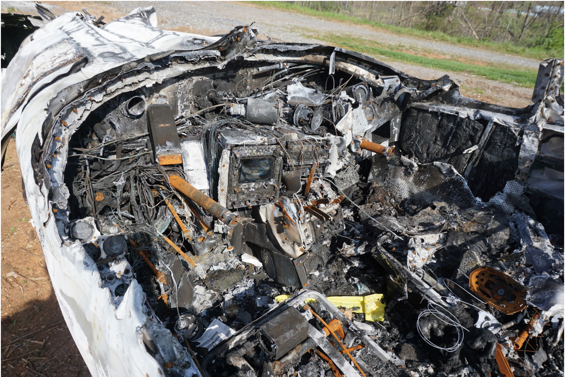
Photo 1 – View of post-fire damaged cockpit
