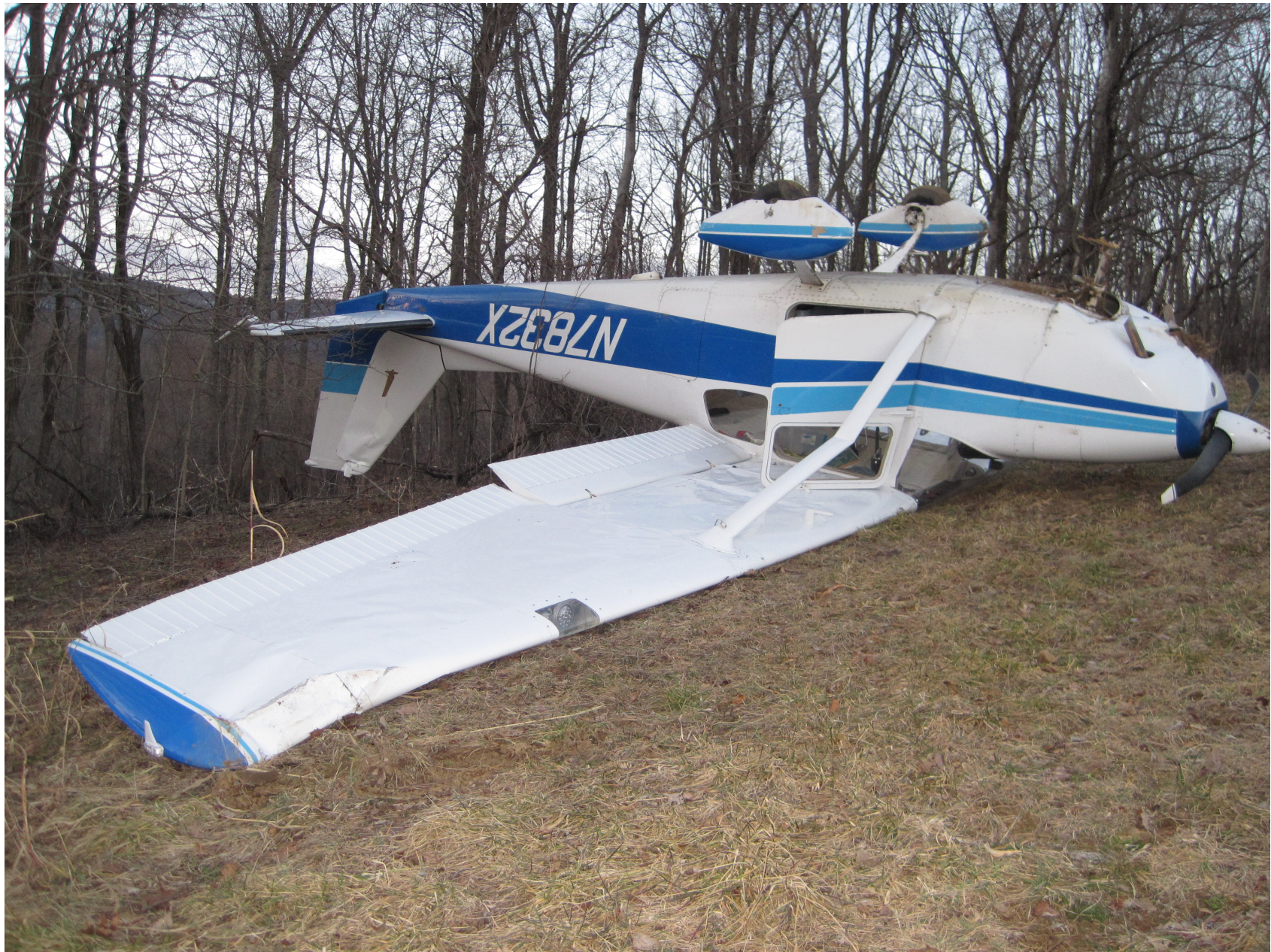
Photo 1 – View of airplane inverted showing left wing structural damage. (FAA Photo)
