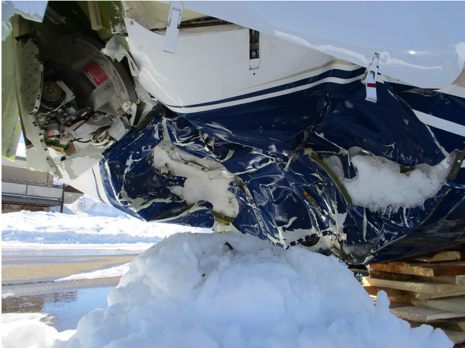
Damage to Underside of Forward Fuselage (Photo Courtesy FAA)
