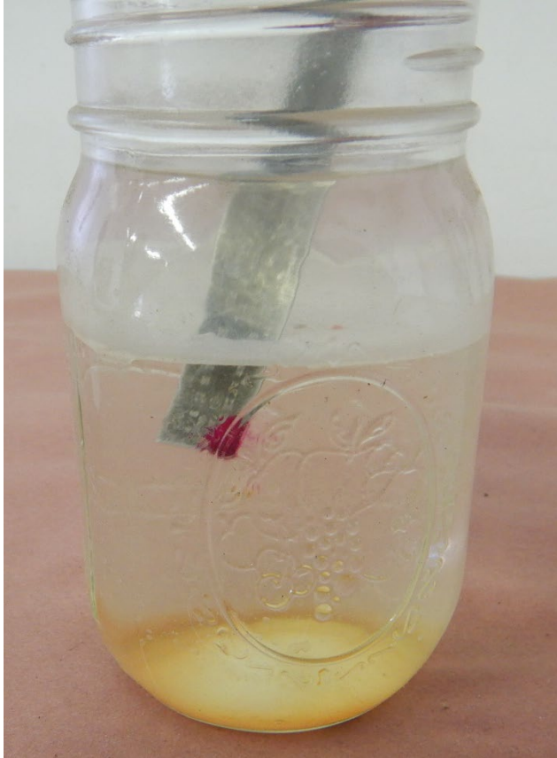
Figure 6: Left wing fuel sample with water contamination
