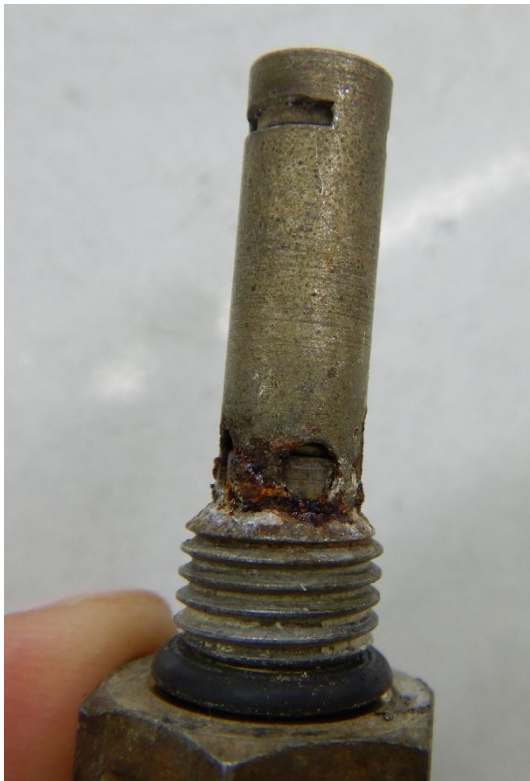
Figure 9: Right fuel sump exhibiting corrosion
