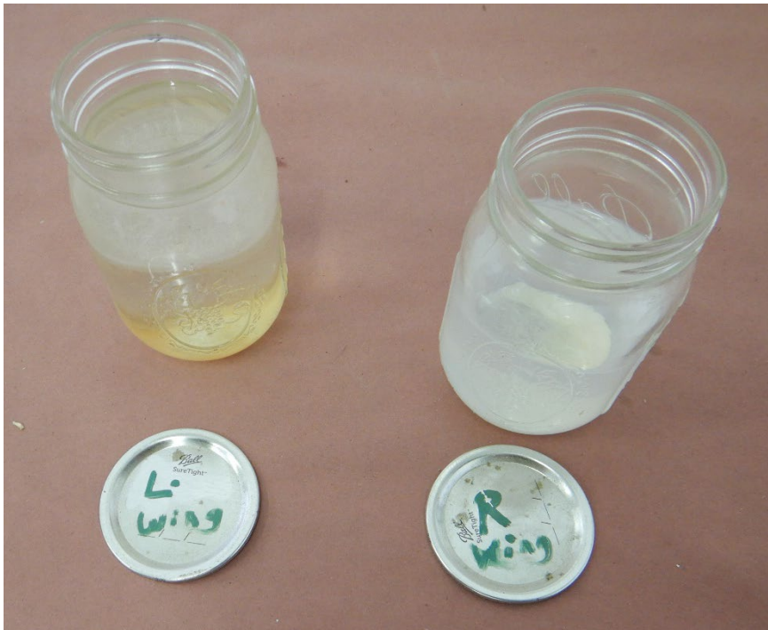
Figure 7: Left- and right-wing fuel samples from accident site showed contamination
