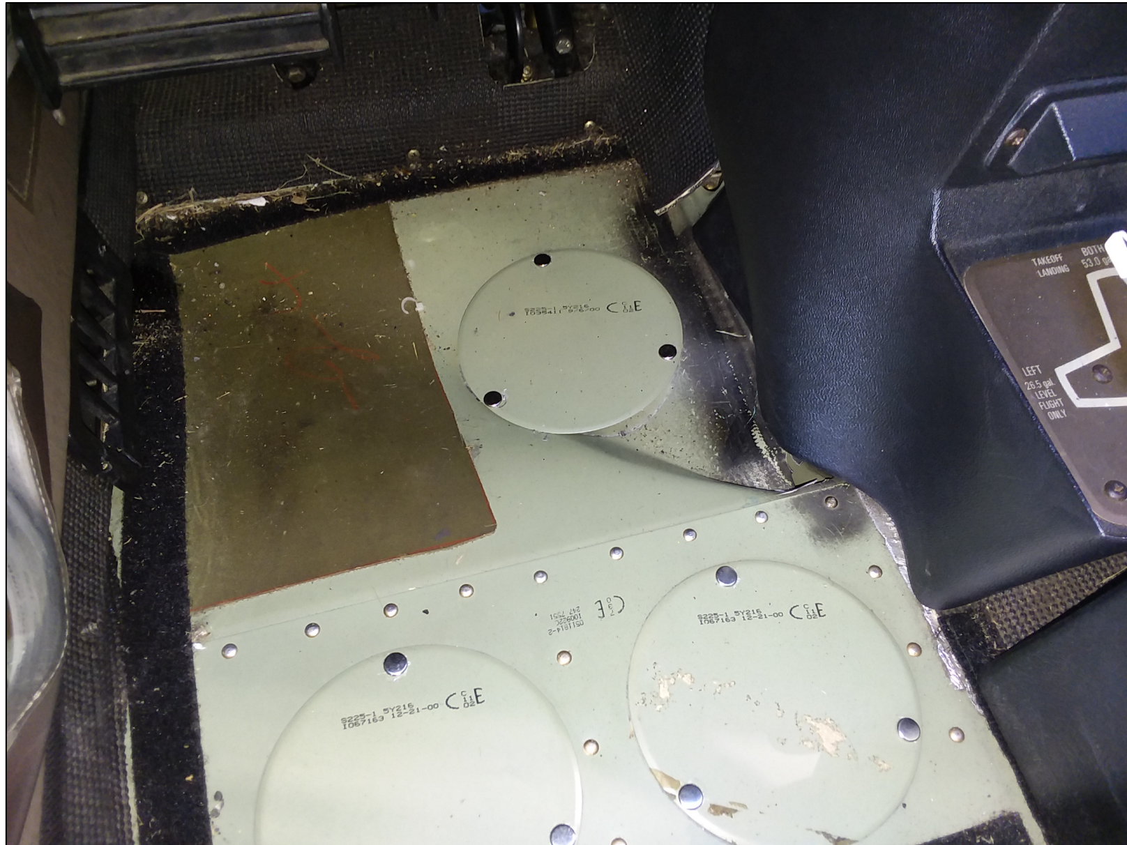
Photo 2 – Substantially damaged lower fuselage area located on left side of cockpit (Photo Courtesy of FAA)
