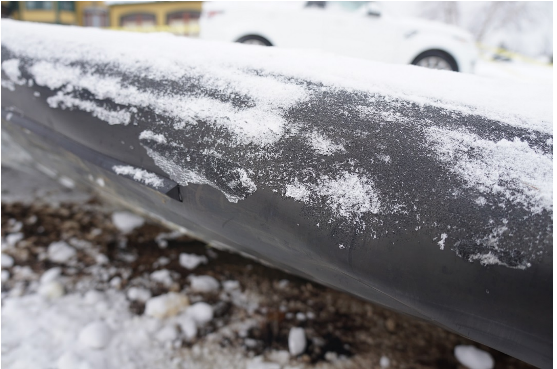
Photo 3 – Right Wing Leading Edge Ice (Photo Courtesy of FAA)
