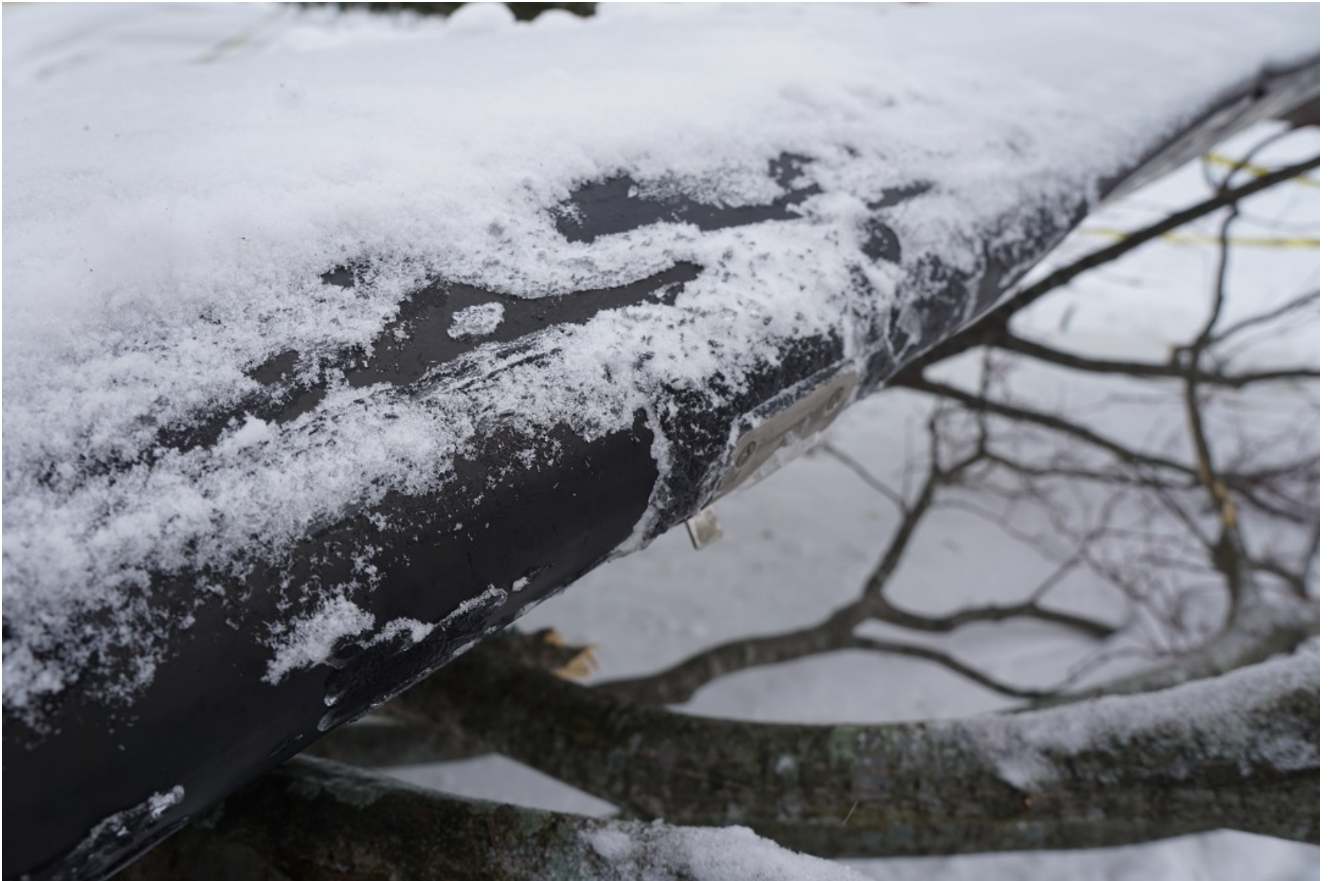
Photo 2 - Left Wing Leading Edge Ice (Photo Courtesy of FAA)
