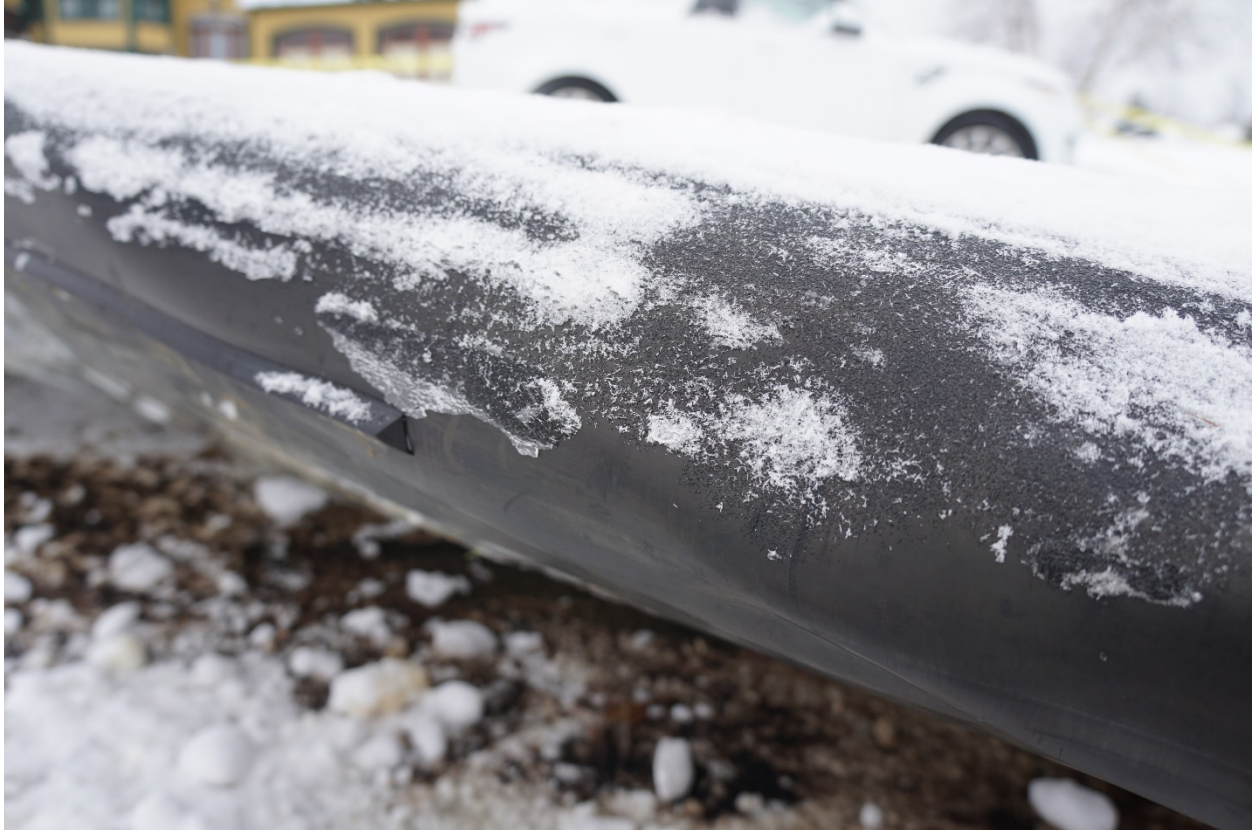
Figure 15 – Icing on the accident aircraft’s wings after the accident.
