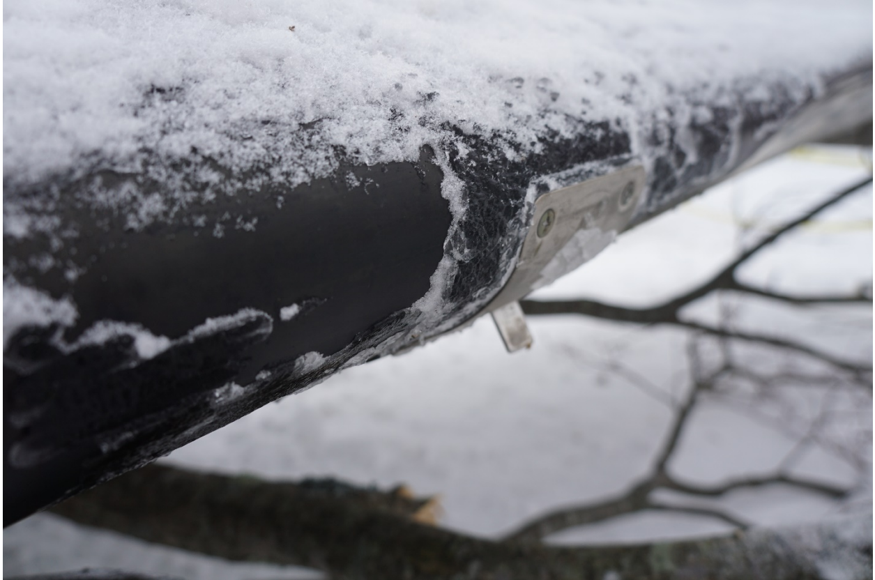
Figure 13 – Icing on the accident aircraft’s wing after the accident.
