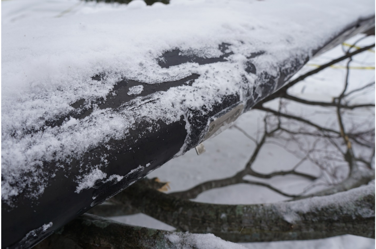
Figure 14 – Icing on the accident aircraft’s wing after the accident.
