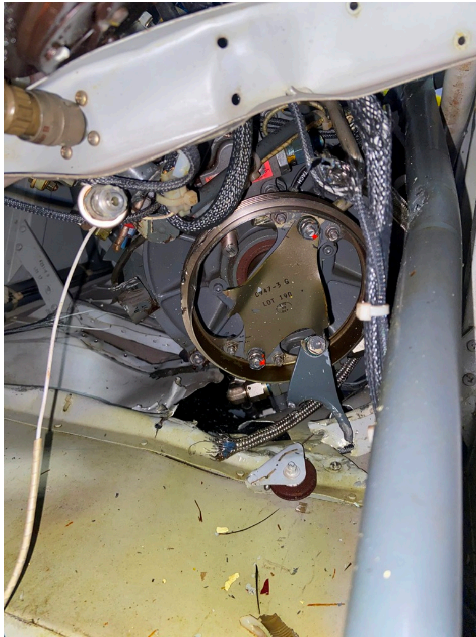
Photo 4 – Digital Photograph Provided by Jim Garst of Sevier County Choppers. View Depicting the Flex Plate Assembly Attached to the Yoke, the deformed and Fractured Flex Plate.
