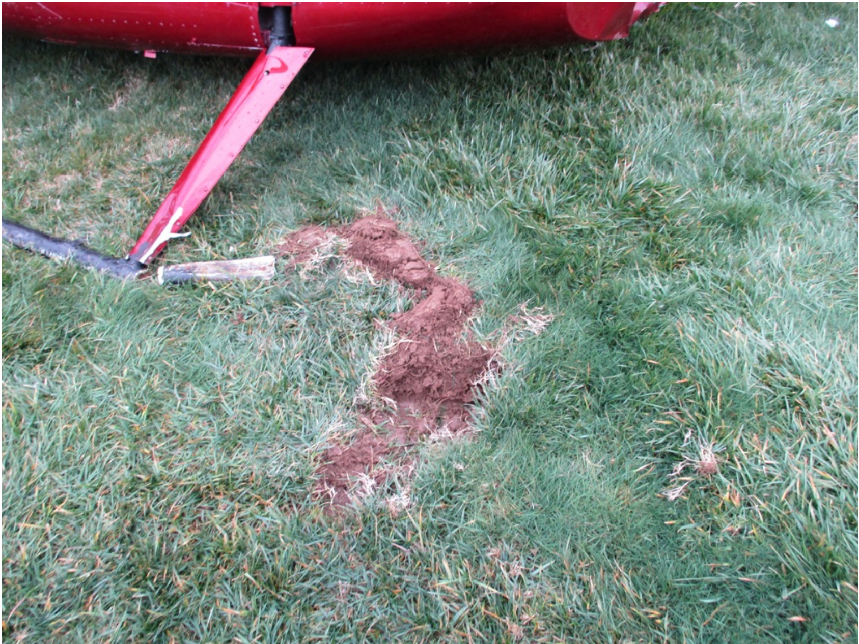
Photo 3 - FAA Digital Photograph. Close-Up View of the Ground Scar Made by and in Close Proximity to the Rear Portion of the Right Skid.
