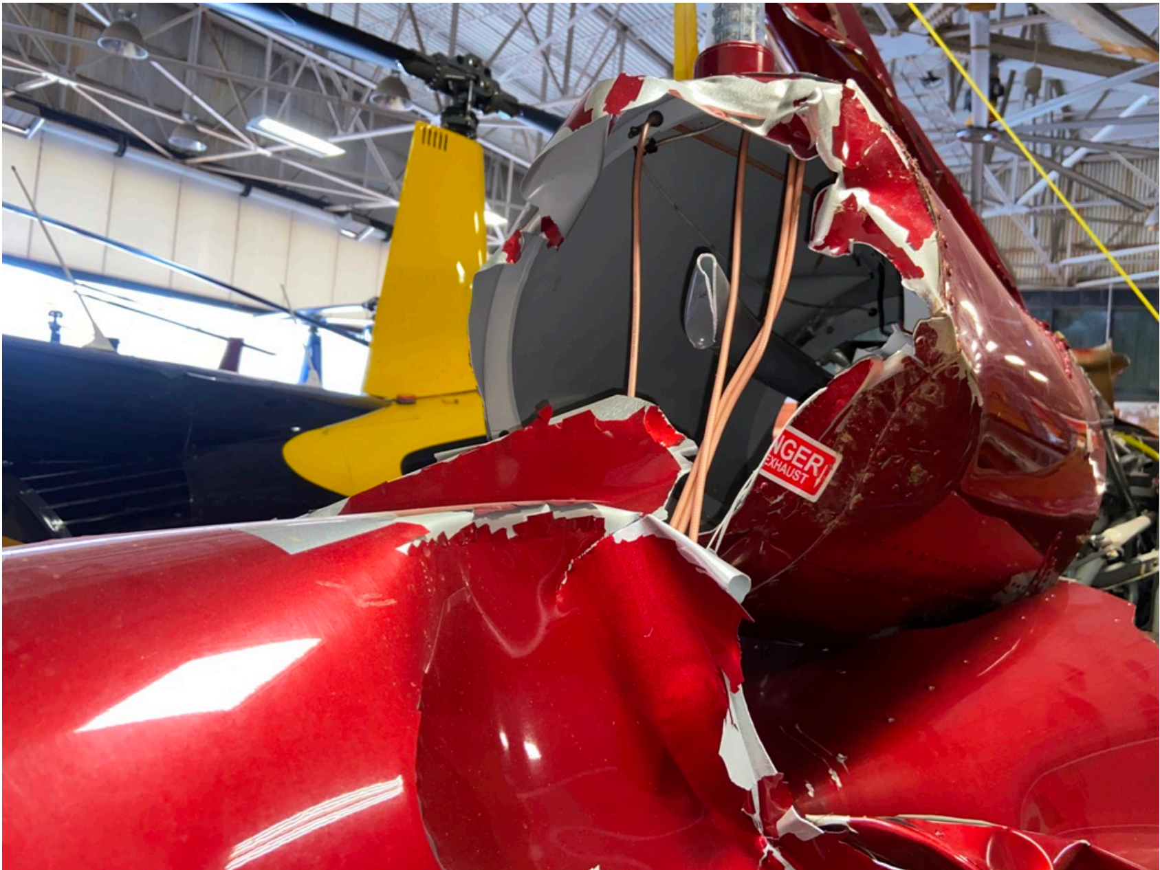
Photo 5 – Digital Photograph Provided by Jim Garst of Sevier County Choppers. View Depicting One end of the Fractured Tail Rotor Drive Shaft. Note the Deformation.
