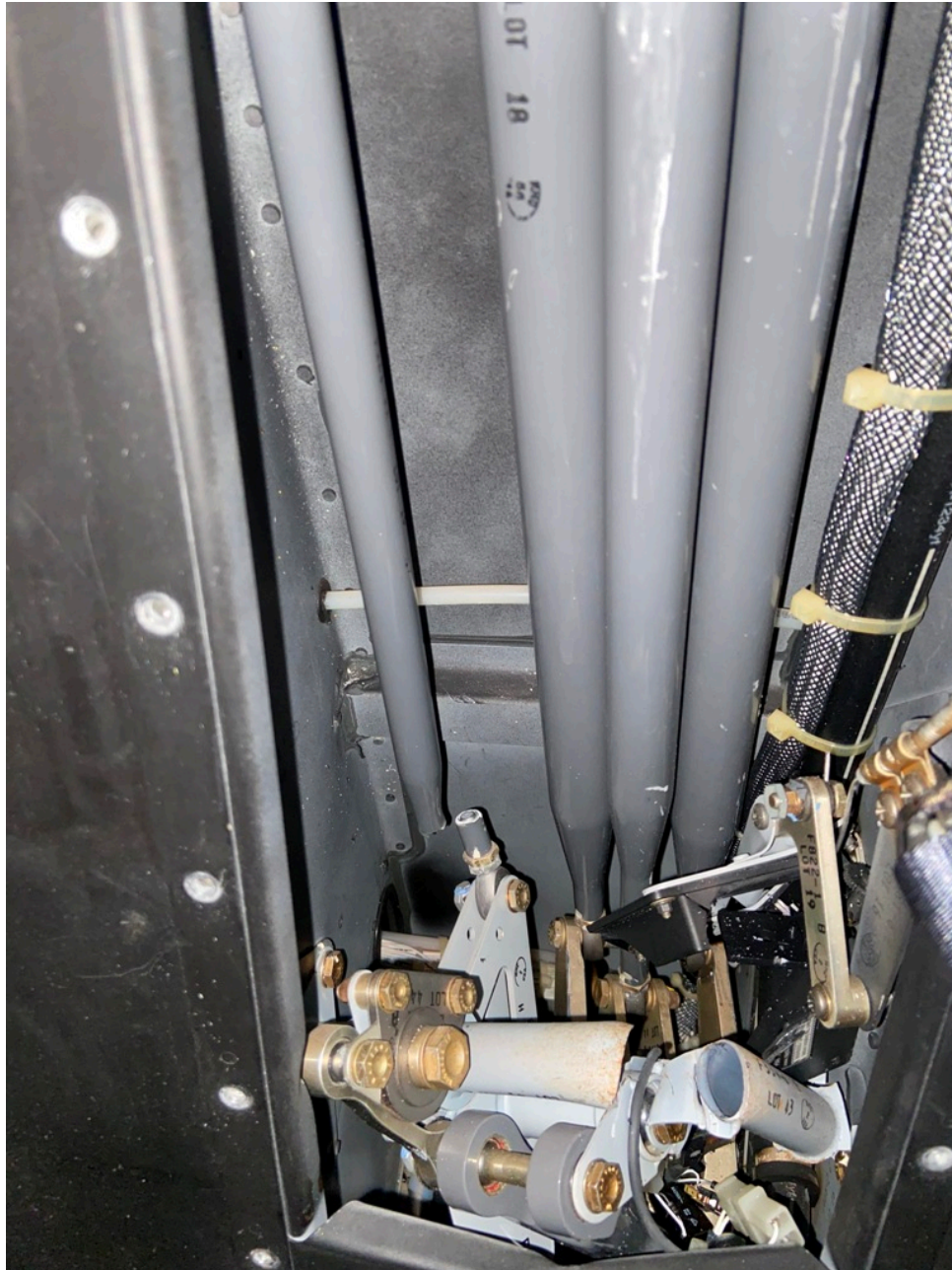
Photo 7 – Digital Photograph Provided by Jim Garst of Sevier County Choppers. View Depicting the Fractured Push-Pull Tube Assembly of the Anti-Torque Control. Note the Fractured Aft Support.
