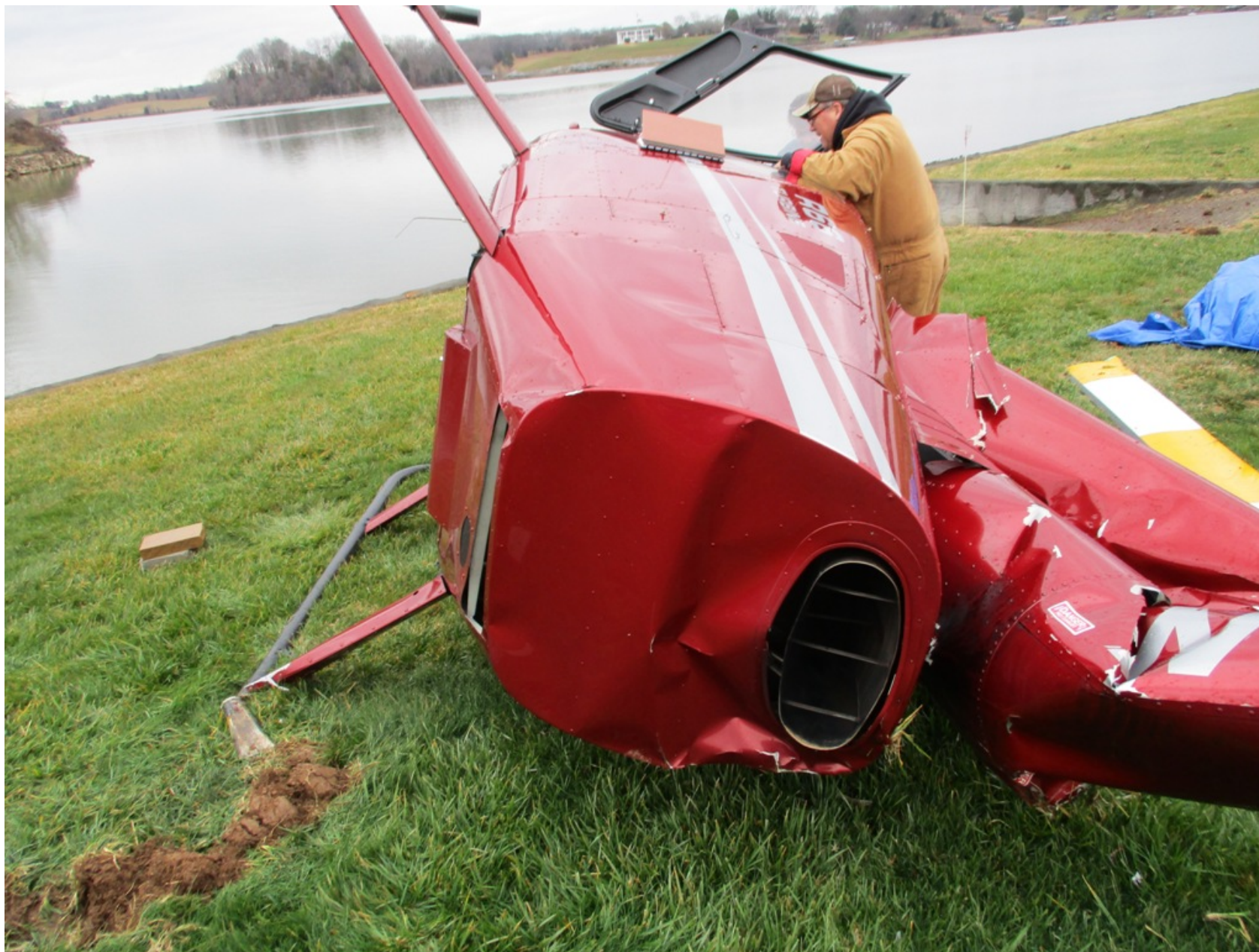
Photo 2 - FAA Digital Photograph. Rear View of the Helicopter Resting on Its Right Side at the Accident Site. Note the Damaged Tailboom Assembly and the Ground Scar near the Rear Right Skid.
