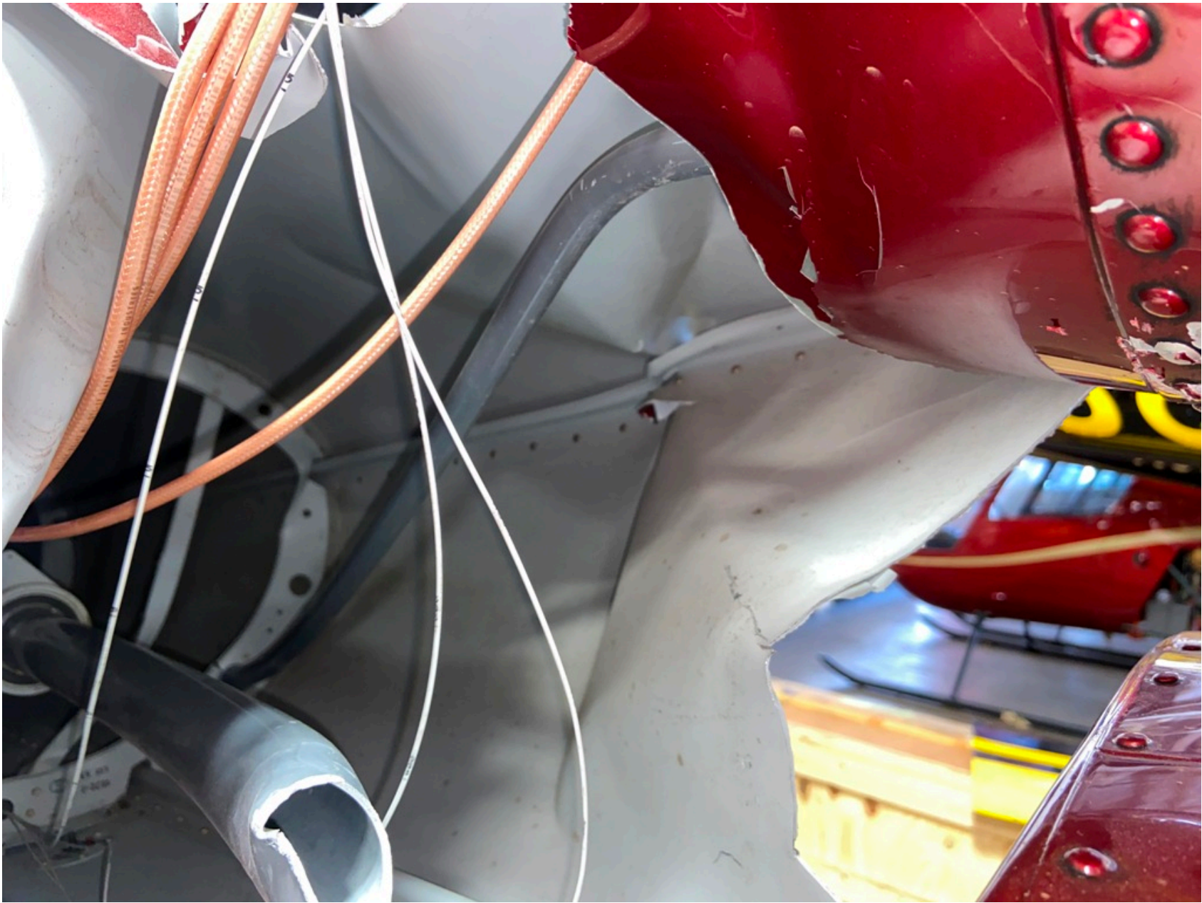
Photo 8 – Digital Photograph Provided by Jim Garst of Sevier County Choppers. View Depicting the Bending Deformation of the Push-Pull Tube Assembly P/N C121-17.
