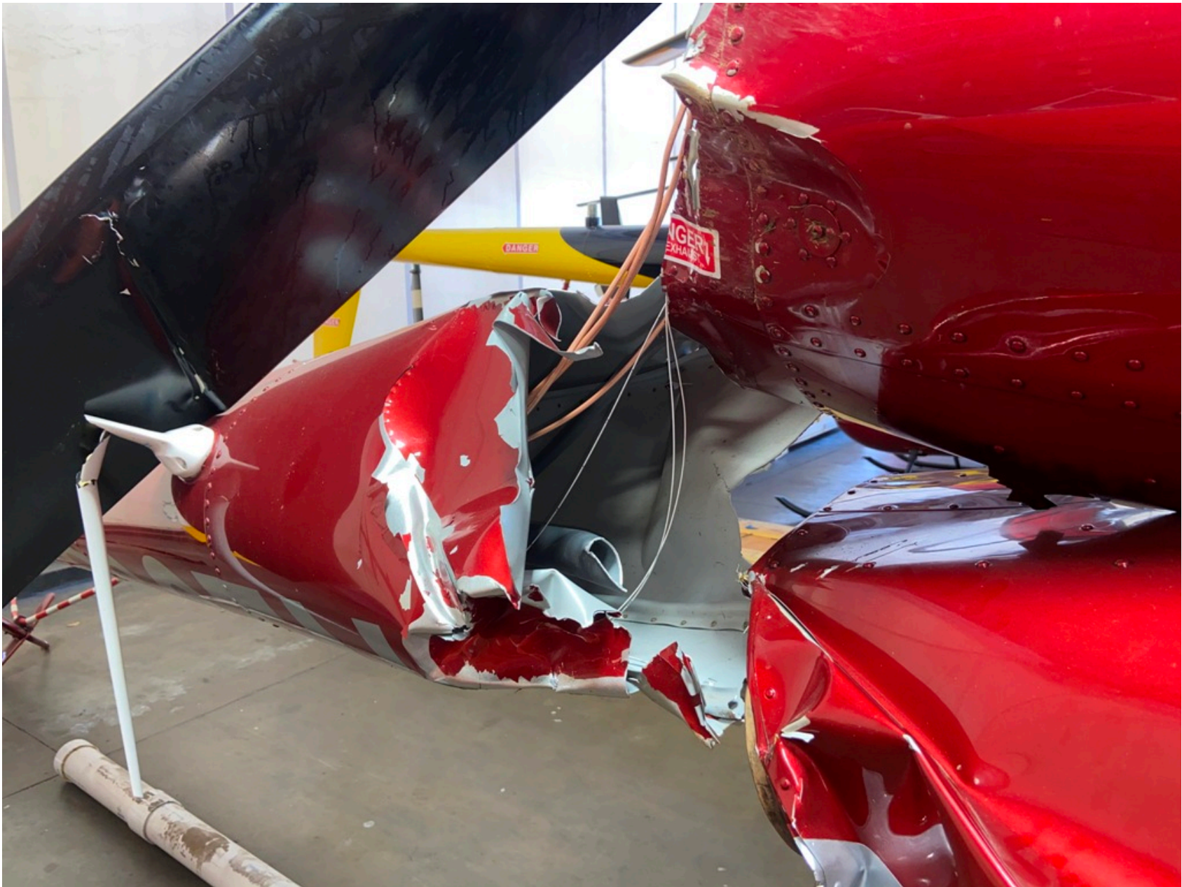
Photo 6 – Digital Photograph Provided by Jim Garst of Sevier County Choppers. View Depicting Opposite end of the Fractured Tail Rotor Drive Shaft. Note the “D” Shaped Deformation.
