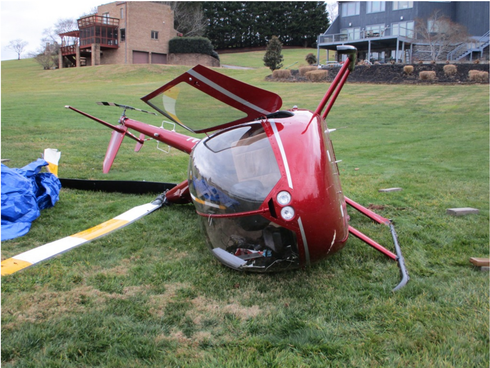
Photo 1 – FAA Digital Photograph. Frontal View of the Helicopter Resting on Its Right Side at the Accident Site. Note the Displaced Tailboom Assembly.
