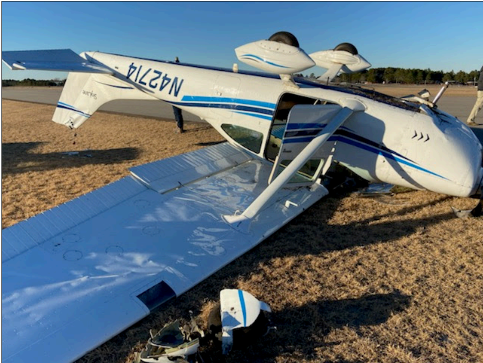
Photo 2 – Additional view of the nosed over airplane at the accident site (Photo Courtesy of FAA)
