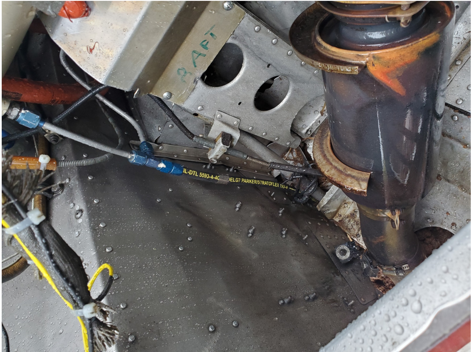
Photo 3 – damaged firewall (FAA)
