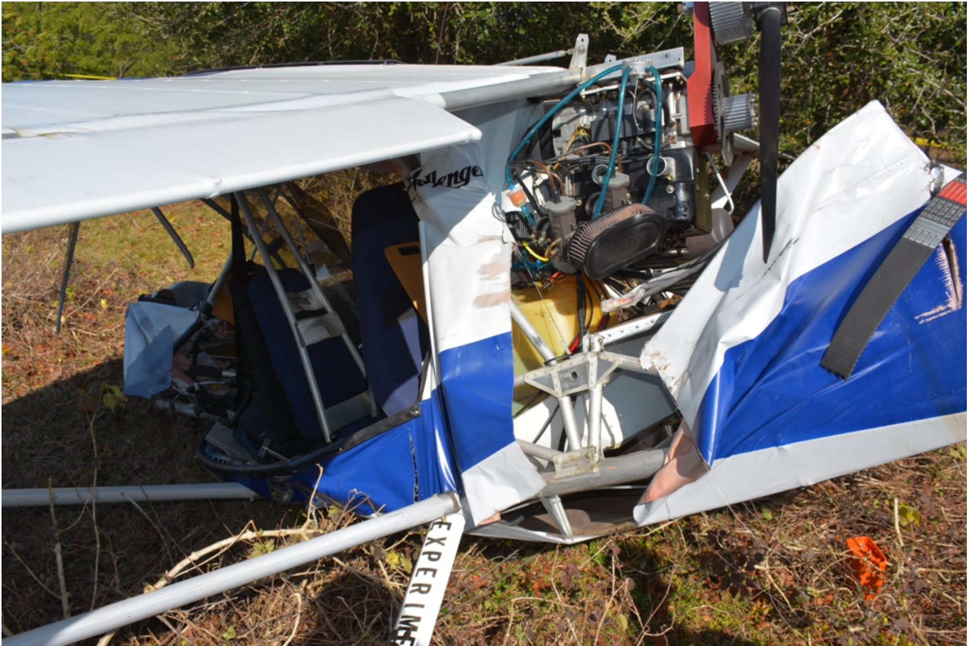
Photo 3 – Left Side of Engine and Broken Drive Belt on Right (Courtesy of Groveland PD).
