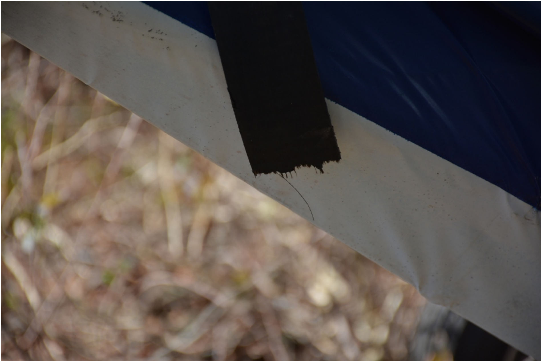
Photo 5 – Broken End of Drive Belt (Courtesy of Groveland PD).
