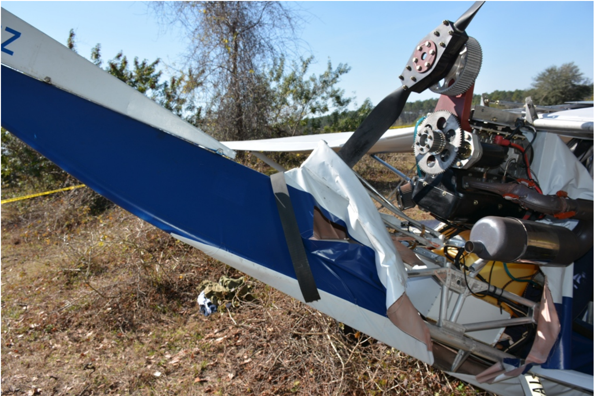
Photo 4 – Right Side of Engine and Broken Drive Belt on Left (Courtesy of Groveland PD).
