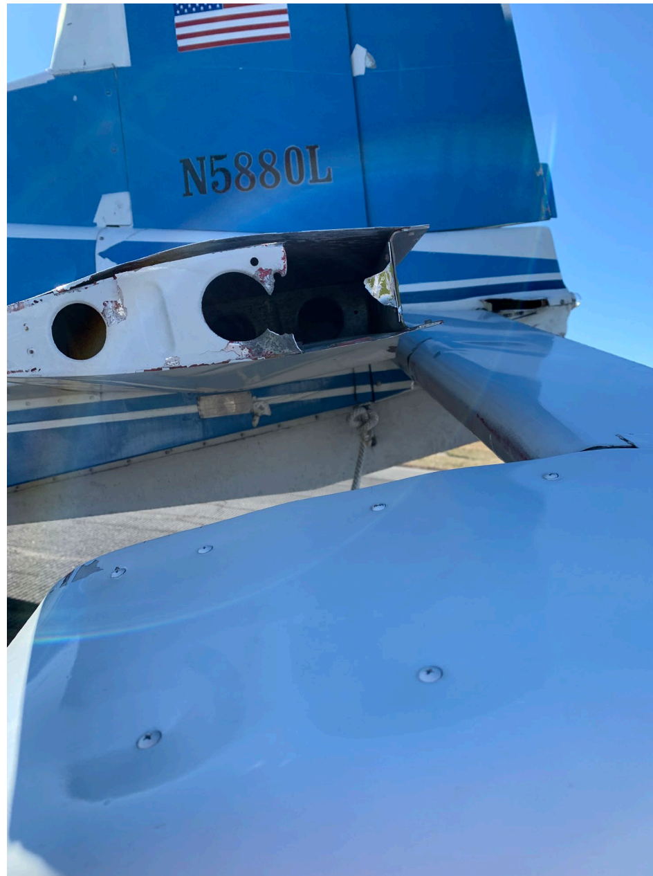
Photo 3 - FAA Digital Photograph. Left Side Close-Up View of the Damaged Outboard Rib of the Left Stabilizer, Displaced Left Elevator, and Portion of Vertical Stabilizer and Rudder.
