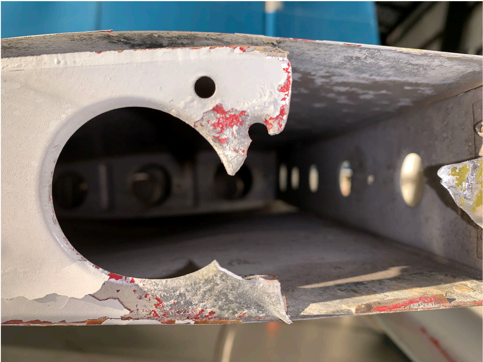
Photo 5 - FAA Digital Photograph. Close-Up View of the Aft Portion of the Outboard Rib of the Left Horizontal Stabilizer. Note the Missing section and Corrosion on the rib and also the Interior Surface of the Upper Skin.
