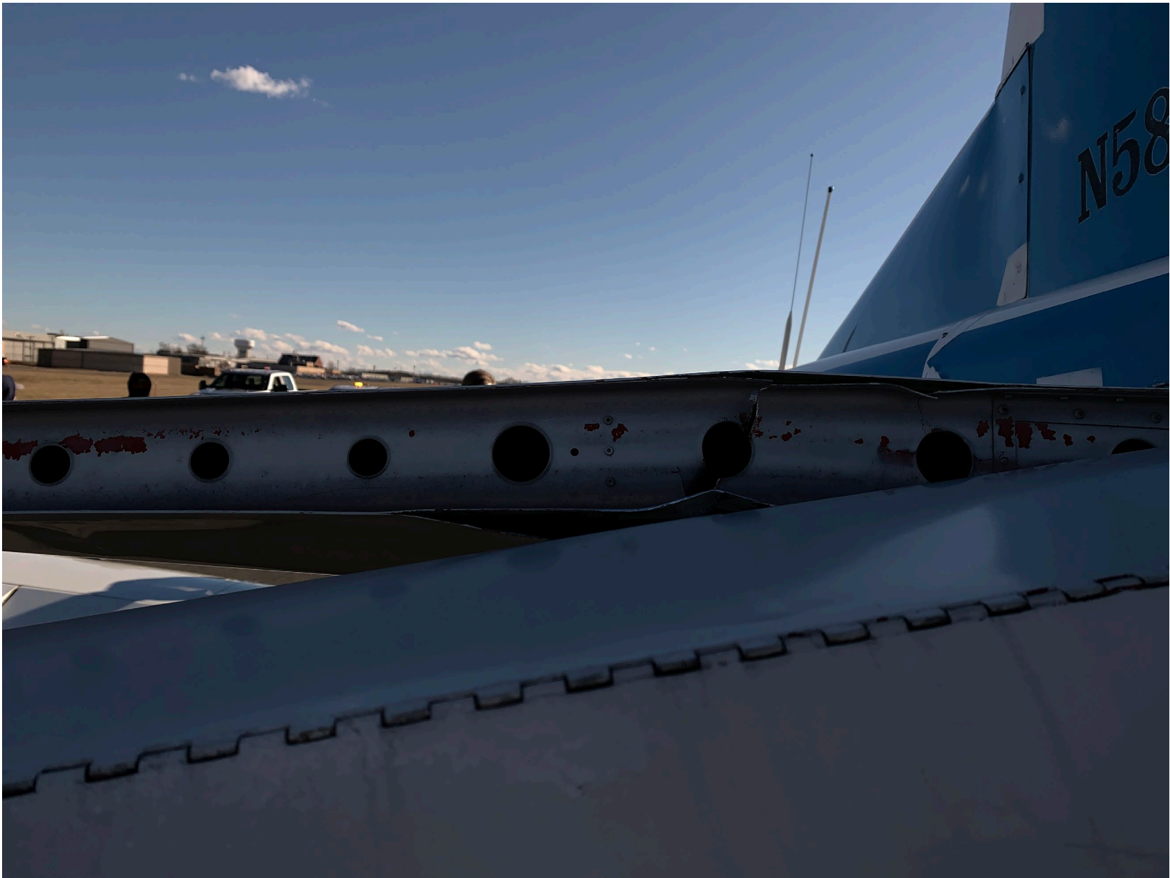
Photo 4 - FAA Digital Photograph. Aft Side View of the Structurally Damaged Aft Spar of the Left Stabilizer, Portion of Displaced Left Elevator.
