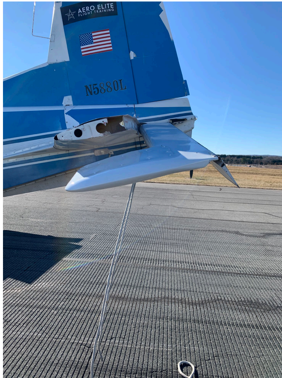
Photo 2 – FAA Digital Photograph. Left Side View Showing the Aft Empennage, Left Horizontal Stabilizer, Portion of the Vertical Stabilizer and rudder, and Displaced Left Elevator.
