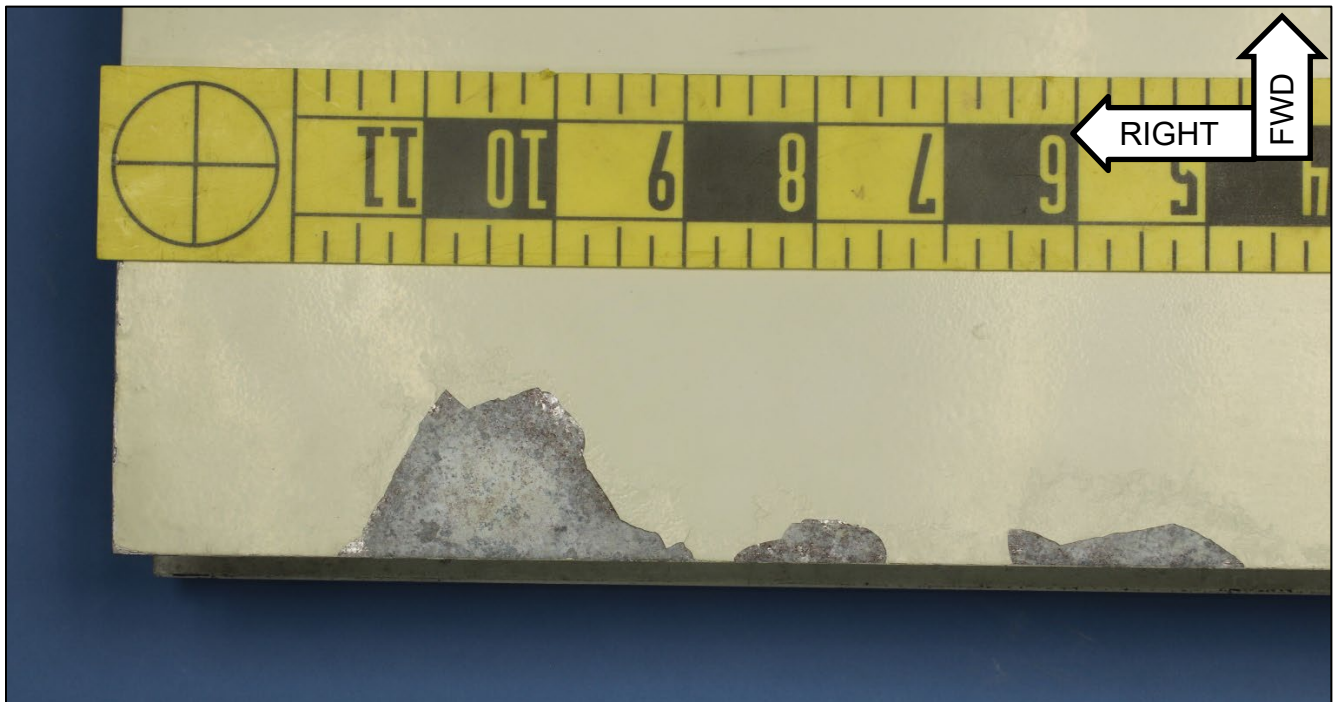
Figure 17. Outboard end of the exemplar right horizontal stabilizer showing corrosion with bubbled and missing paint on the lower skin at the trailing edge.
