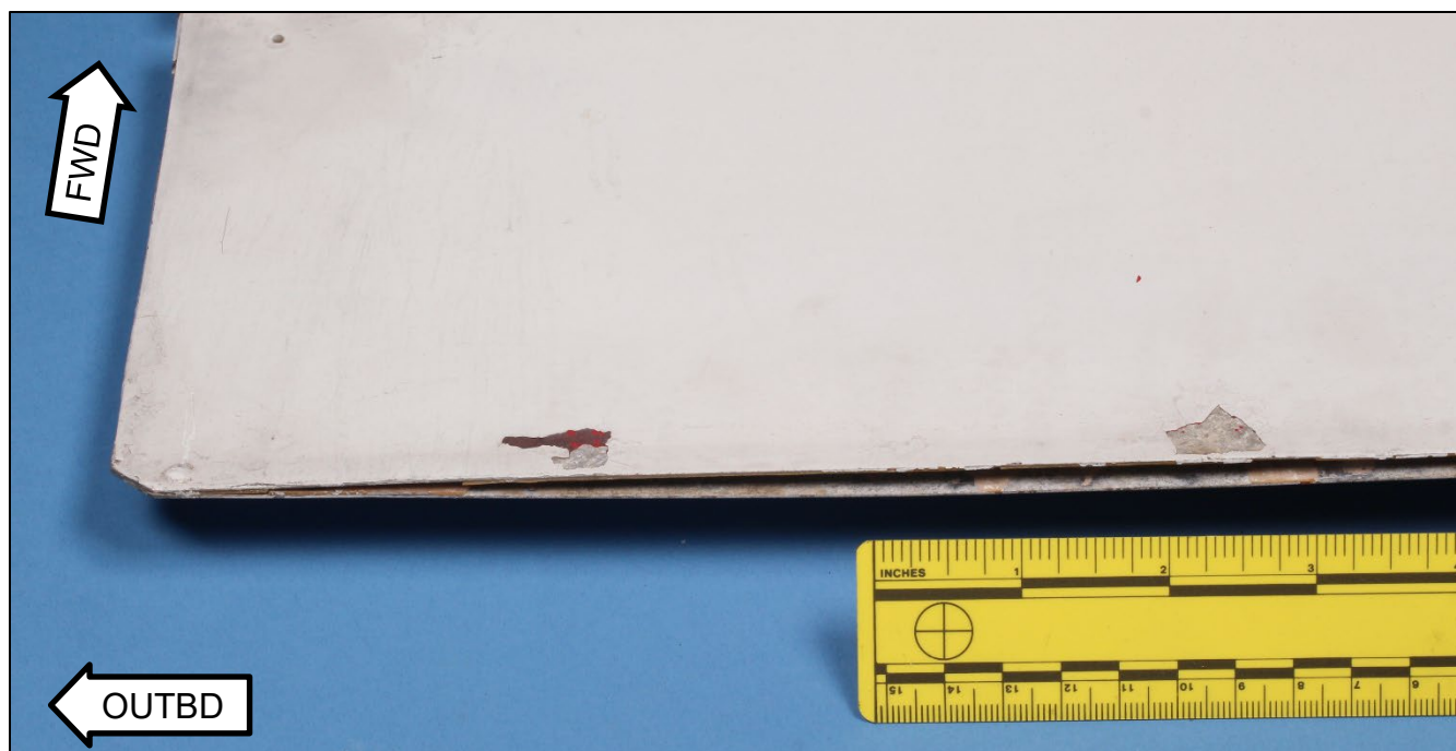
Figure 13. Outboard end of the left elevator trim tab showing bondline separation, corrosion, and bubbled paint along the trailing edge.
