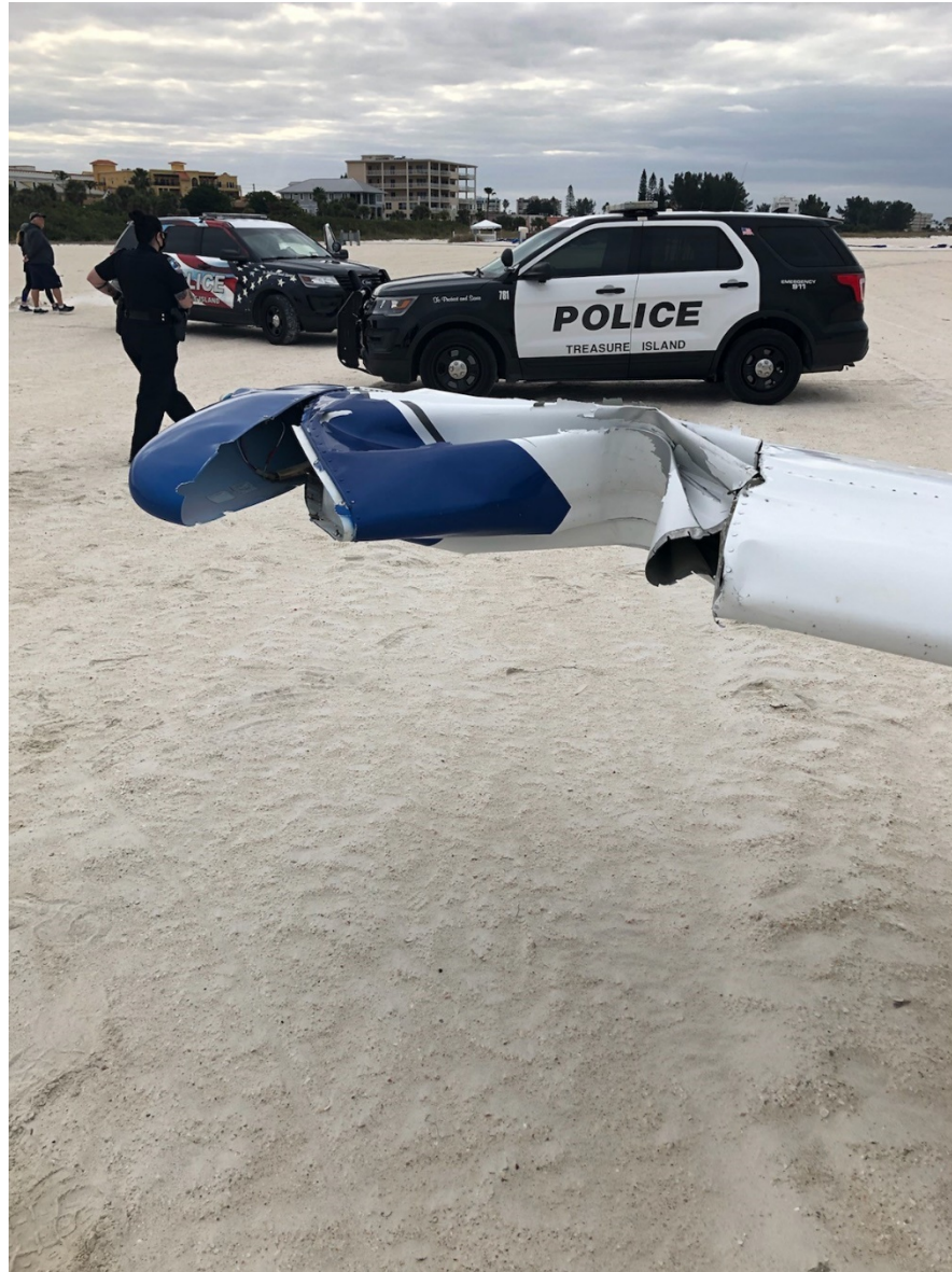
Photo 2 – View of right wing damage (Courtesy of FAA)
