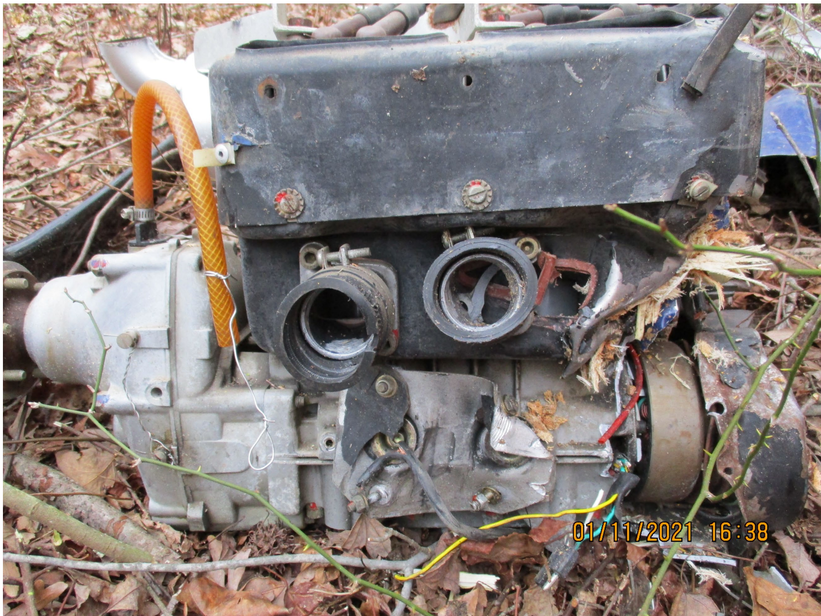
Photo 4 - Closeup of aircraft engine – note damage (courtesy of FAA)
