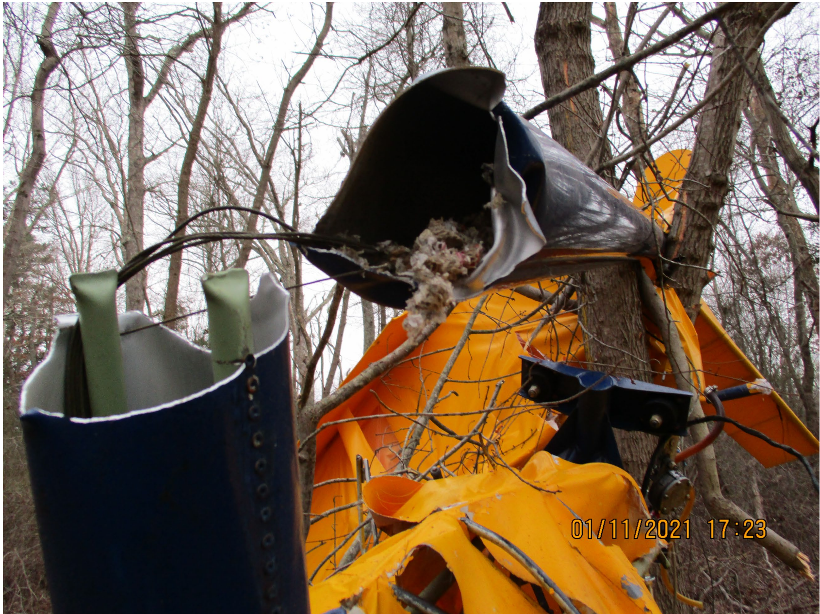
Photo 6 – Closeup of tail boom damage (courtesy of FAA)
