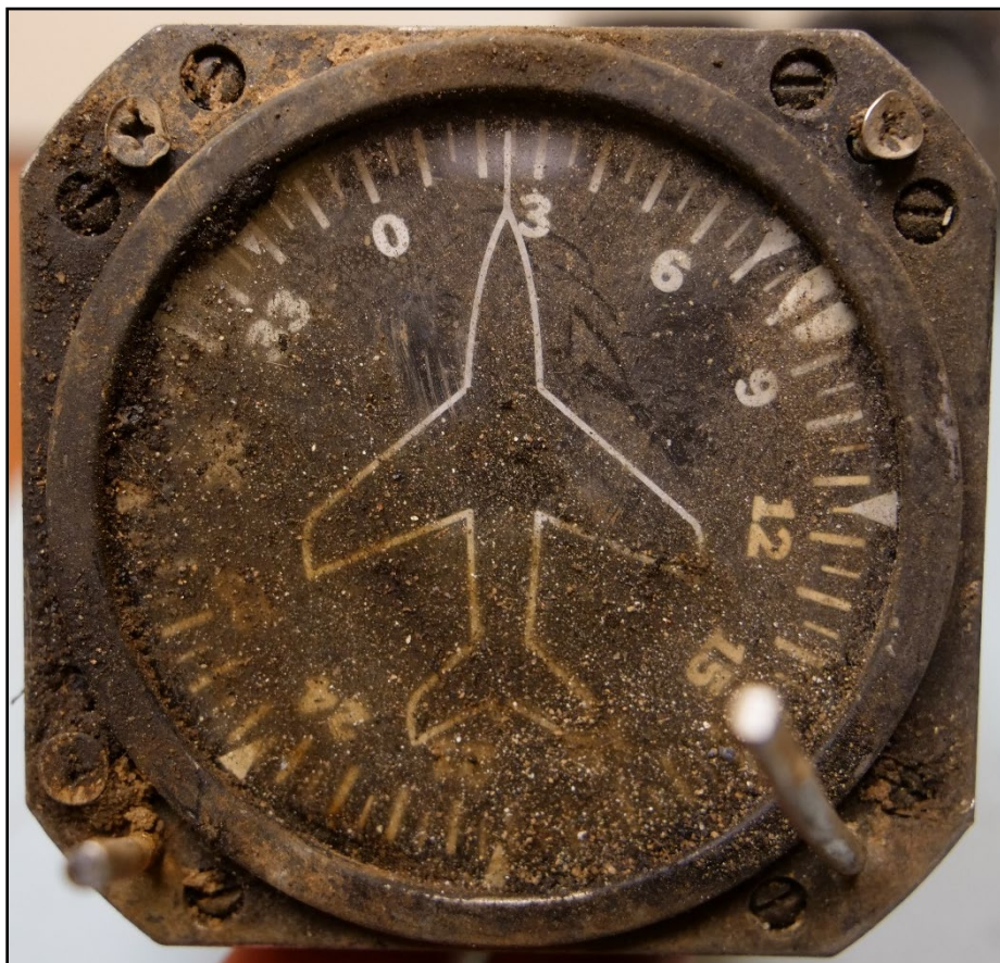
Photograph 1 – Accident airplane - directional gyro.
