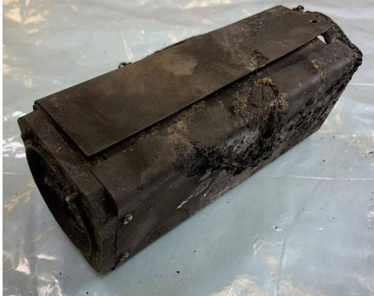
Figure 1. Damaged exterior of EDM.
