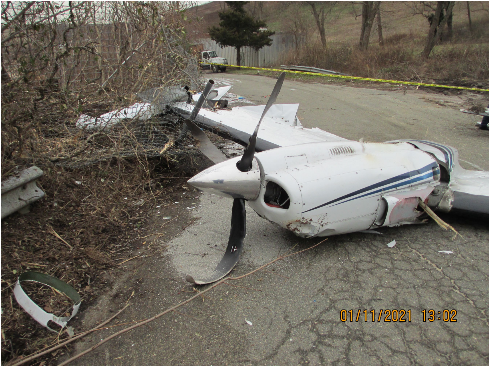
Photo 3 – Right Wing and Engine (FAA Photo)
