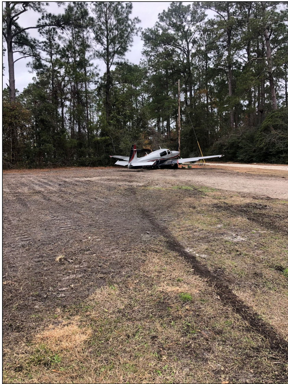
Photo 1 – View of the airplane and ground scarring from the runway excursion (Photo Courtesy of FAA)
