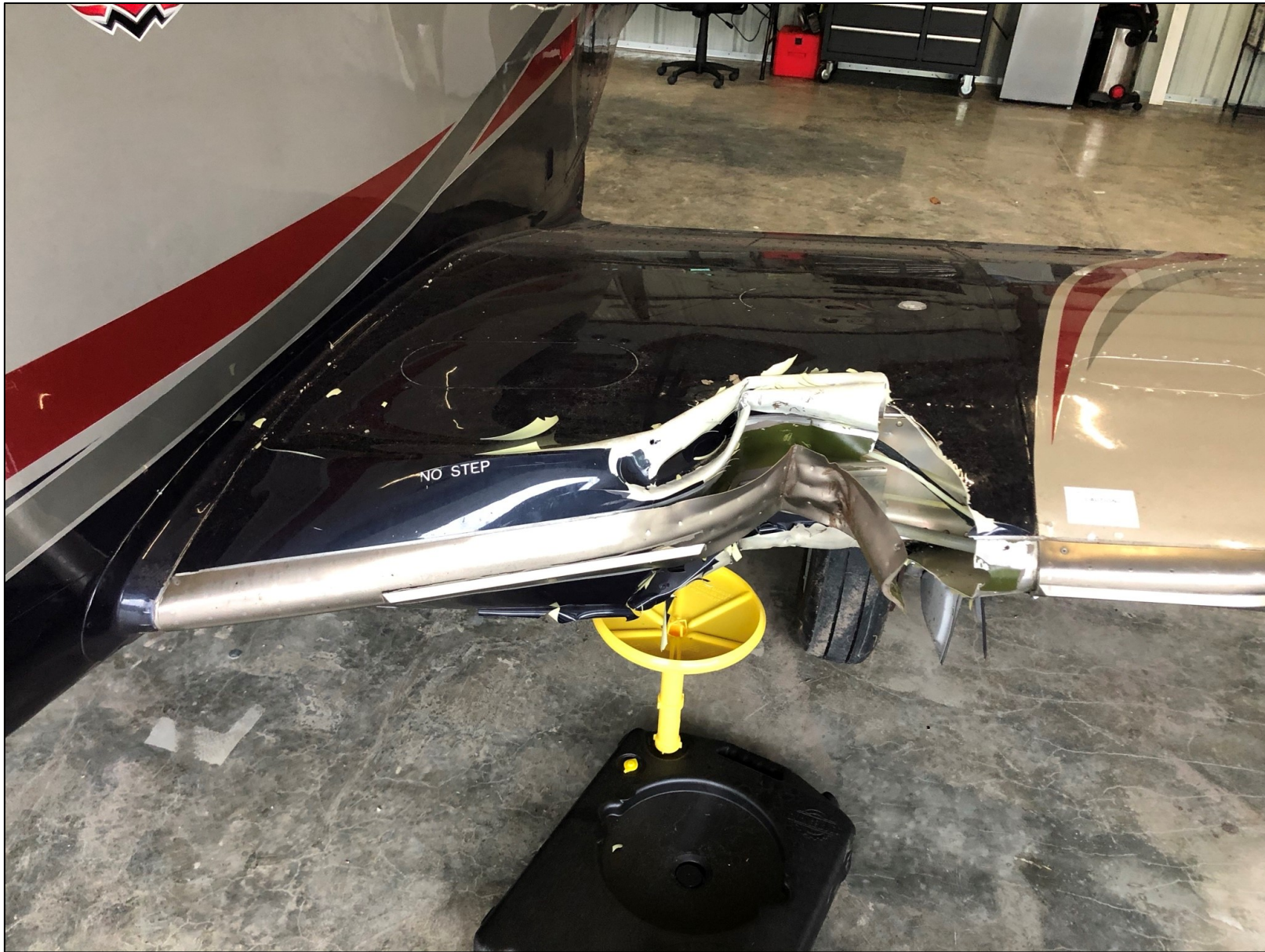
Photo 2 – View of the substantially damaged left wing (Photo Courtesy of FAA)
