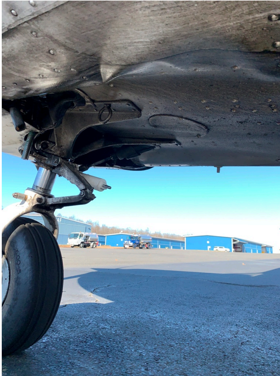
Photo 2 - FAA Digital Photograph. View Taken Aft of Nose Landing Gear Looking Forward and to the Right. Note The Structural damage to Bottom of Fuselage Aft of the Nose Landing Gear.
