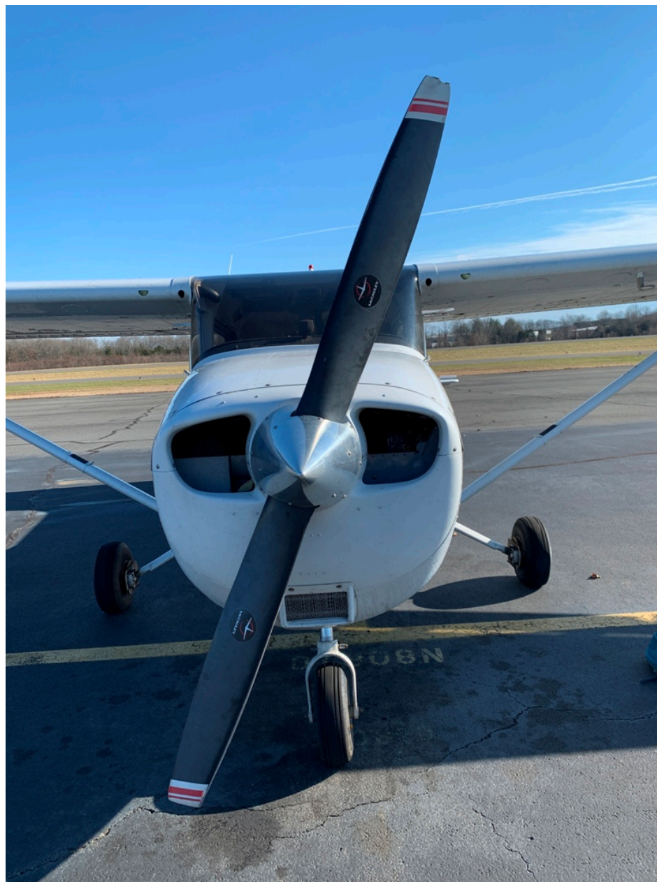
Photo 1 – FAA Digital Photograph. Frontal View of the Airplane Looking Aft. Note the Damage to the tip of Each Propeller Blade.
