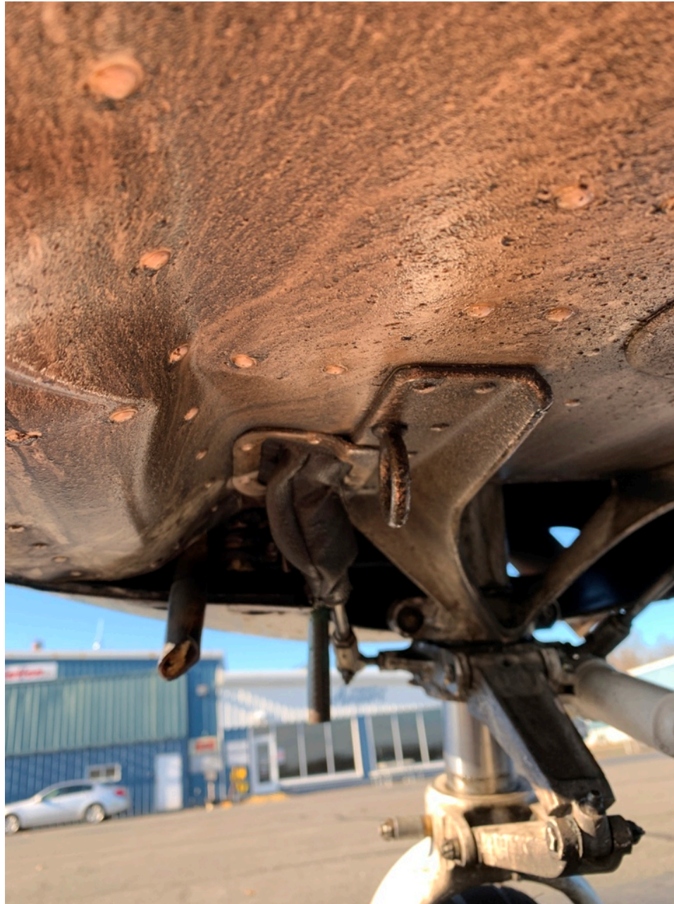
Photo 3 - FAA Digital Photograph. Close-Up View Taken Aft of Nose Landing Gear Looking Forward. Note Structural damage to Bottom of Fuselage Aft of the Nose Landing Gear.
