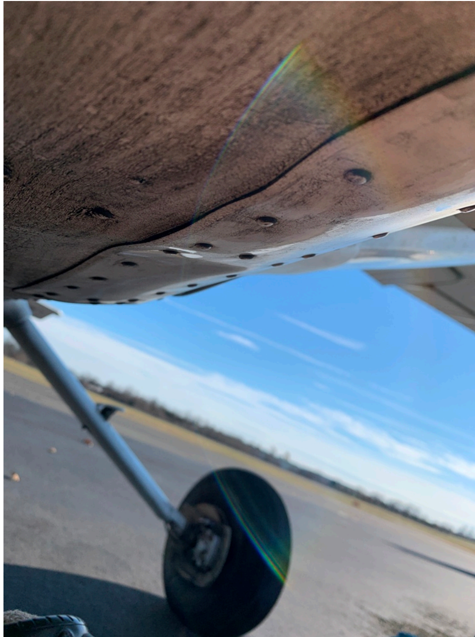
Photo 4 - FAA Digital Photograph. View Taken Aft of Nose Landing Gear Looking Aft. Note the Structural Damage to the Bottom Portion of the Fuselage.
