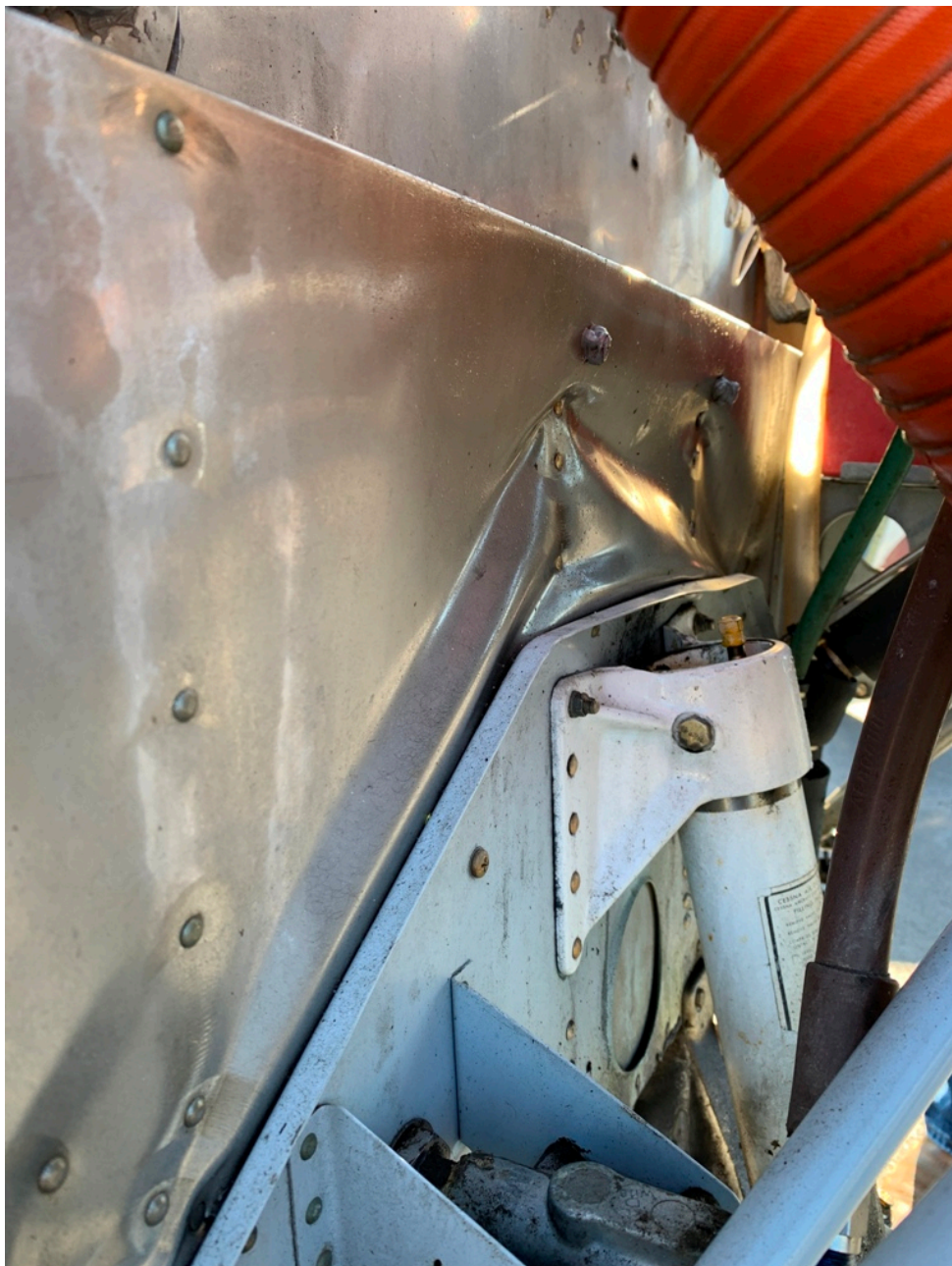
Photo 5 - FAA Digital Photograph. View Depicting Damage to the Firewall.
