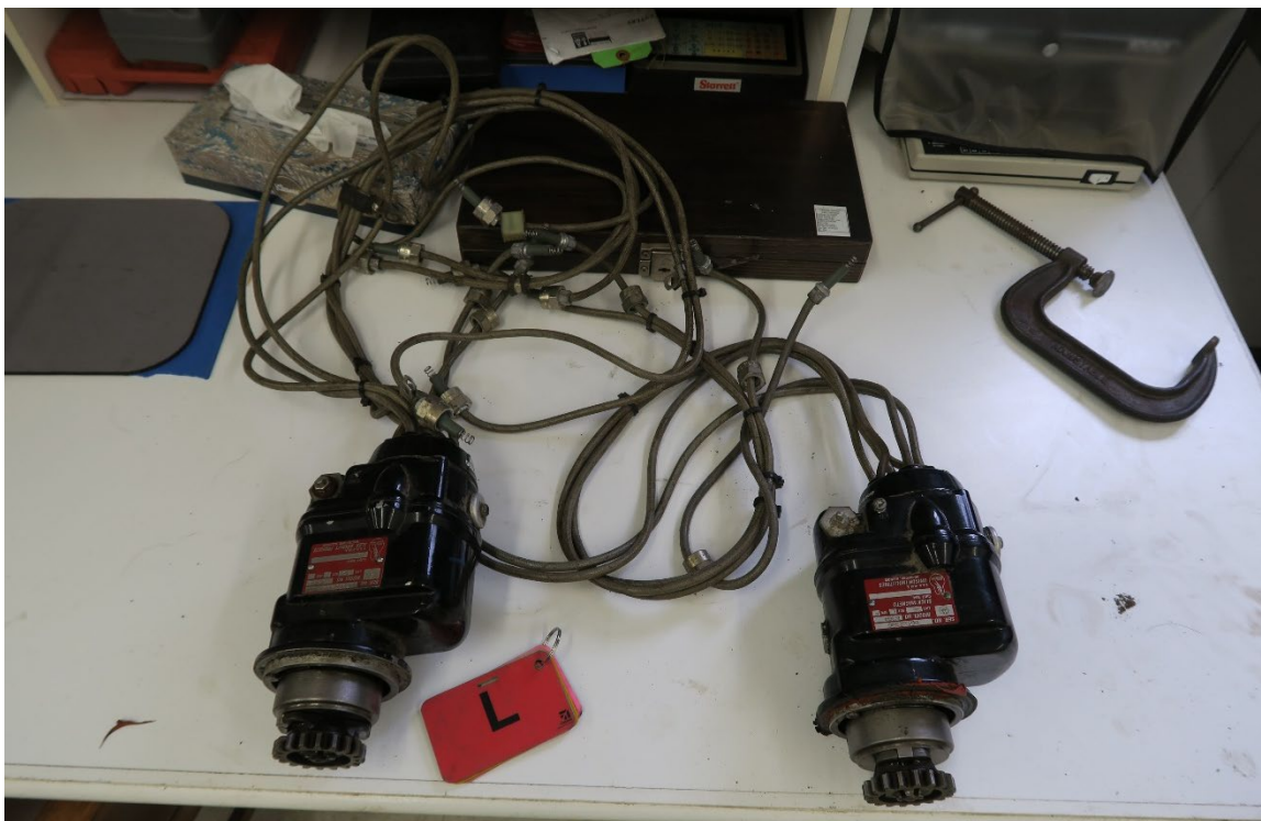
Figure 3: View of the left and right magnetos. (Photo courtesy of Textron)
