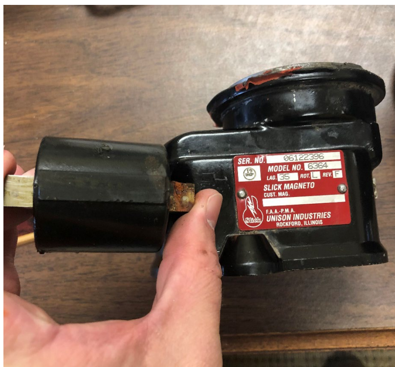
Figure 2: View of the right magneto and coil. (Photo courtesy of Textron)
