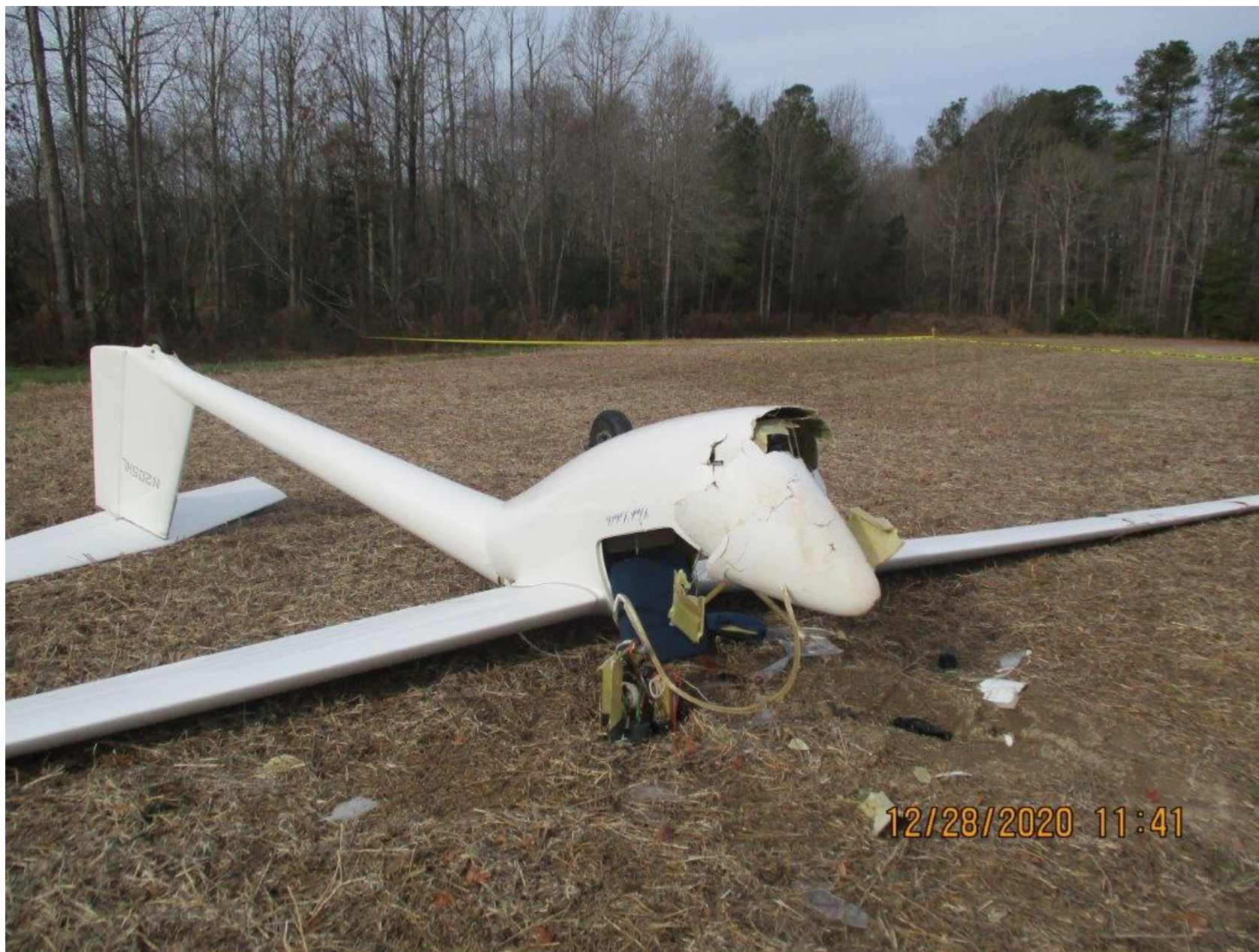
Photo 1 – View of glider structurally damaged in a field (FAA Photo)
