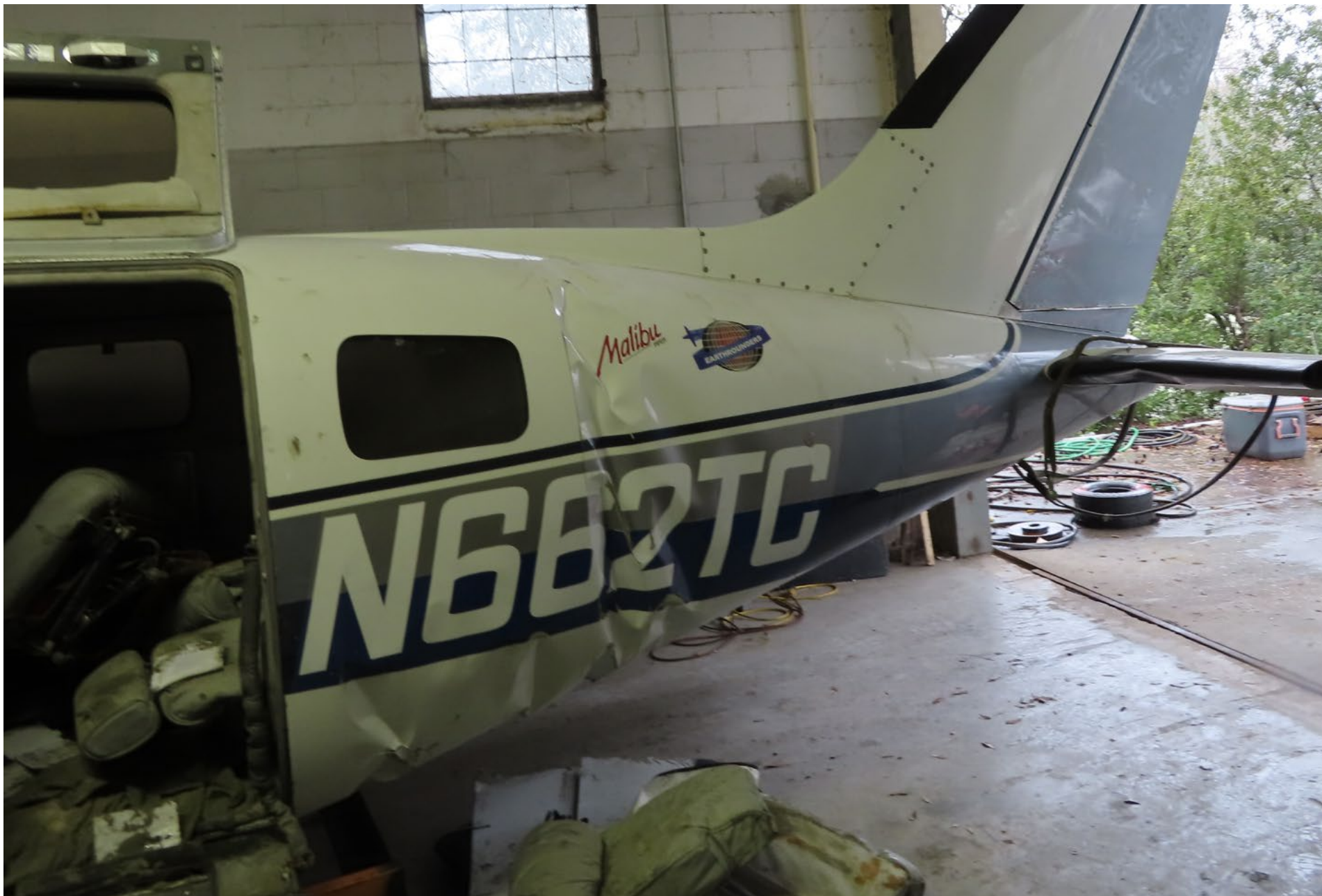
Photo 12 – Close Up of Damage to Aft Fuselage Area – Courtesy of Piper Aircraft
