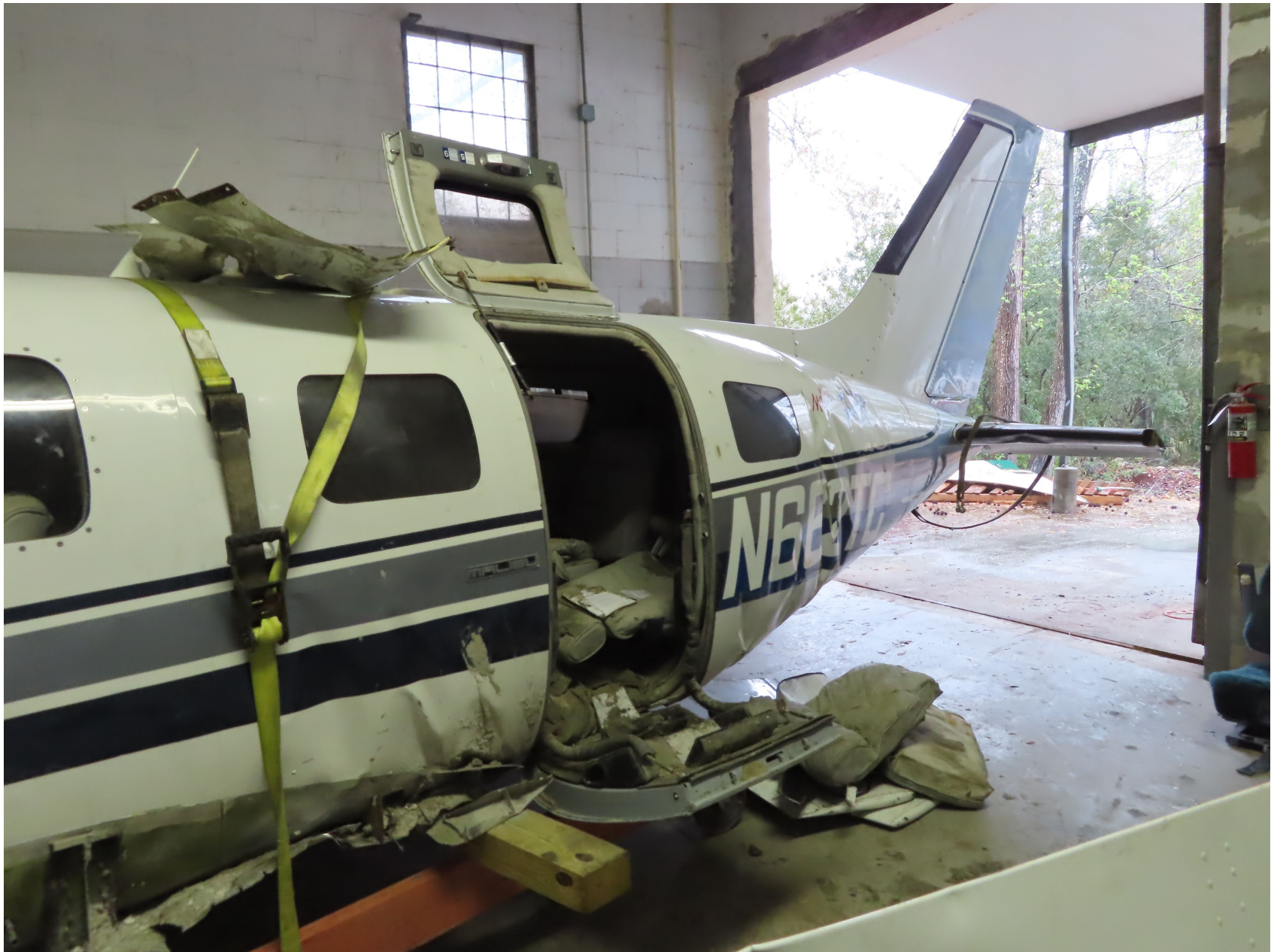
Photo 10 – Damage to Mid and Aft Fuselage Areas – Courtesy of Piper Aircraft
