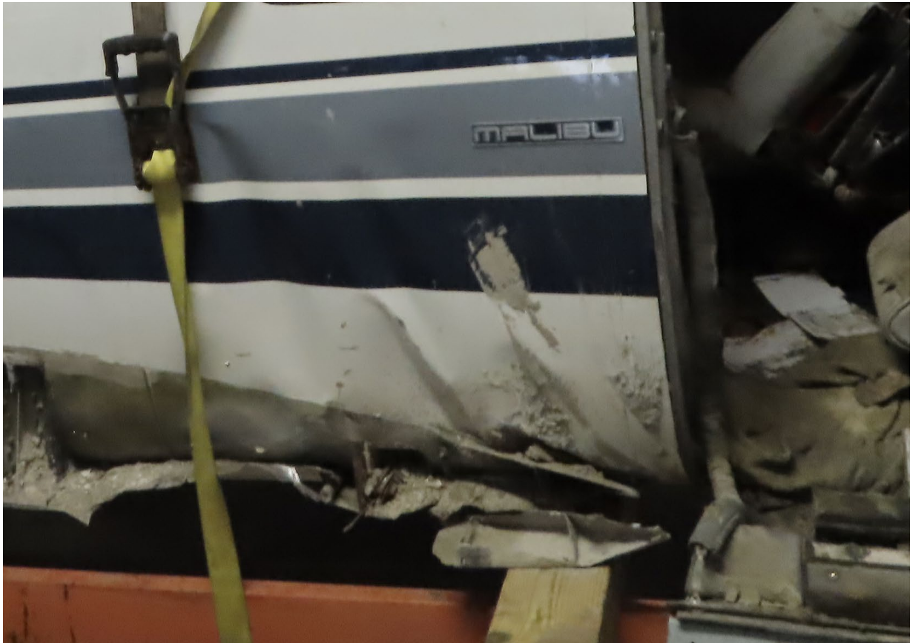
Photo 11 – Close Up of Damage to Mid Fuselage Area – Courtesy of Piper Aircraft
