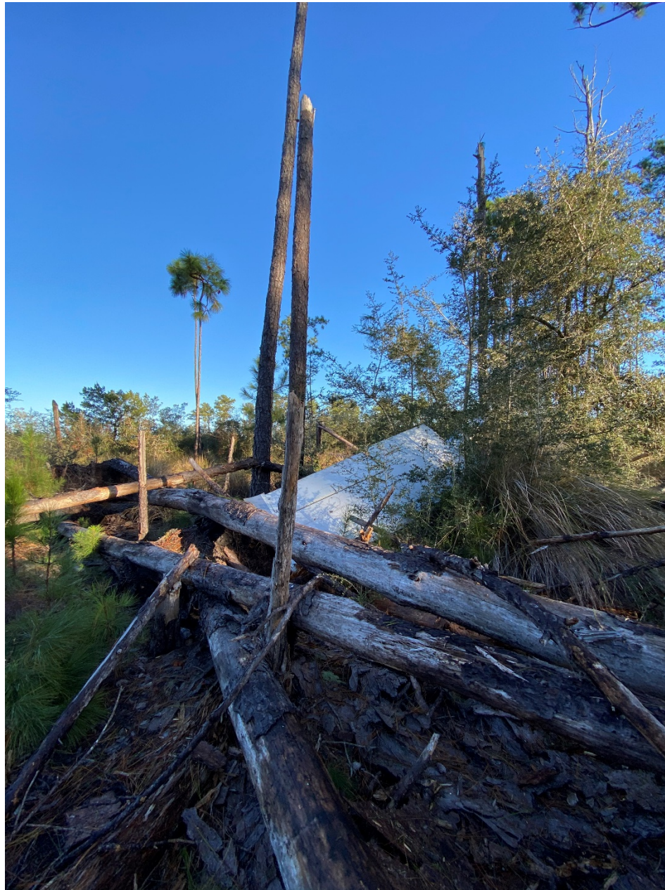
Photo 6 – View of Outer Right Wing Section (Photo Courtesy of Atlanta Air Salvage)
