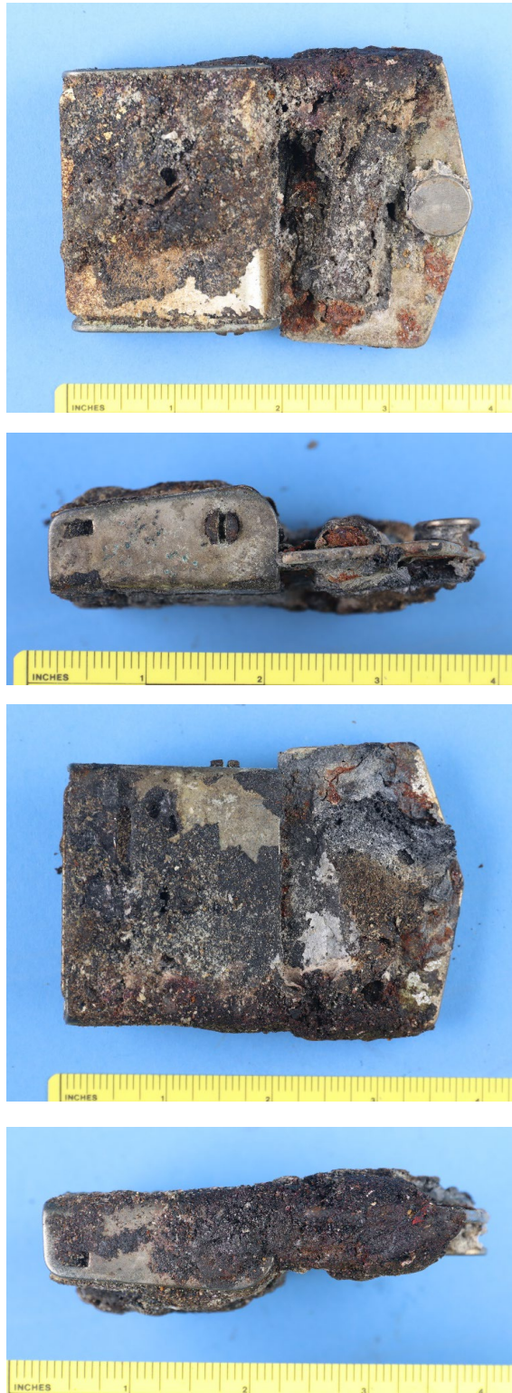
Figure 1: Macro photos of the left rear seat belt buckle with the link connector still engaged. The views are rotated 90 degrees from each other, top to bottom.
