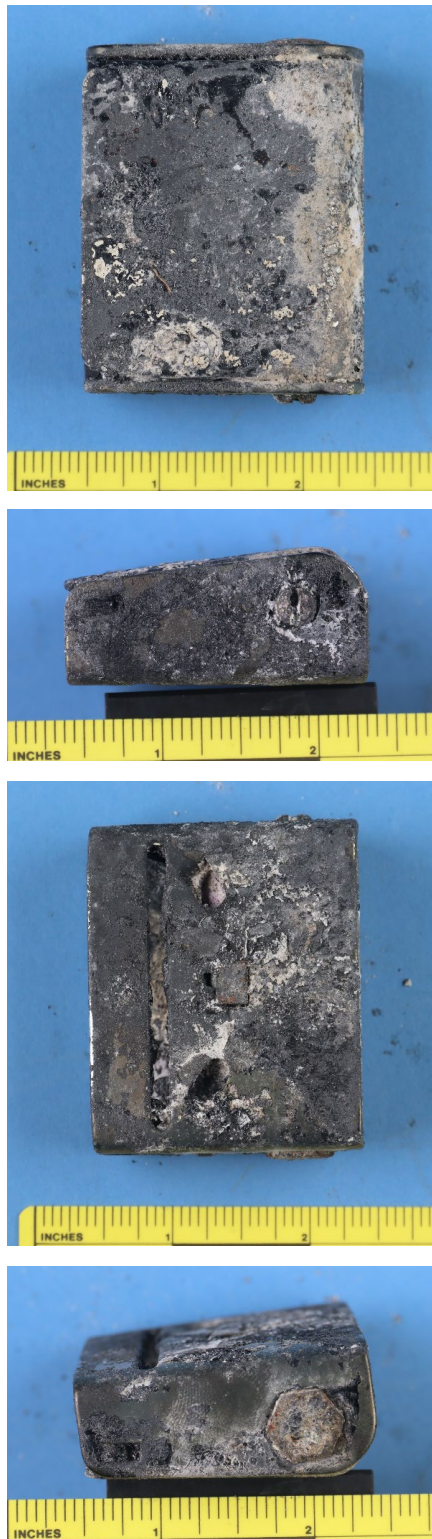
Figure 2: Macro photos of the right rear seat belt buckle that did not have a link connector still engaged. The views are rotated 90 degrees from each other, top to bottom.
