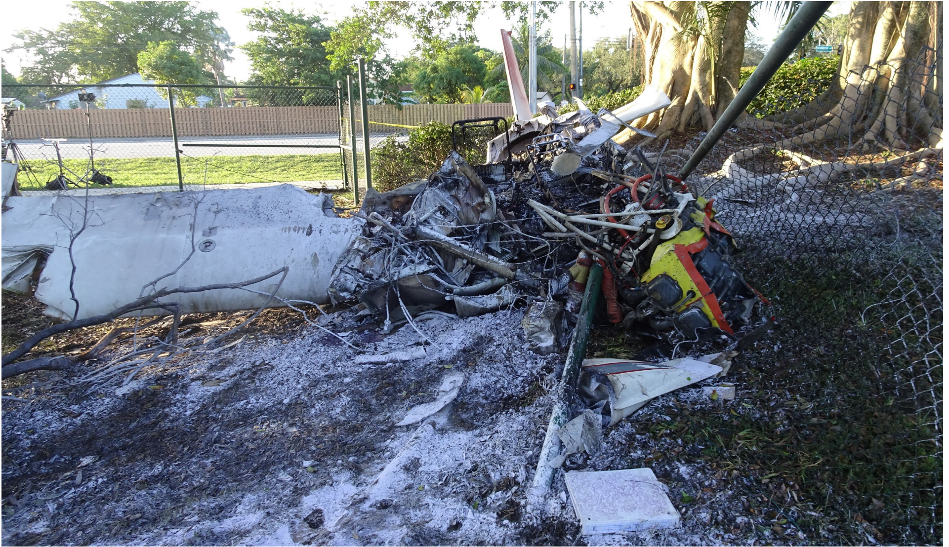
Photo 3 - Digital Photograph From Daher. View Depicting The Right Wing, Separated Engine, and Fuselage. Note the Extensive Postcrash Fire Damage to the Cockpit and Cabin.
