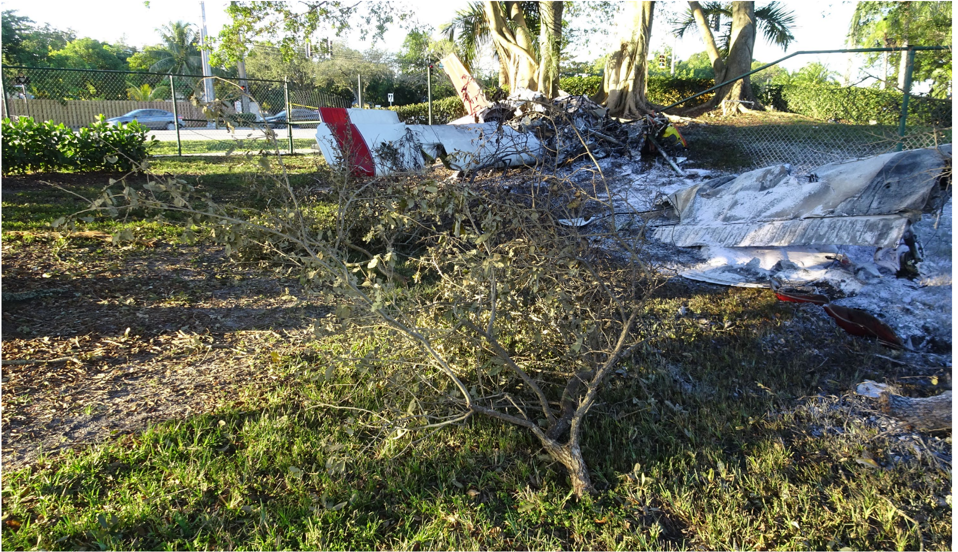
Photo 2 - Digital Photograph From Daher. View Depicting the Separated Portion of the Left Wing in the Foreground, Right Wing and Main Wreckage in the Background.
