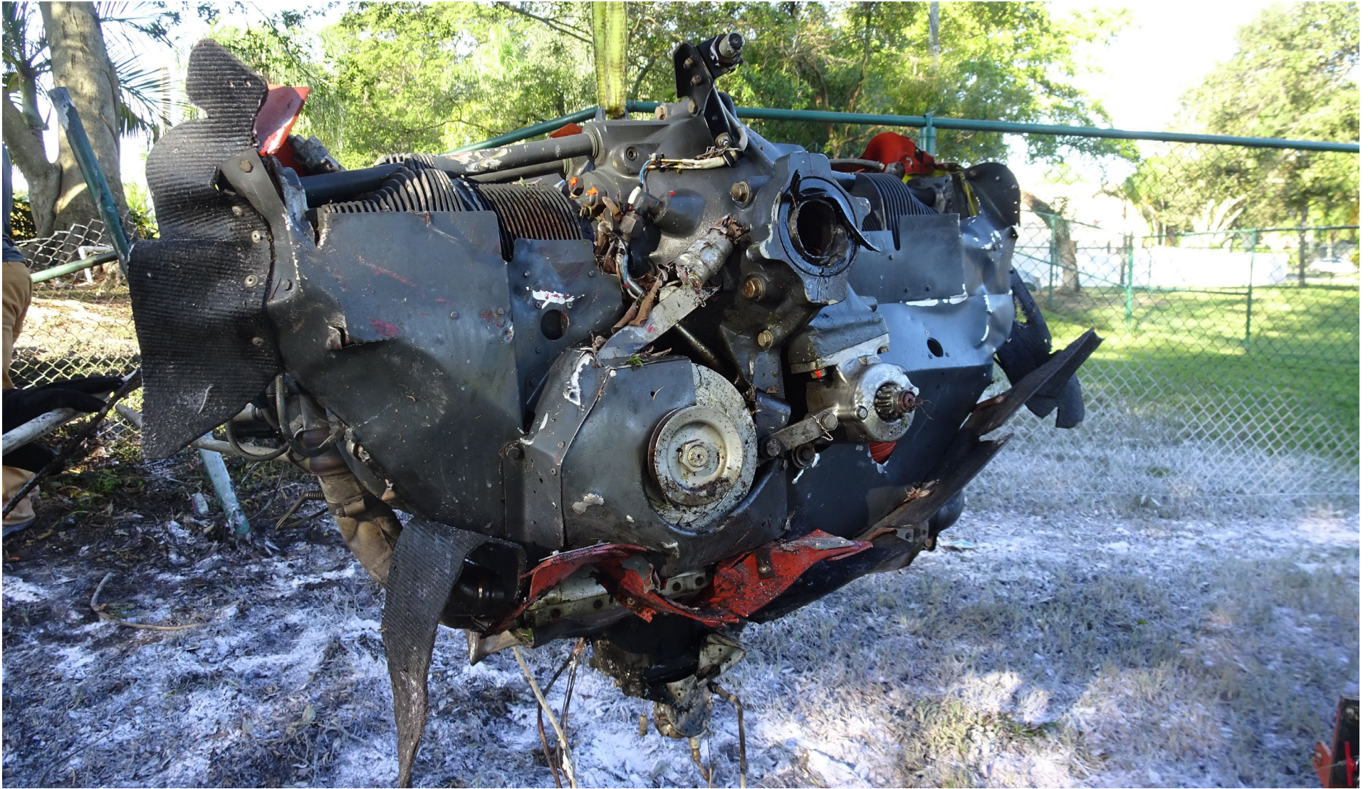
Photo 7 - Digital Photograph From Daher. View Depicting The Separated Engine Assembly. Note the Fractured Crankshaft.
