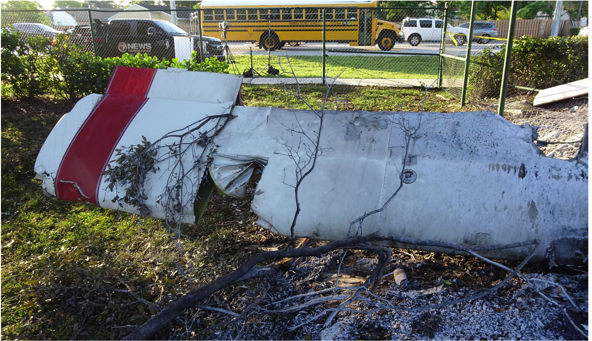
Photo 4 - Digital Photograph From Daher. View Depicting The Majority of the Right Wing. Note the Impact Damage to the Outer Leading Edge and the fire damage to the Inboard Section of the Wing.
