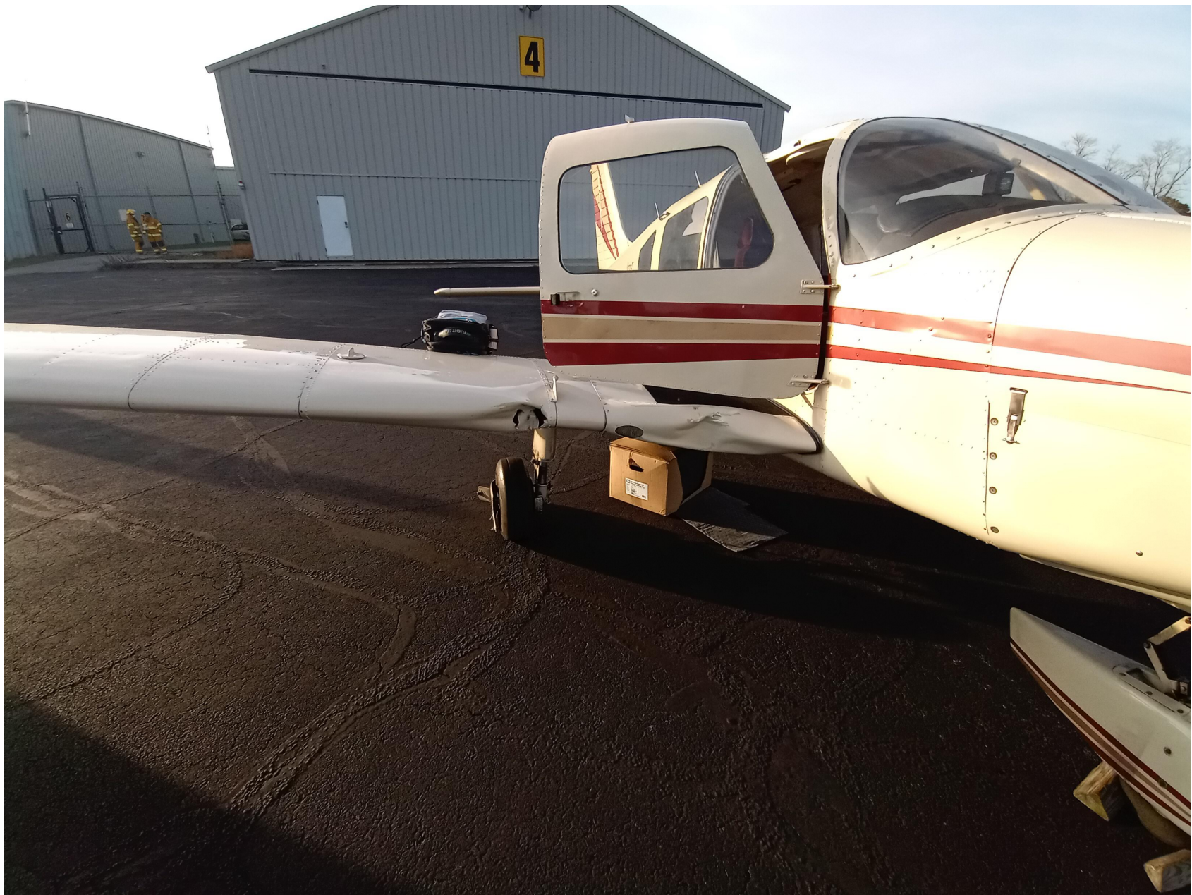
Photo 1 – View of the damage to the right wing leading edge and wing root. (Photo courtesy of the FAA)
