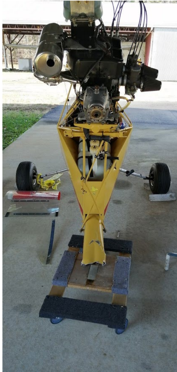
Photo 3 – Aft view of airplane looking forward. View of damaged tail boom. (Courtesy of Owner/Operator)
