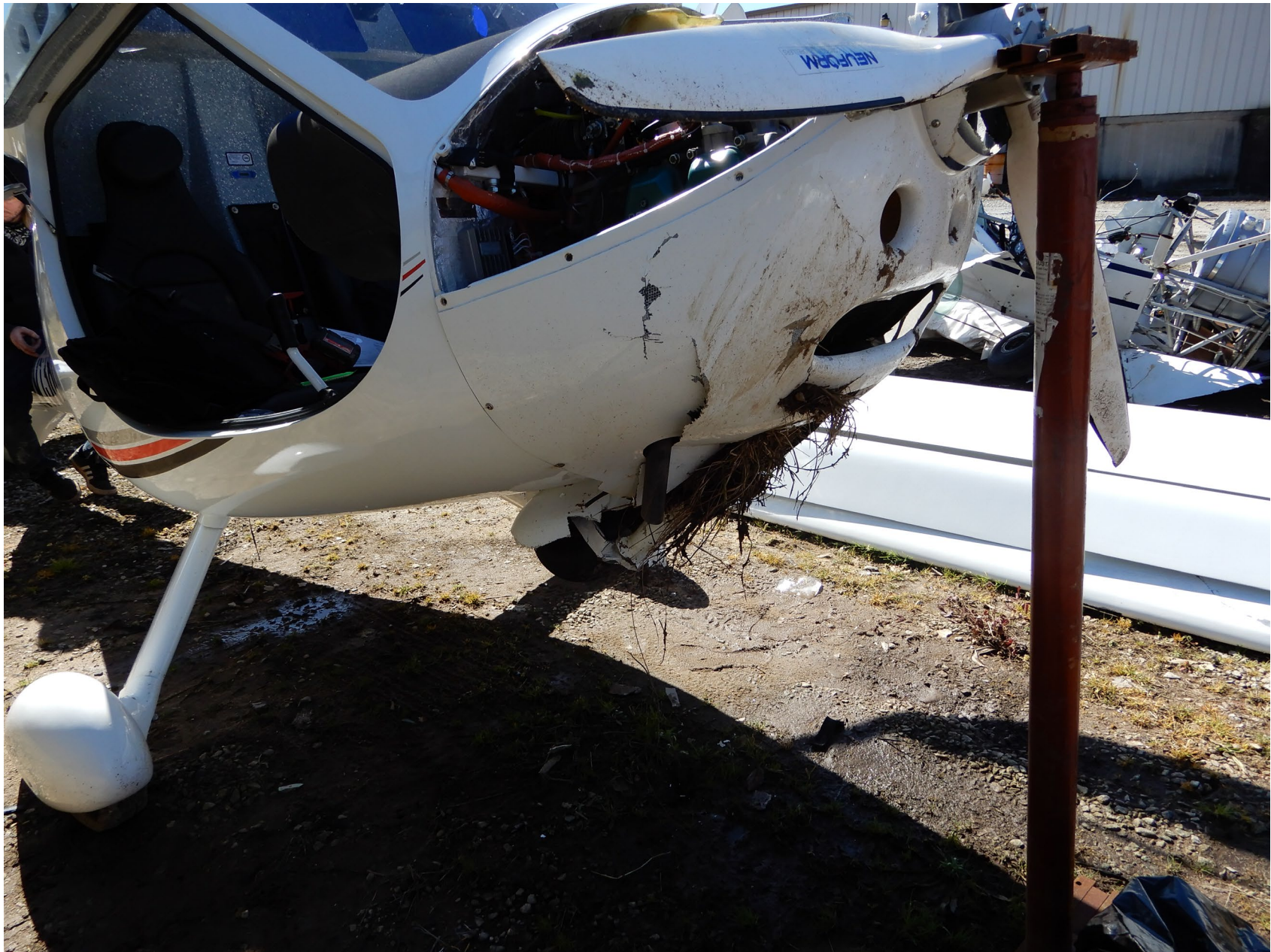
Photo 5 – Nose Gear Damage (NTSB Photo)
