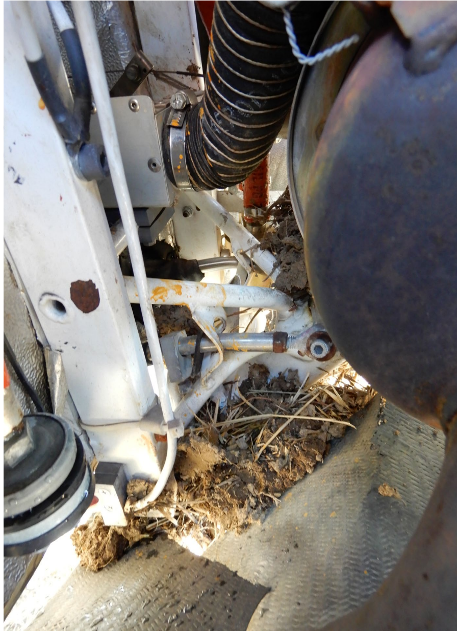
Photo 7 – Bent Rod Between Rudder Pedals and Nose Landing Gear (NTSB Photo)
