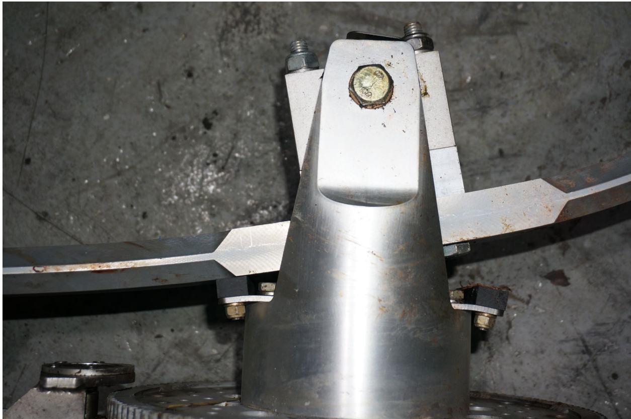
Figure 2. View of the droop stops for the main rotor blades.
