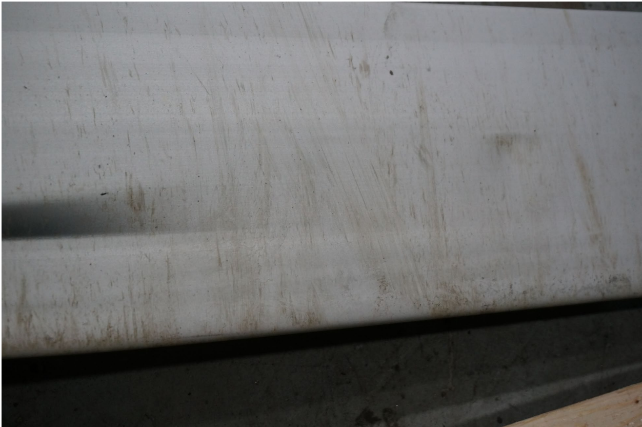
Figure 3. View of chordwise scratching on main rotor blade.
